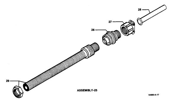
Figure 4. Magnetic Pickup Assembly
