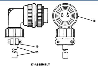
Figure 2. 90° Connector Assembly
