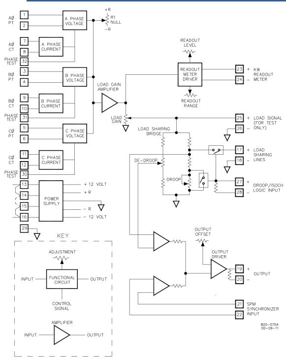
Figure 2-1. Real Power Sensor Block Diagram (8272-781 and 8272-826)
