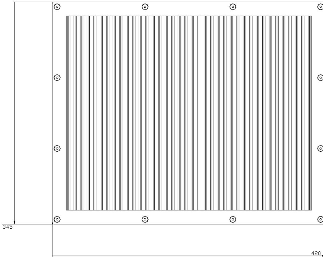
Heat Sink : Extruded anodized aluminium
