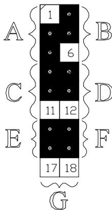
If the controlling signal of the transmitter should be DTR instead of RTS, move the 3-pin jumper, B, to the opposite position (4 + 6).
