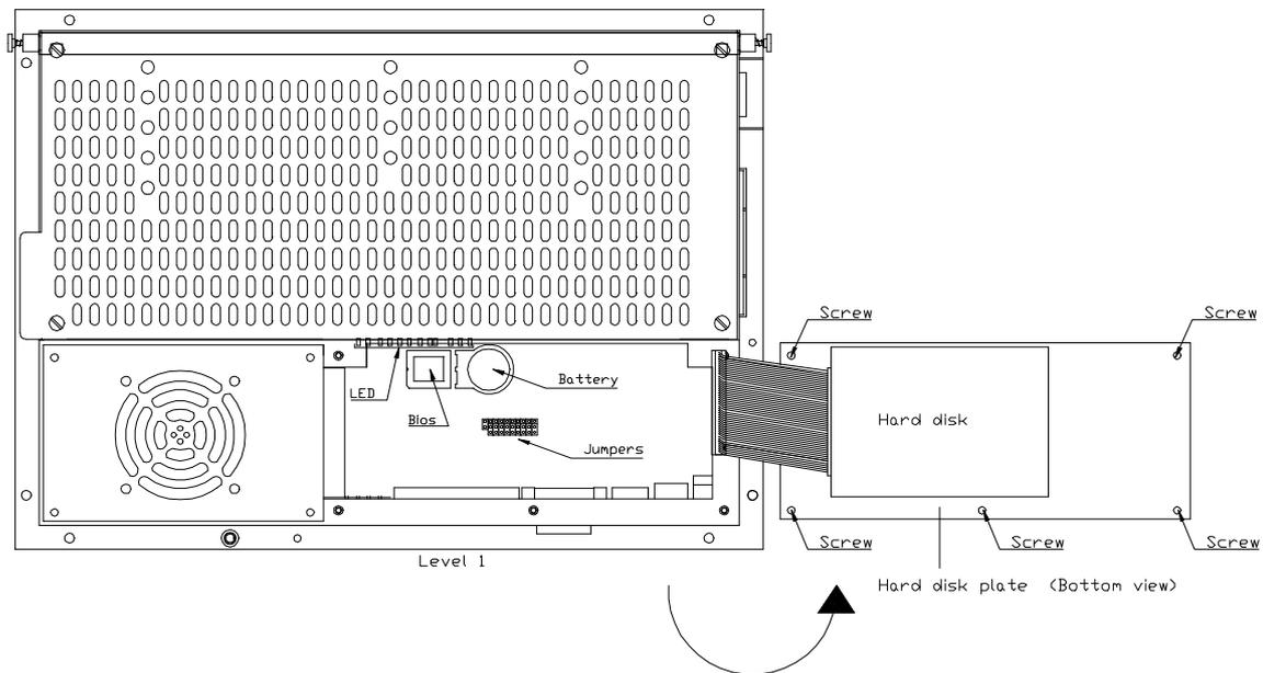
**Battery** : - Remove the 5 screws (4) and turn the sheet 90 degrees to the right
