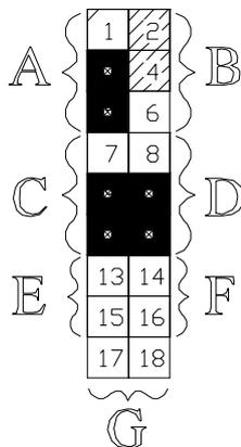
If an 120W termination between RxD and RxD- is required, then short jumper G (17 + 18) as well. Please note, that jumper G is 90° rotated.
