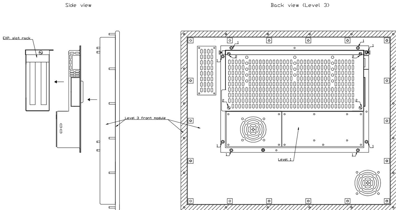
Remove the 8 nuts (marked 1) and then pull the Level 1 away from the front module.
