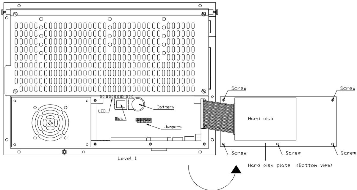
By rewinding 5 screws, the service zone of the Level 1 unit can be accessed. It is not necessary to remove the cable from the hard disk.
