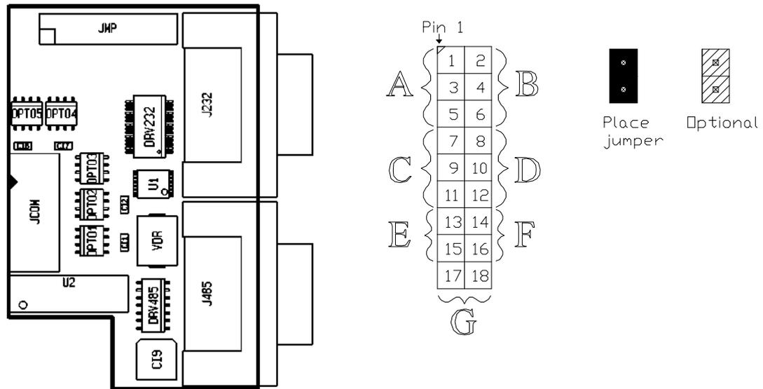
The location of the connectors depends on the PCI6000 model. Each serial port module provides two Dsub-9 connectors: One male and one female. They are not electrically mutual exclusive, as they are only intended to be used one at a time. Please note that the module must be factory mounted.
