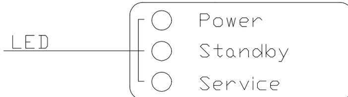
To inspect the system parameters start the ISC hardware monitor program and check parameters. This program may also turn the LED off if the violation is removed. System reset will also reset the LED.
