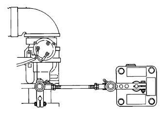
Figure 2-5. Carburetor Compensating Linkage at Minimum Fuel
