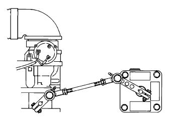
Figure 2-6. Carburetor Compensating Linkage at Maximum Fuel
