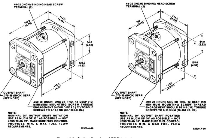
Figure 2-3. Outline Drawing of EPG Actuators (EPG Models 1712/1724 left, Models 512/524 right) (Do not use for construction.)
