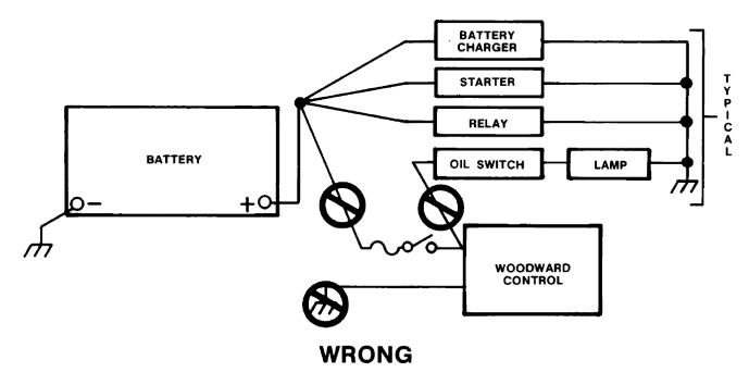
Figure 2-10. Correct and Incorrect Wiring to Battery
