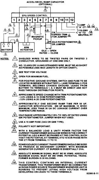
Figure 2-7. Typical EPG (with droop) Wiring Diagram
