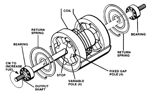
Figure 4-2. Actuator Schematic
