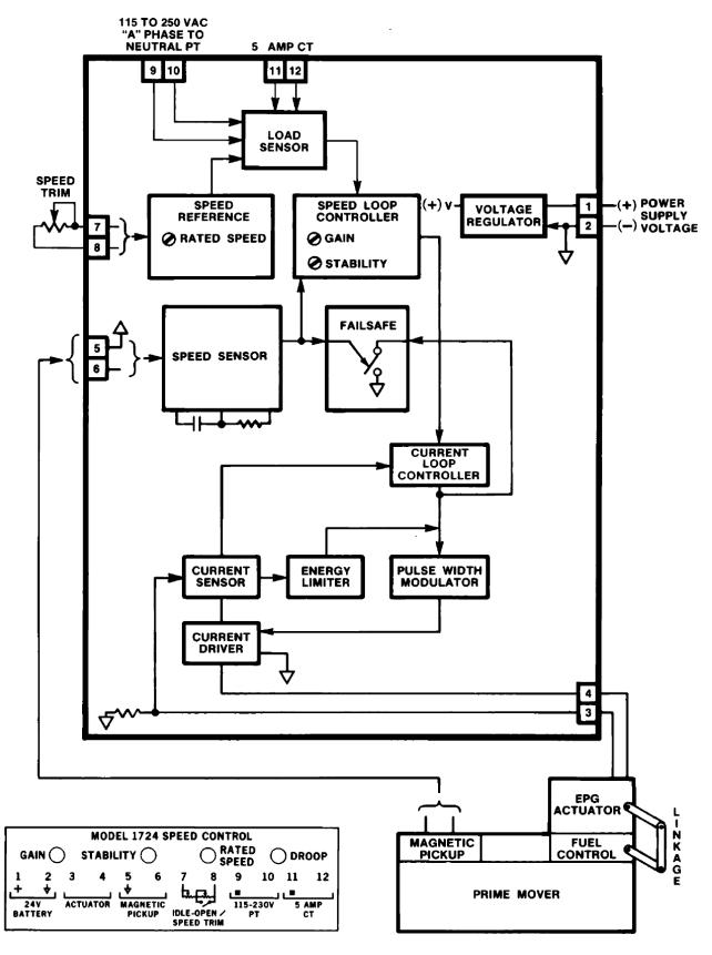
Figure 4-1a. EPG Block Schematic Diagram (standard)
