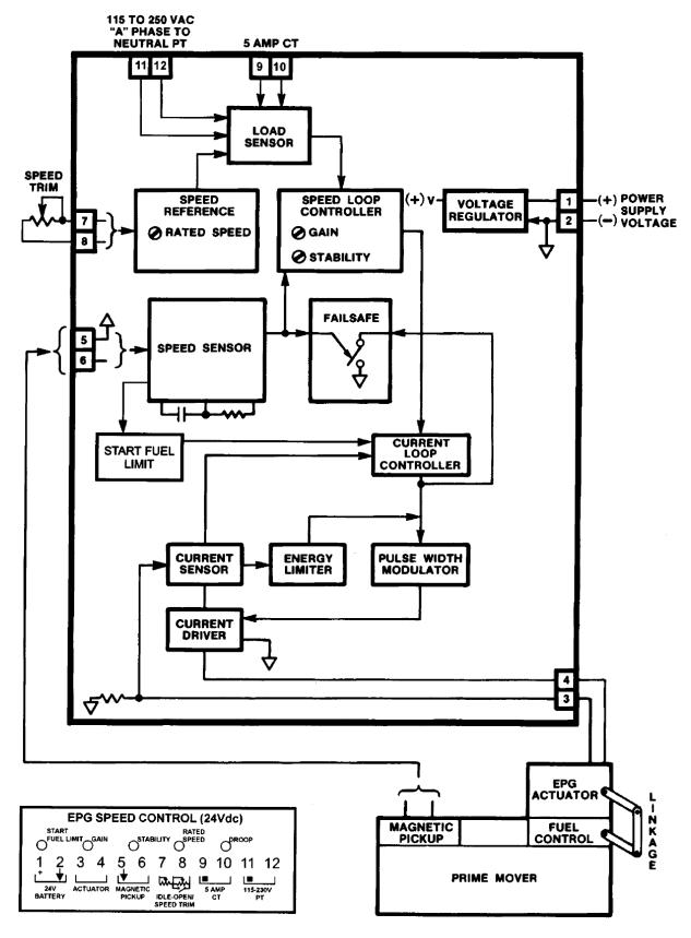
Figure 4-1b. EPG Block Schematic Diagram (start fuel limit)
