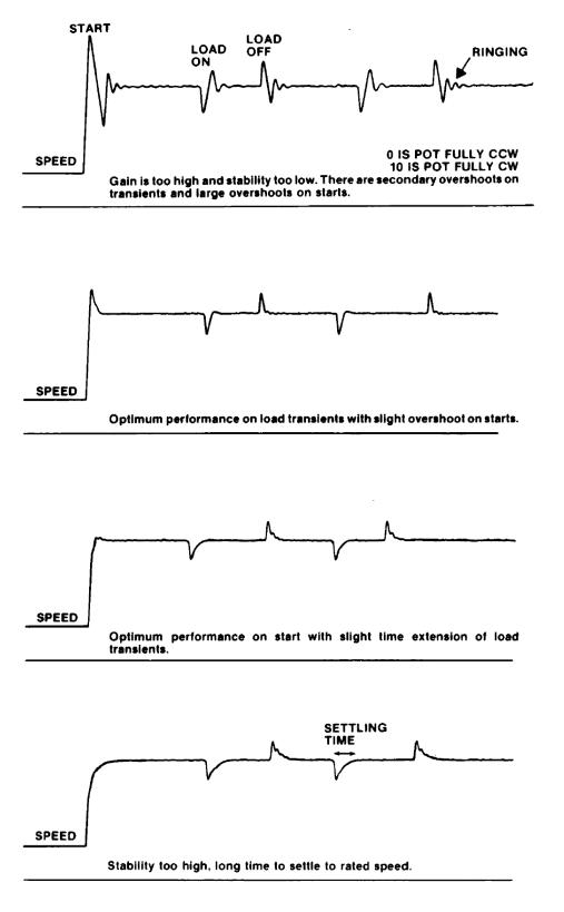
Figure 2-11. Starting and Transient Response Curves
