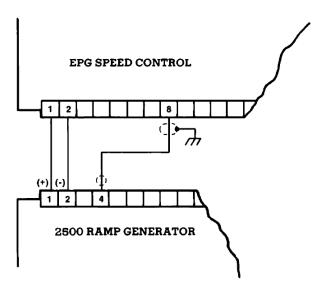
Figure 2-8. Typical Wiring for 2500 Ramp Generator
