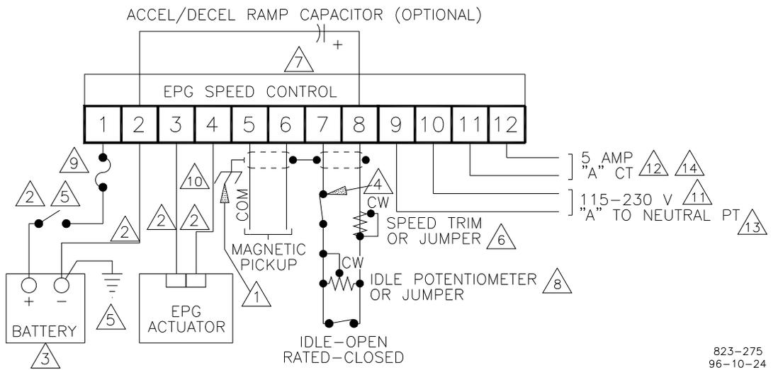
Figure 1-3. Wiring Diagram (EPG with Droop)
