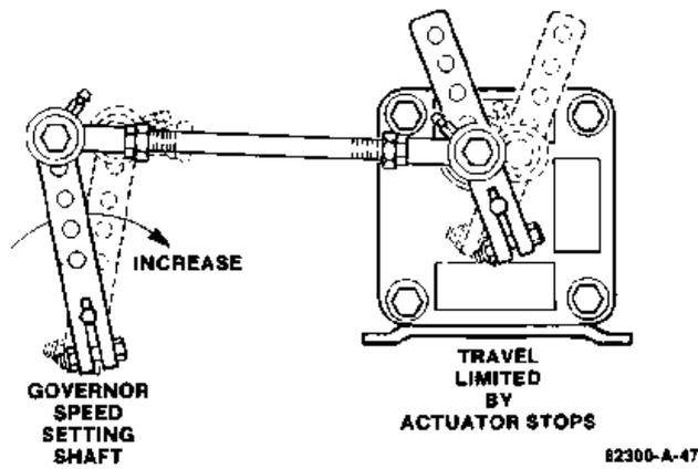
Figure 2-1. Actuator Linkages
