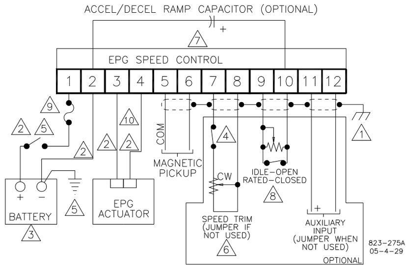
Figure 1-2. Wiring Diagram (Isochronous EPG)
