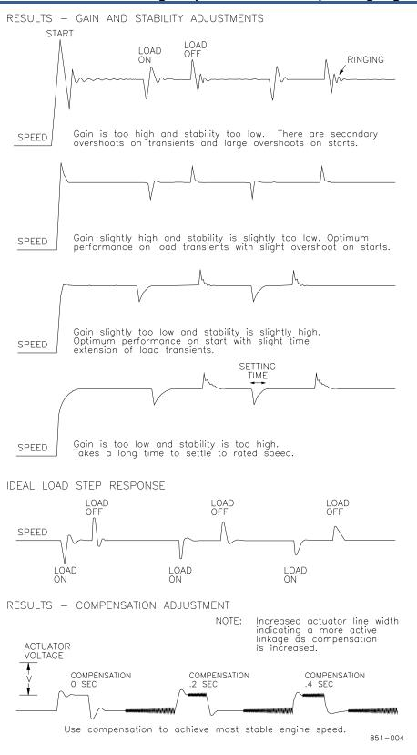
Figure 3-4. Typical Transient Response Curves
