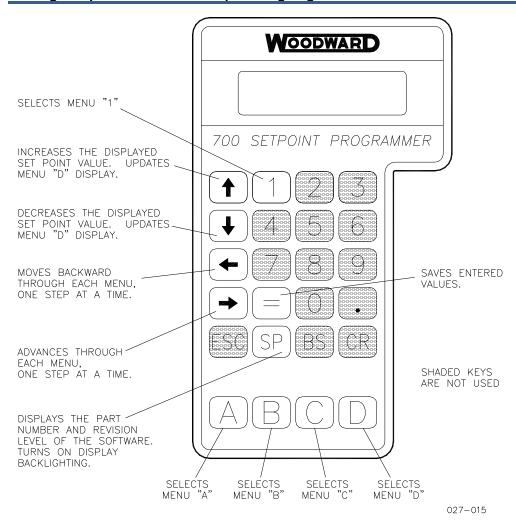
Figure 3-1. Set Point Programmer Functions
