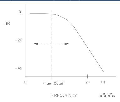
Figure 3-5. Speed Filter
