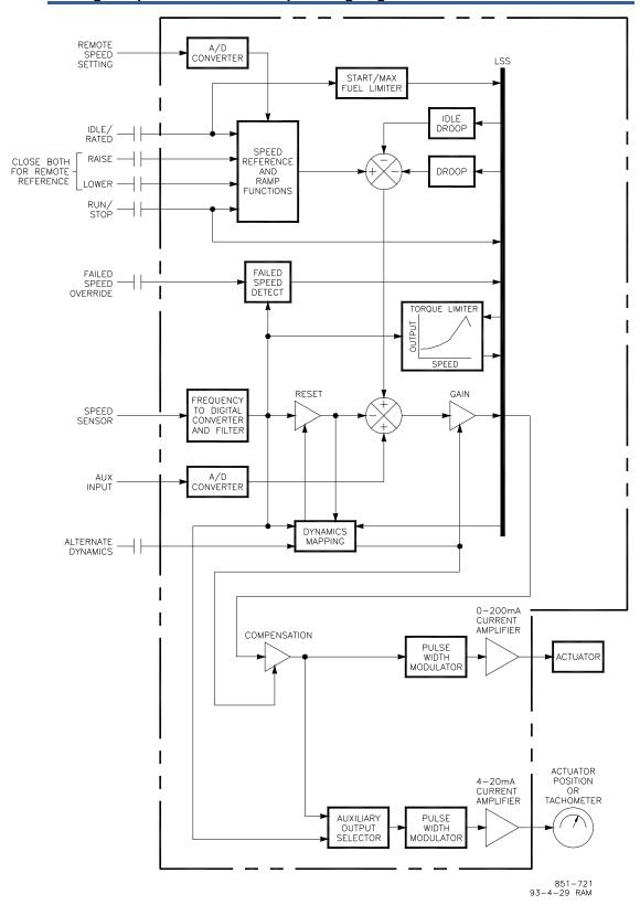
Figure 1-4b. Block Diagram (9905-457)
