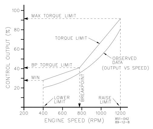
Figure 3-6a. Torque Limit Setup Example (standard models)
