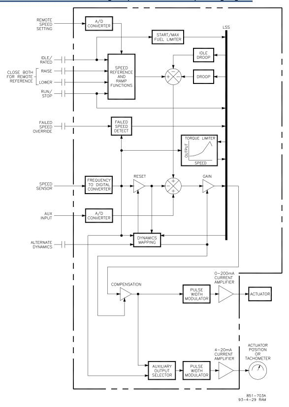
Figure 1-4a. Block Diagram (standard models)
