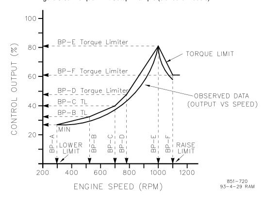
Figure 3-6b. Six-Breakpoint Torque Limiter (9905-457)
