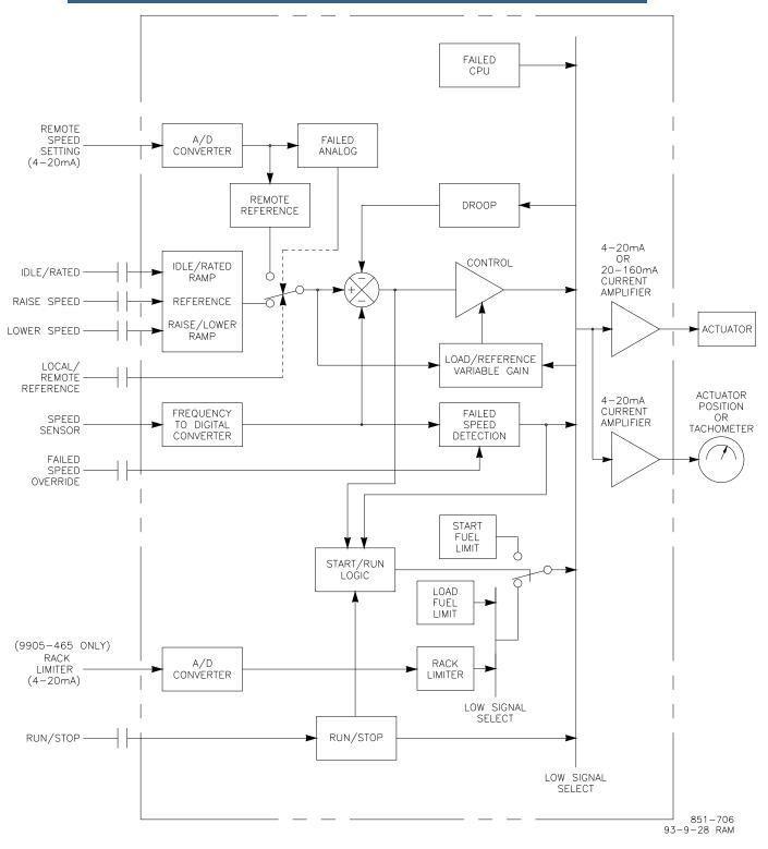
Figure 1-7. Block Diagram
