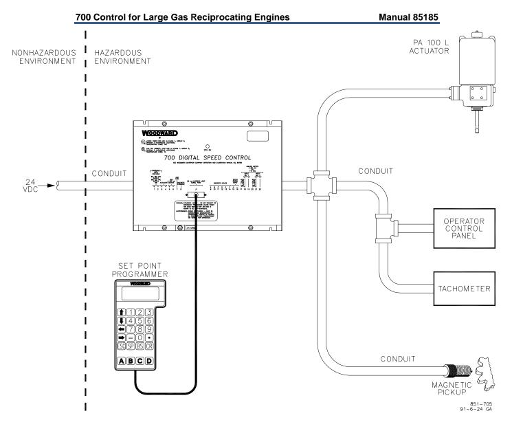
Figure 1-4. Typical Class I, Division 2, Group D Installation
