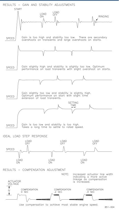
Figure 3-4. Typical Transient Response Curves
