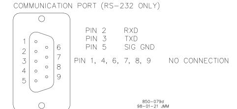
Figure 4-16. CPU Communications Port
