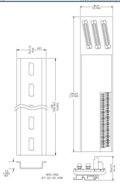
Figure 3-7. DIN Rail & ATM Outline Drawing
