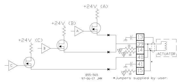
Figure 4-6. Example Single Coil Actuator Wiring Diagram
