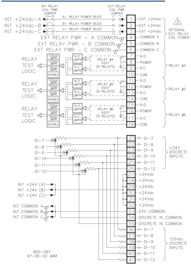
Figure 4-24. DTM–2 Wiring Diagram
