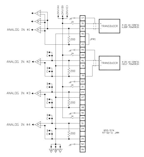
Figure 4-4. Example Analog Input Wiring Diagrams
