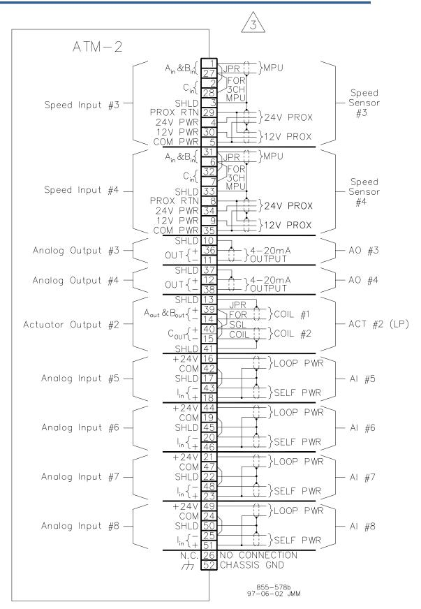
Figure 4-22. ATM-2 Wiring Diagram
