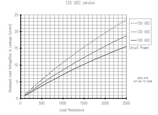
Figure 4-12. Latent Fault Detection Verification Graph—100–150 Vdc Circuitry
