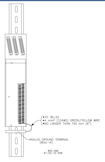
Figure 3-8. ATM Grounding Diagram
