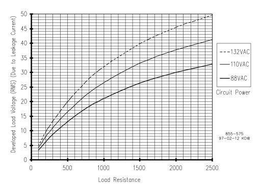
Figure 4-11. Latent Fault Detection Verification Graph—88–132 Vac Circuitry
