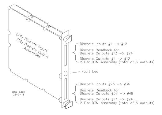
Figure 2-7. Discrete Input/Output Module
