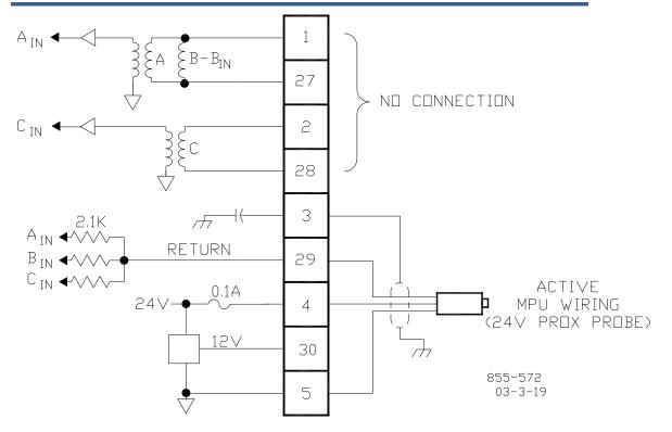
Figure 4-3a. Example 24 V Proximity Probe Wiring Diagram
