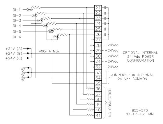
Figure 4-8. Optional Internal 24Vdc Contact Wetting Configuration
