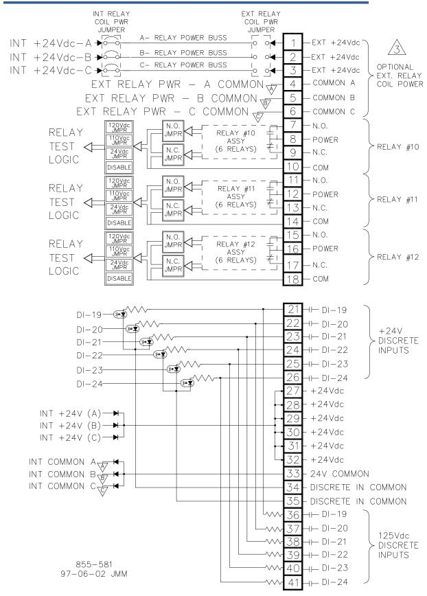
Figure 4-26. DTM-4 Wiring Diagram
