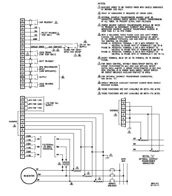
Figure 8-7. Plant Wiring Diagram for the Real Power Sensor
