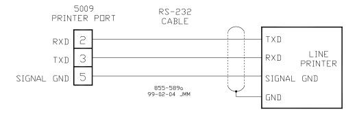
Figure 4-29. Optional Alarm Printer Diagram
