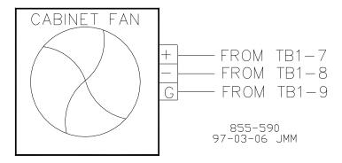
Figure 4-30. Cabinet Fan Diagram
