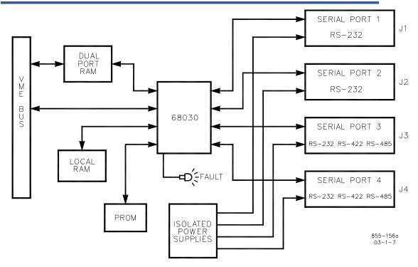
Figure 2-9. SIO Module Block Diagram
