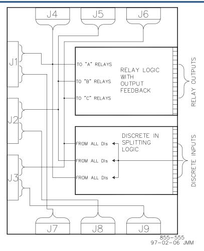
Figure 2-8. DTM Block Diagram
