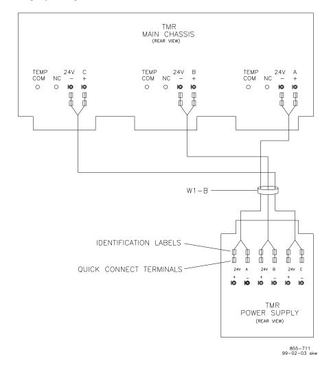
Figure 3-3. Chassis-to-Chassis Power Cable W1-B
