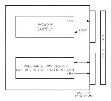
Figure 2-2. Kernel Power Supply Block Diagram
