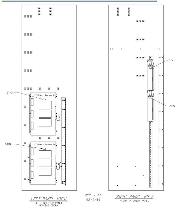
Figure 4-18b. Cabinet—Device Location Diagram
