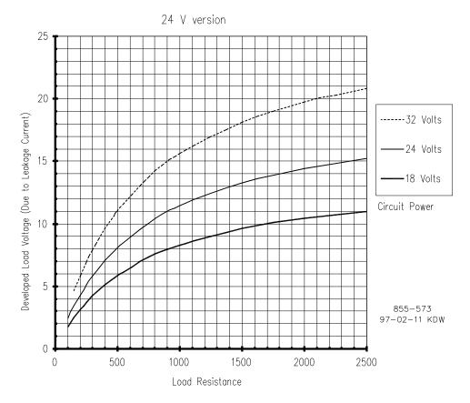
Figure 4-10. Latent Fault Detection Verification Graph—18–32 Vdc Circuitry
