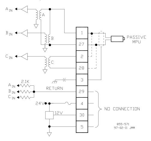
Figure 4-2. Example MPU Interface Wiring Diagram
