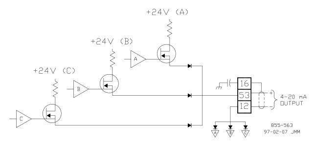
Figure 4-5. Example Analog Output Wiring Diagram
