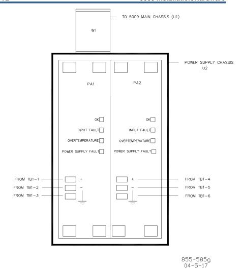
CABINET CONNECTIONS TB1 CUSTOMER CONNECTIONS TB-1TO PA1 (+) LINE NEUTRAL TO PA1 (-)-TO PA1 (GND)-CONTROL INPUT POWER - GROUND - LINE TO PA.2 (+) 16 - NEUTRAL - GROUND CONTROL INPUT POWER TO PA2 (-) TO PA2 (GND) LINE TO CAB FAN (+)
