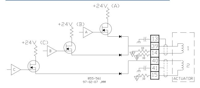
Figure 4-7. Example Dual Coil Actuator Wiring Diagram
