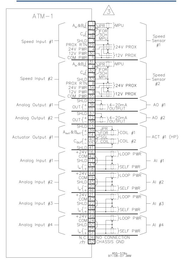
Figure 4-21. ATM-1 Wiring Diagram
