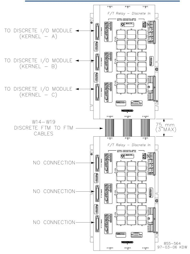
Figure 3-10. DTM Mounting Configuration
