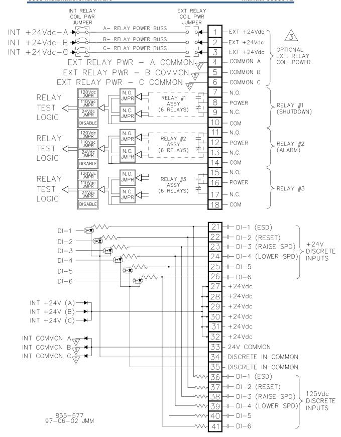
Figure 4-23. DTM-1 Wiring Diagram
