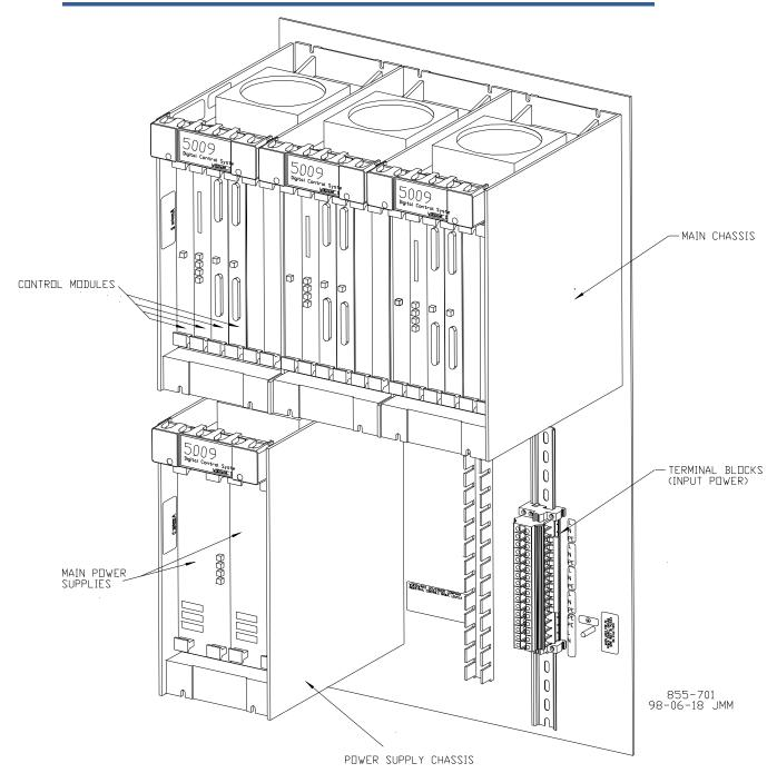
Figure 2-1. Control and Power Chassis
