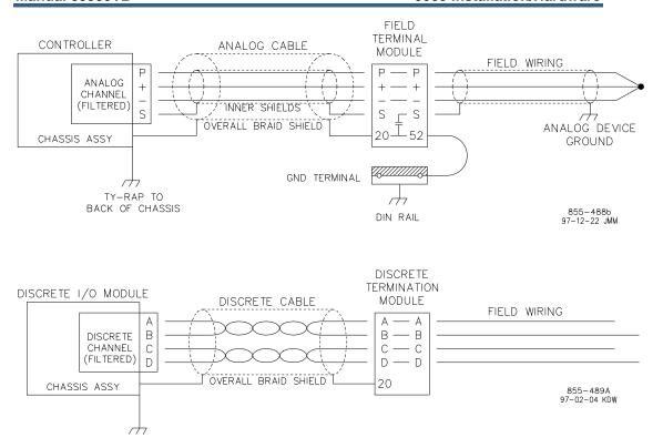
Figure 4-1. Shield Termination Diagram
