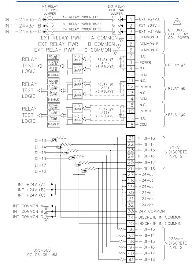
Figure 4-25. DTM-3 Wiring Diagram
