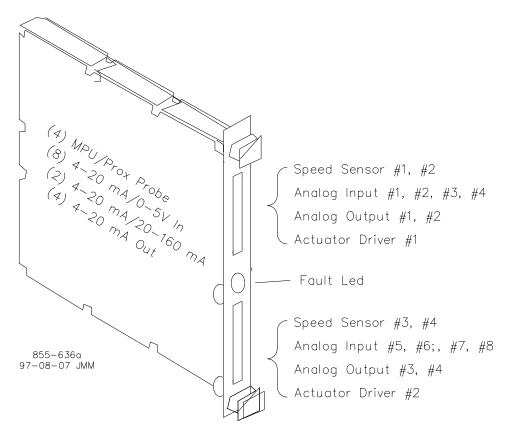
Figure 2-5. MPU and Analog I/O Module
