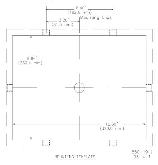
Figure 3-12. Mounting Template
