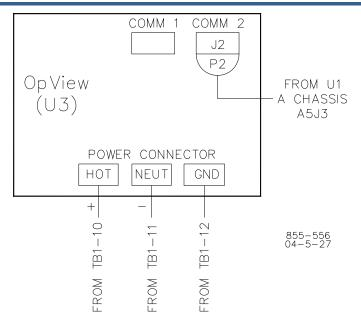
Figure 4-27. OpView Wiring Diagram
