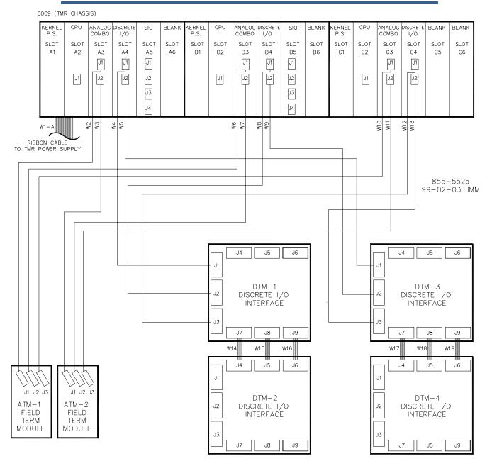
Figure 4-19. System Cable Layout Diagram
