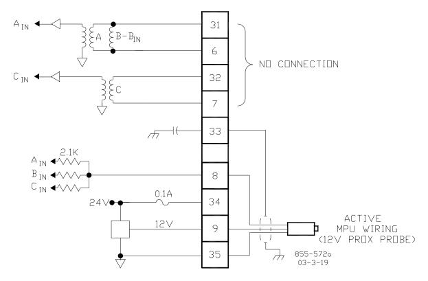
Figure 4-3b. Example 12 V Proximity Wiring Diagram
