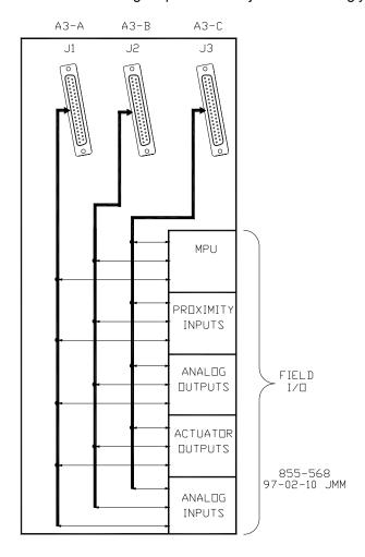
Figure 2-6. Analog Termination Module Diagram
