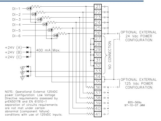
Figure 4-9. Optional External Contact Wetting Configurations
