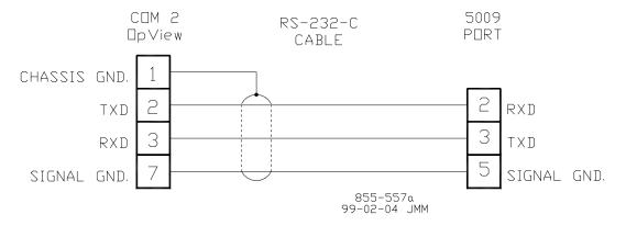
Figure 4-28. OpView Cable Diagram
