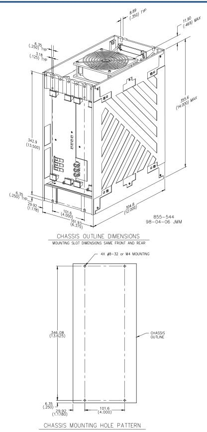
Figure 3-4c. Outline Drawing of 5009 Power Chassis
