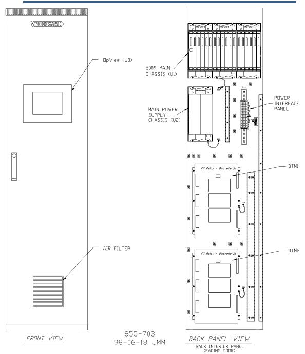
Figure 4-18a. Cabinet—Device Location Diagram
