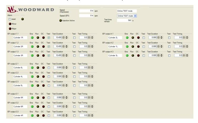
When an engine is running, the **Online TEST mode** can be selected from the drop down selector.
