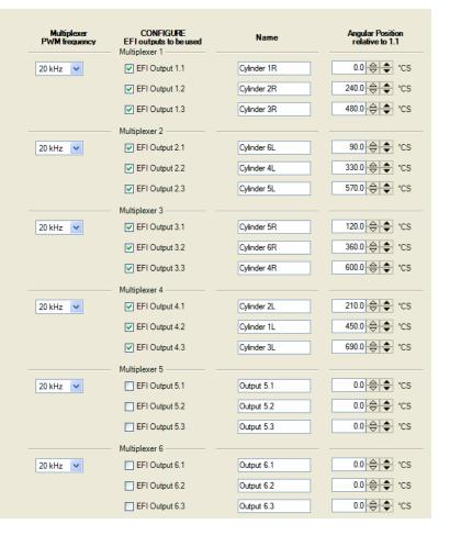
Up to 18 injector outputs can be used. They are distributed over 6 multiplexers of 3 injectors each. Per multiplexer group, only 1 injector can be active at any time. Using the firing order of the engine, the injectors output shall be distributed to cylinders such that there will be no overlap in activation time of injectors within the same multiplexer group.
