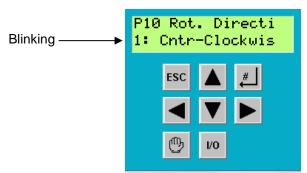
9. By using the **up and down keys**, set the value of **P10** according to the direction of rotation (see table below):
