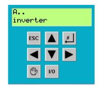
9. Navigate to the parameter **A00** using the **up and down keys** if needed, then press "**Enter key**". "0: inactive" should appear blinking on the second line of the display.
