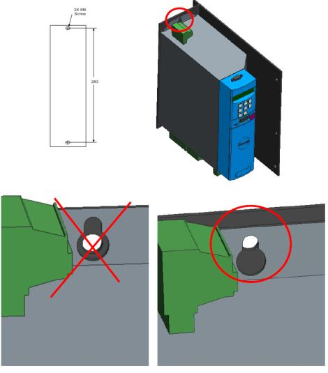
Figure 5-3. Driver Mounting Profile Dimension
