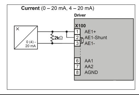
**NOTICE** The 2 k $\Omega$  external shunt resistor attached to the connector for X100 is REQUIRED for proper operation of the driver. It is installed and tested at the factory. <u>Do not remove</u>.
