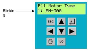
5. By using the **up and down keys** set the value of **P11** according to the motor type (see table below):
