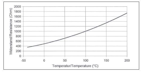
Figure 8-1. Motor Temperature Sensor Diagram
