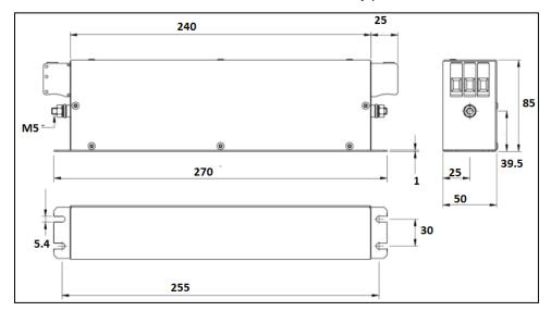
Figure 5-5. 1326-1125 Filter Assembly (mm)
