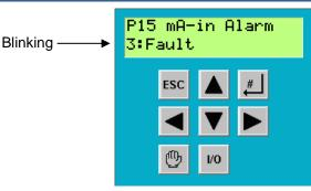
5. By using the up and down keys, set the value of P15 according to the required action (see table below):
