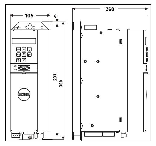
Figure 5-1. EM-80/300 Driver Dimensions (mm)
