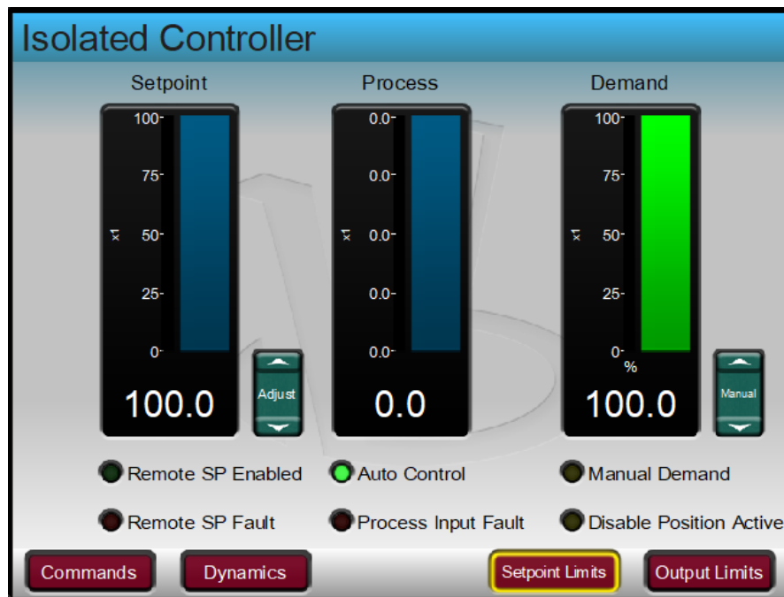
Figure 6-52. Isolated Controller Operation Screen in Service Menu
