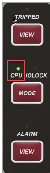
Figure 11-12. Front Panel CPU LED SYCON/BACKUP Indication
