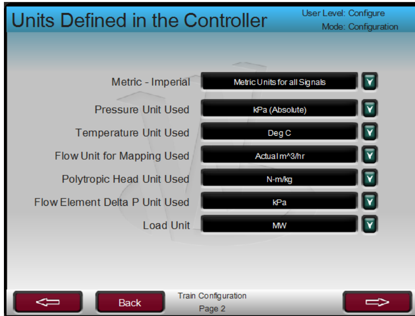
Figure 20-15. Units Defined in the Controller
