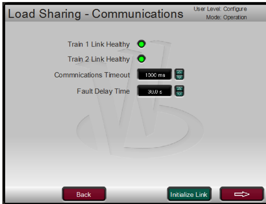
Figure 26-2. Service Screen- Load Sharing Communication
