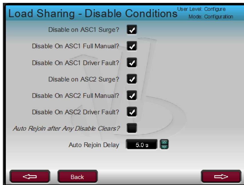
Figure 25-12. Service Screen- Load Sharing Disable Conditions Continued
