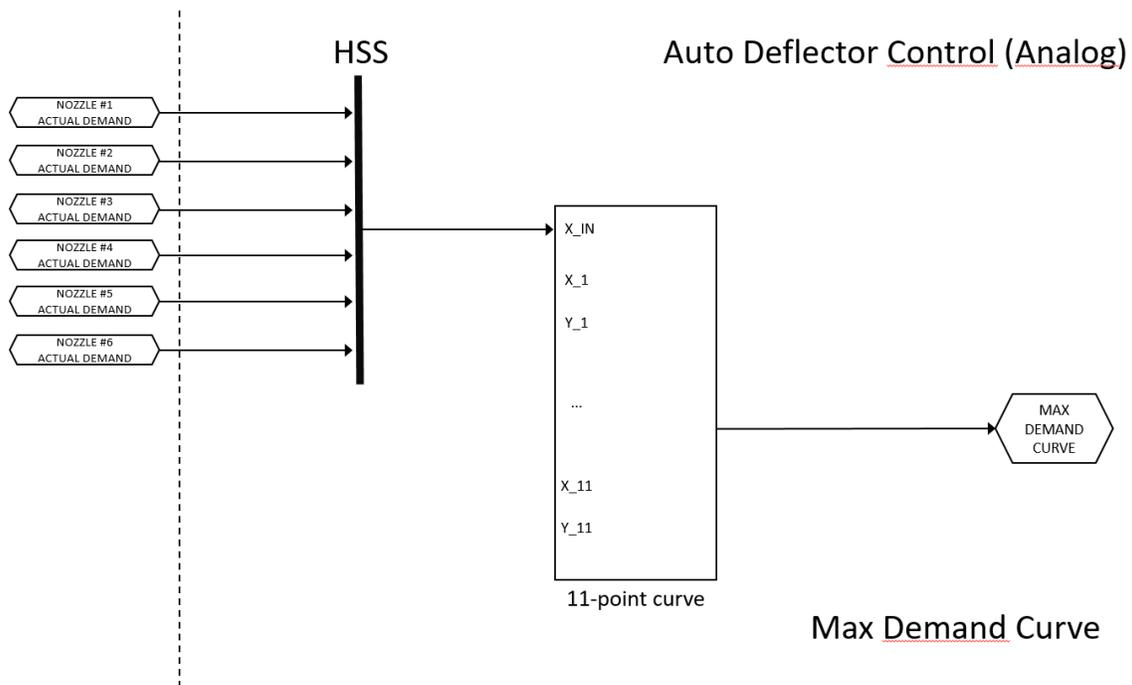
Figure F-16. Auto Deflector Control – Max Demand Curve (Analog)
