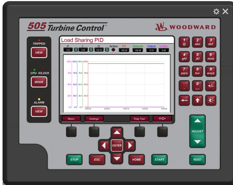
Figure 4-28. Load Sharing PID Screen
