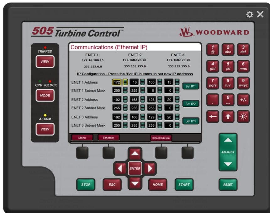
Figure 4-55. Communications (Ethernet IP) Screen
