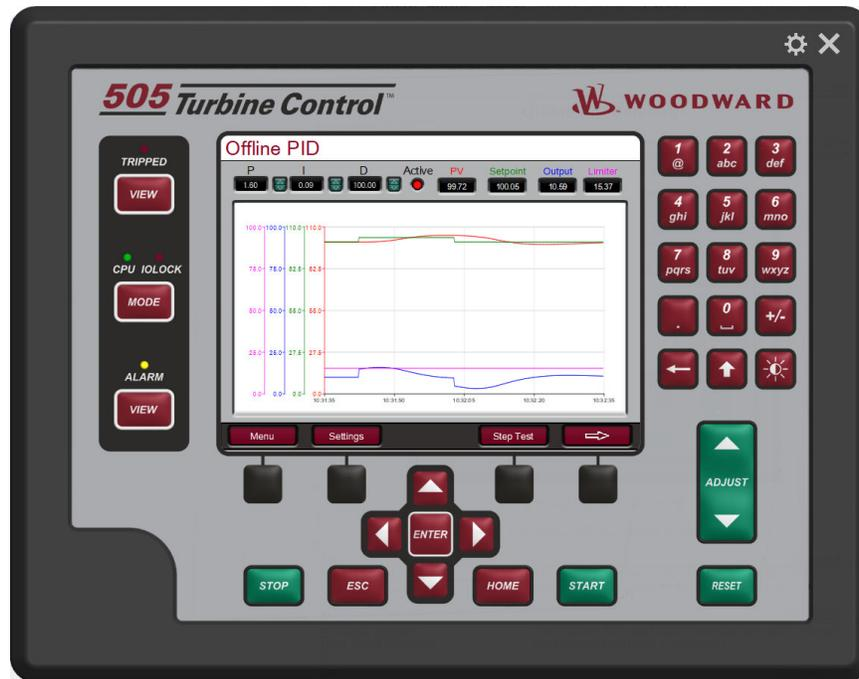
Figure 4-24. Offline PID Screen
