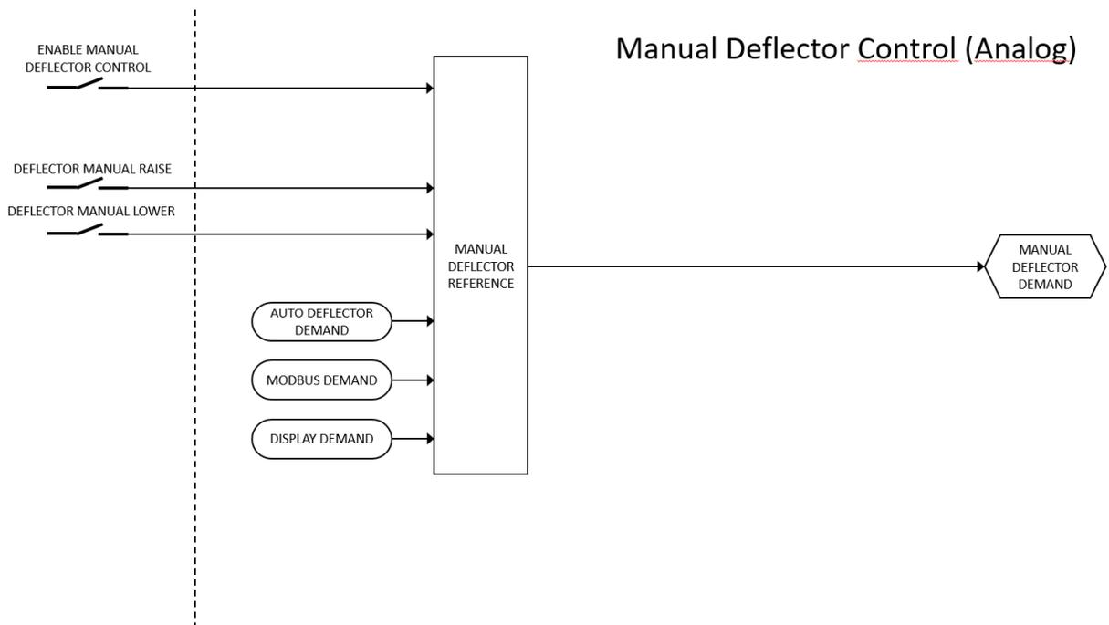
Figure F-14. Manual Deflector Control (Analog)
