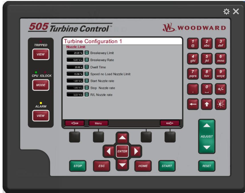
Figure 4-15. Turbine Configuration 1 Screen
