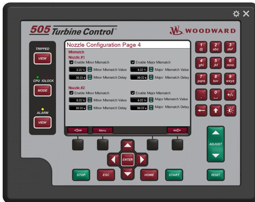
Figure 4-40. Nozzles Configuration Page 4 Screen
