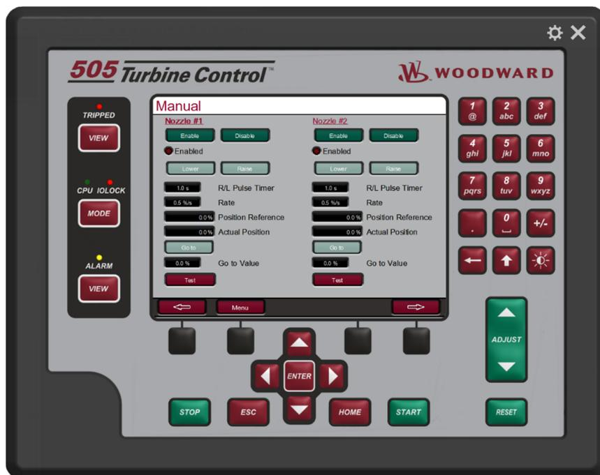
Figure 4-11. Manual (Individual Nozzles) Screen
