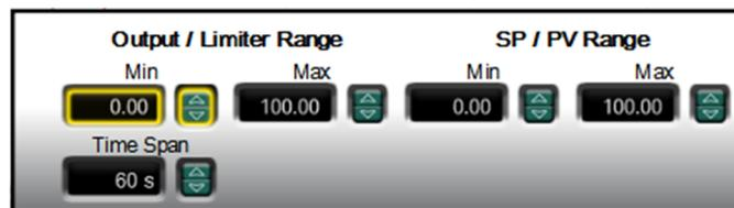
Figure 4-25. Offline PID Settings Screen
