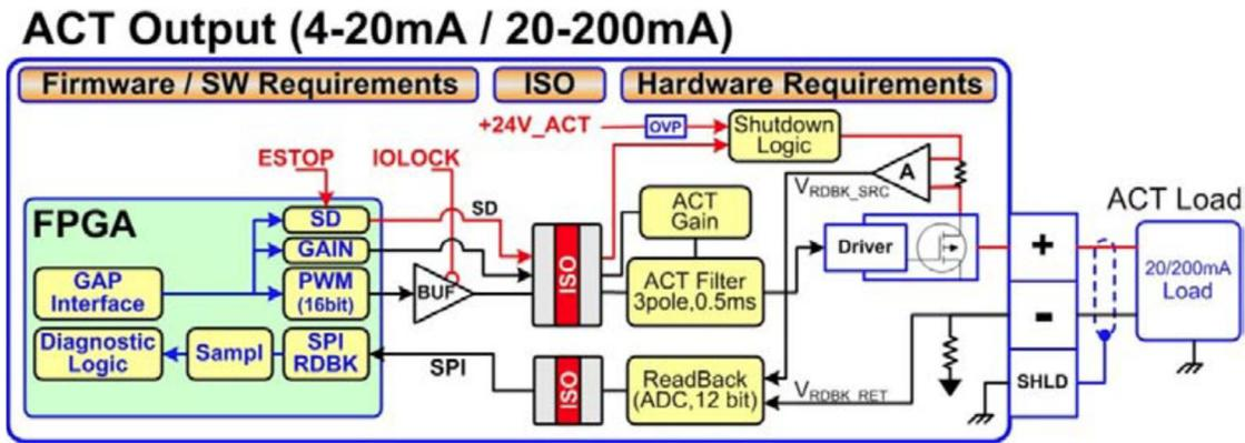
Figure 2-10. Actuator Output Block Diagram
