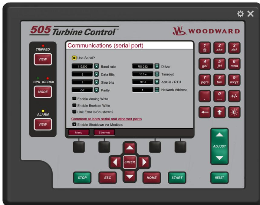
Figure 4-54. Communications (Serial Port) Screen
