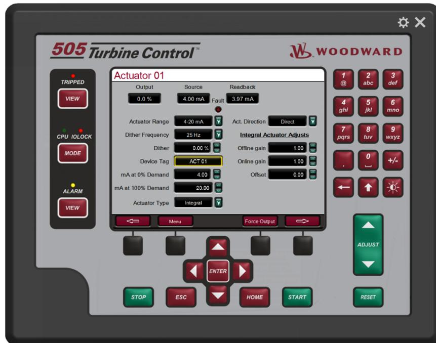
Figure 4-73. Actuator Outputs Screen
