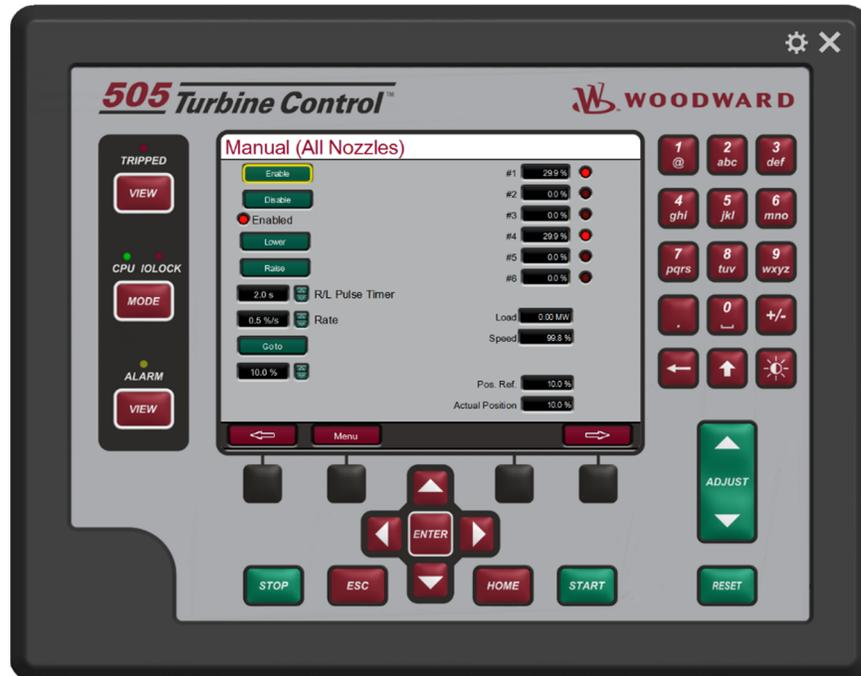
Figure 4-10. Manual (All Nozzles) Screen
