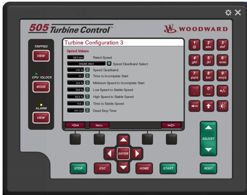
Figure 4-17. Turbine Configuration 3 Screen
