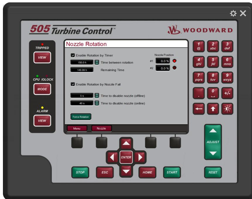
Figure 4-41. Nozzles Rotation Screen
