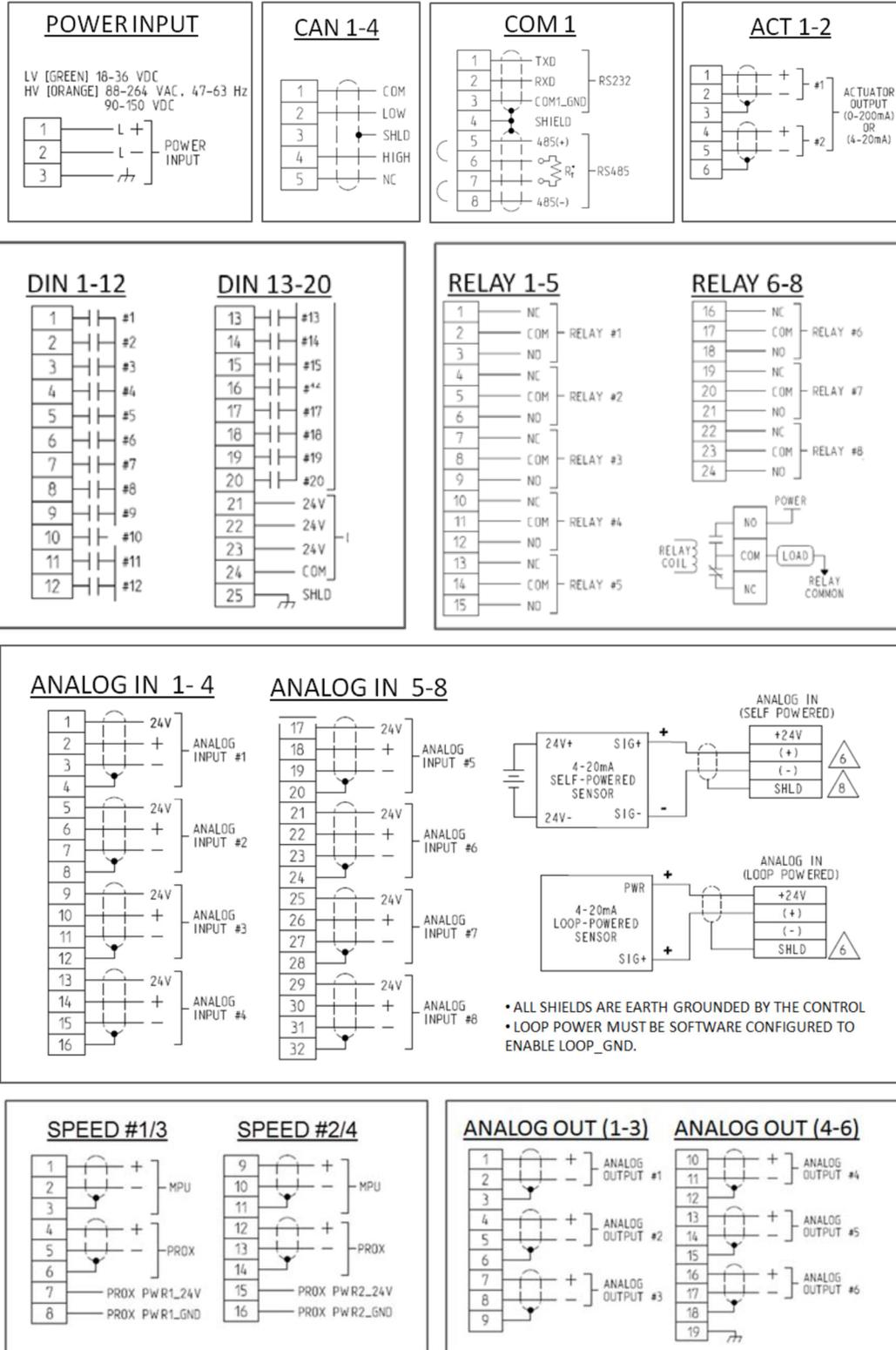
Figure 2-5. Terminal Block Connectors
