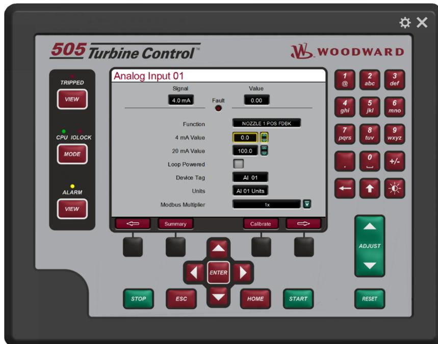
Figure 4-62. Analog Inputs Screen
