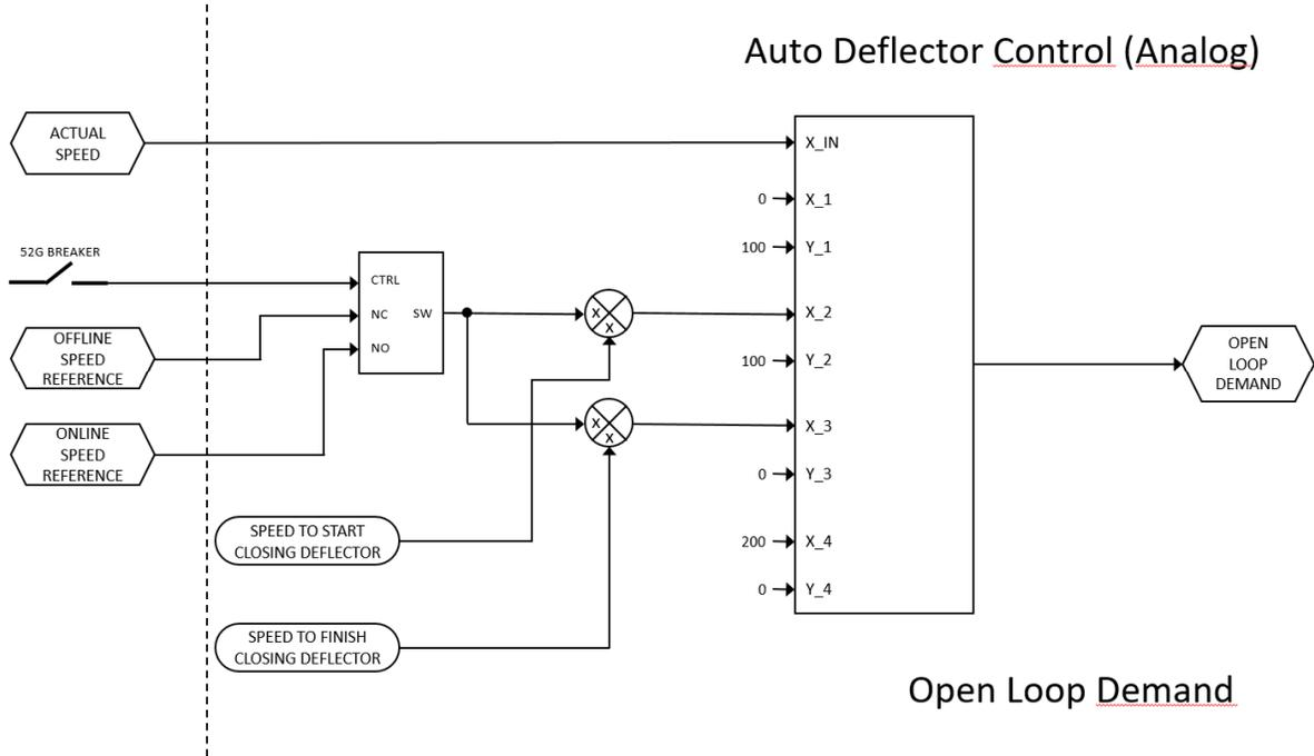
Figure F-15. Auto Deflector Control – Open Loop Demand (Analog)
