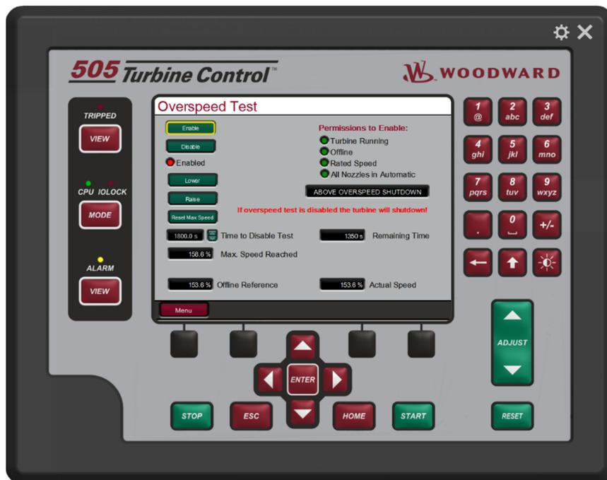
Figure 4-52. Overspeed Test Screen
