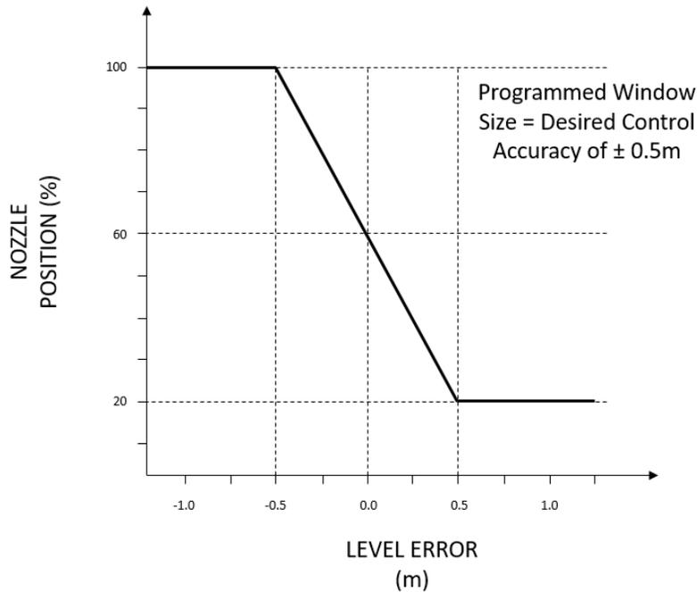
Figure 3-4. Pond Level Control Accuracy
