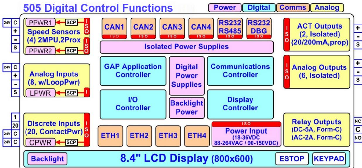
Figure 2-1. Functional Block Diagram (505 Control)
