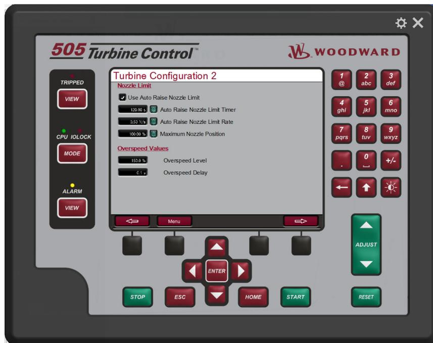
Figure 4-16. Turbine Configuration 2 Screen
