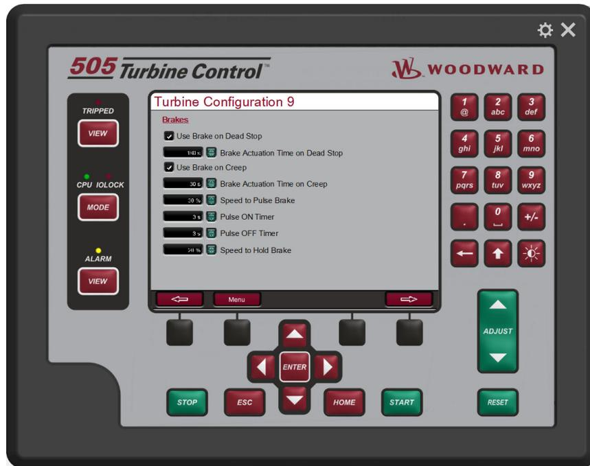
Figure 4-23. Turbine Configuration (9/9) Screen
