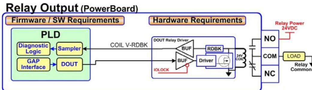
Figure 2-12. Relay Output Block Diagram
