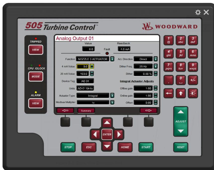
Figure 4-70. Analog Outputs Screen
