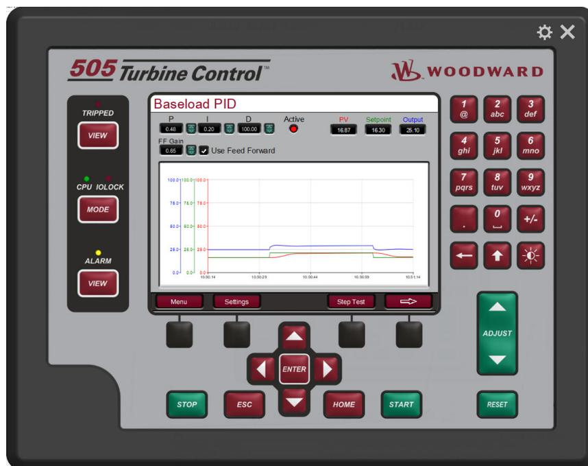
Figure 4-30. Baseload PID Screen
