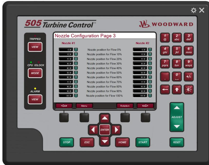
Figure 4-39. Nozzles Configuration Page 3 Screen
