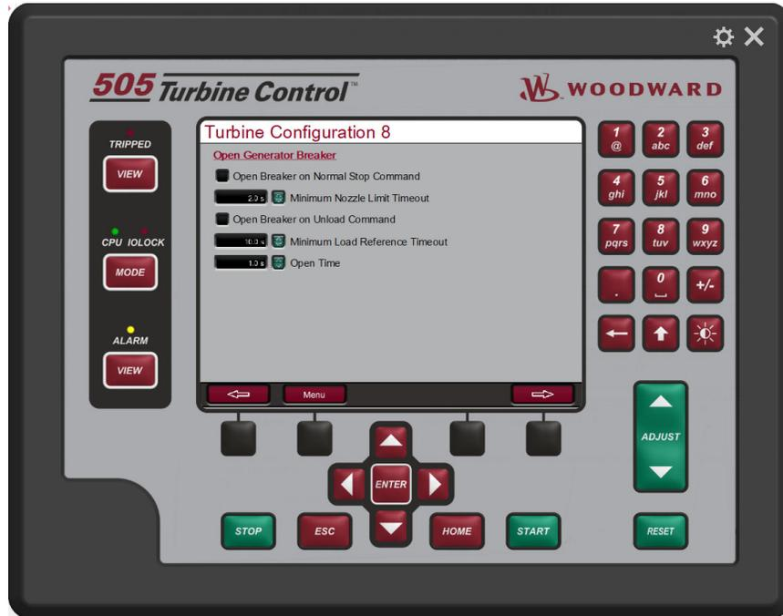
Figure 4-22. Turbine Configuration 8 Screen
