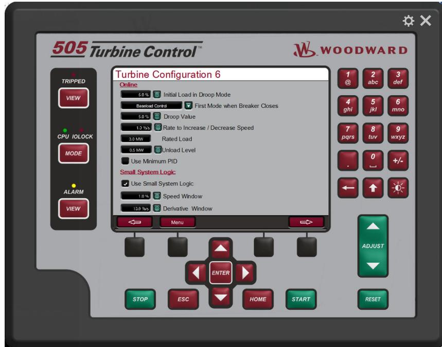
Figure 4-20. Turbine Configuration 6 Screen
