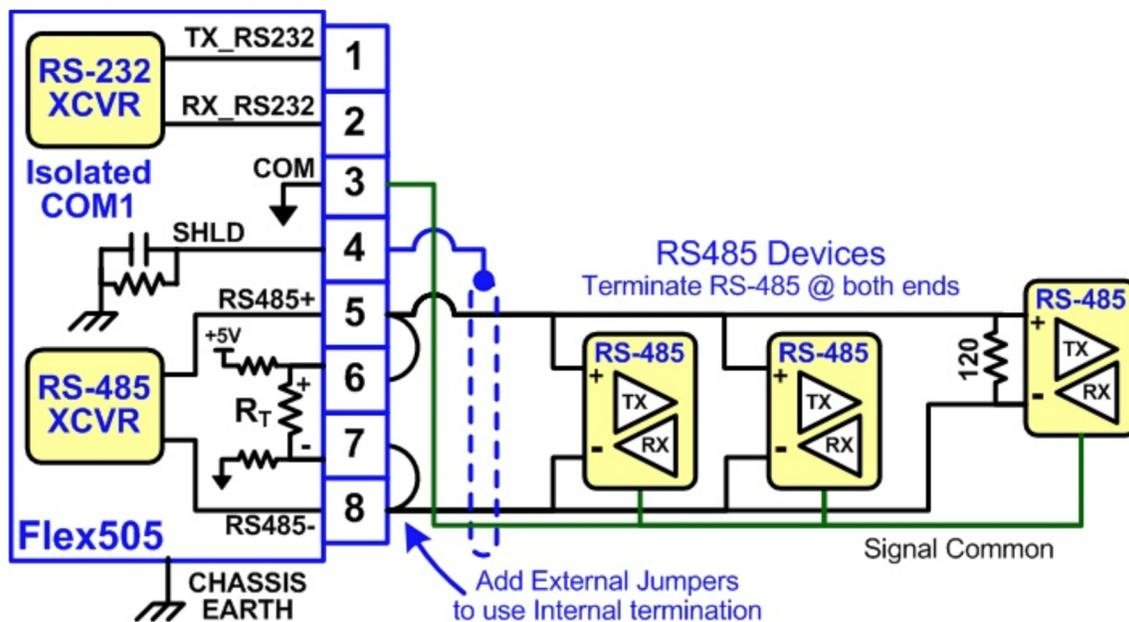
Figure 2-3. COM1 Example RS-485 wiring
