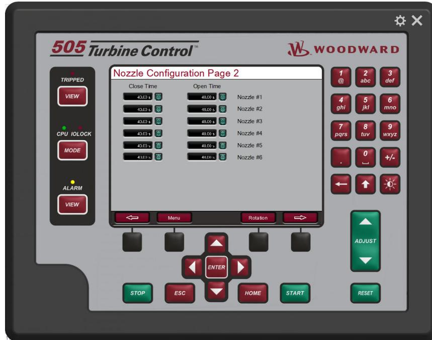
Figure 4-38. Nozzles Configuration Page 2 Screen
