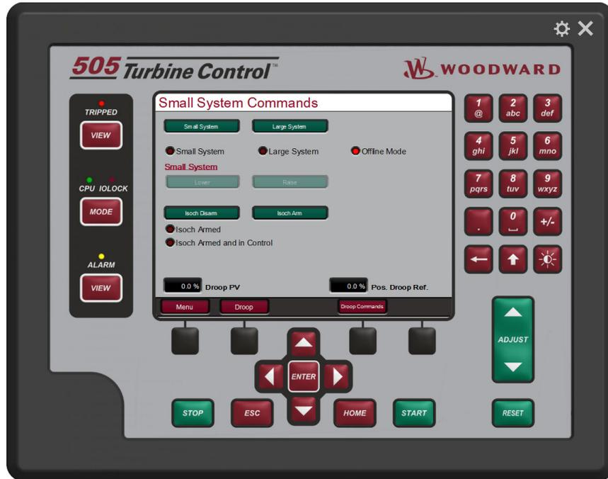
Figure 4-49. Small System Mode Commands Screen
