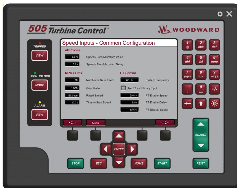
Figure 4-64. Speed Signal (Common Configuration) Screen
