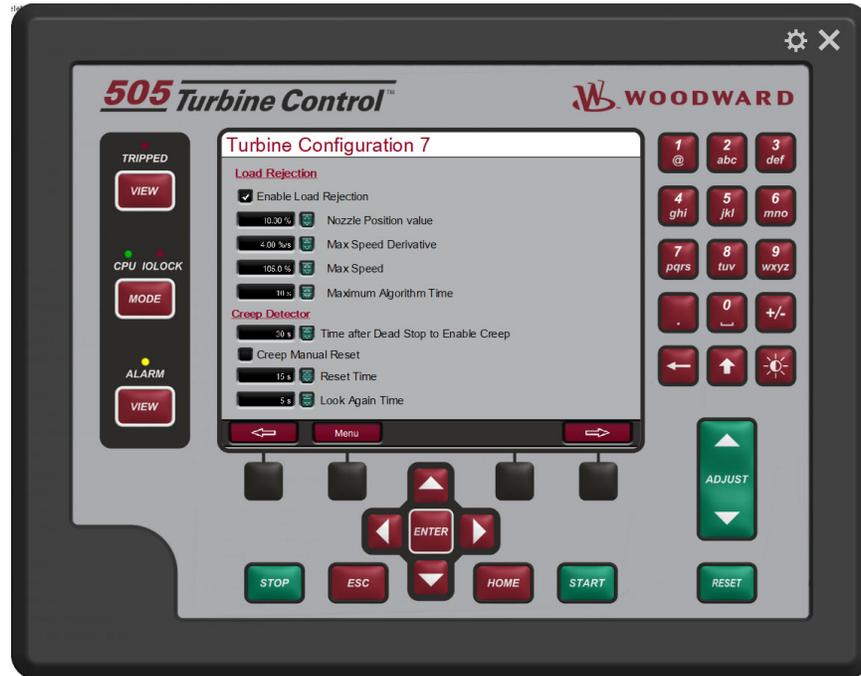
Figure 4-21. Turbine Configuration 7 Screen
