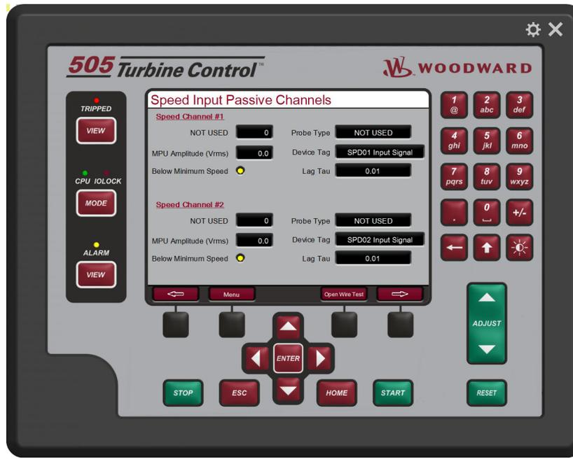
Figure 4-65. Speed Signal (Passive Channels) Screen
