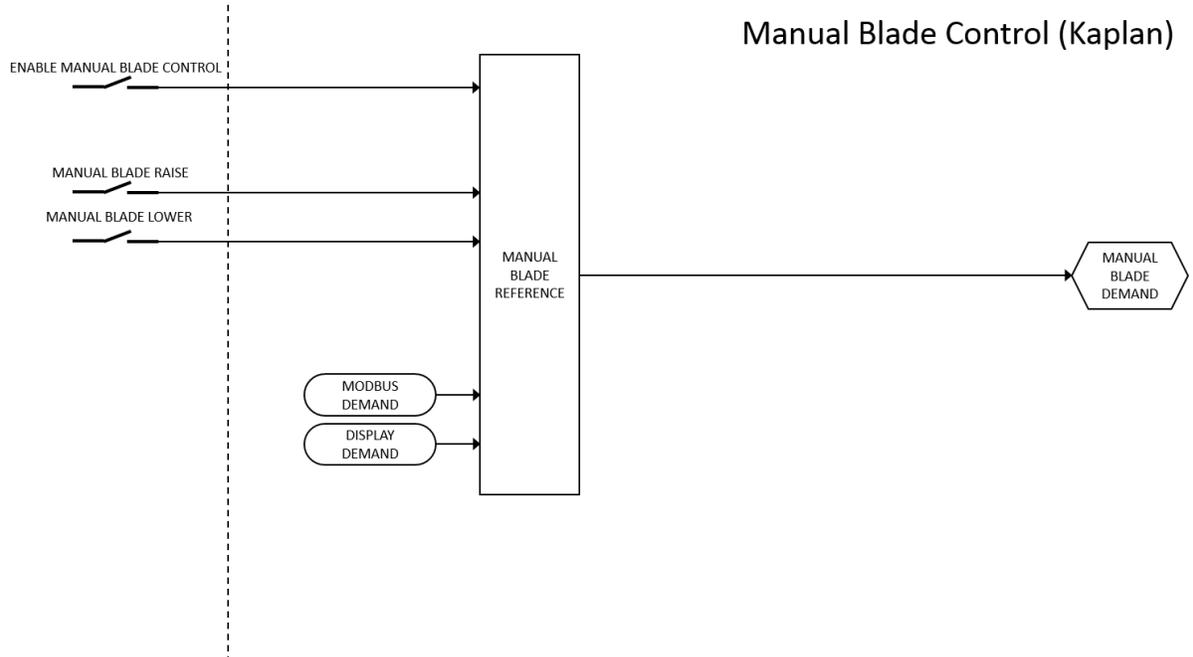
Figure F-15. Manual Blade Control (Kaplan)
