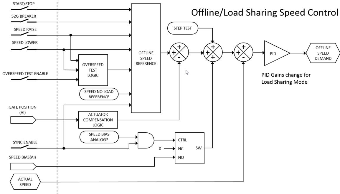
Figure F-3. Offline/Load Sharing Speed Control
