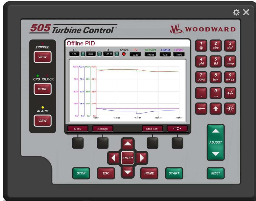
Figure 4-28. Offline PID Screen
