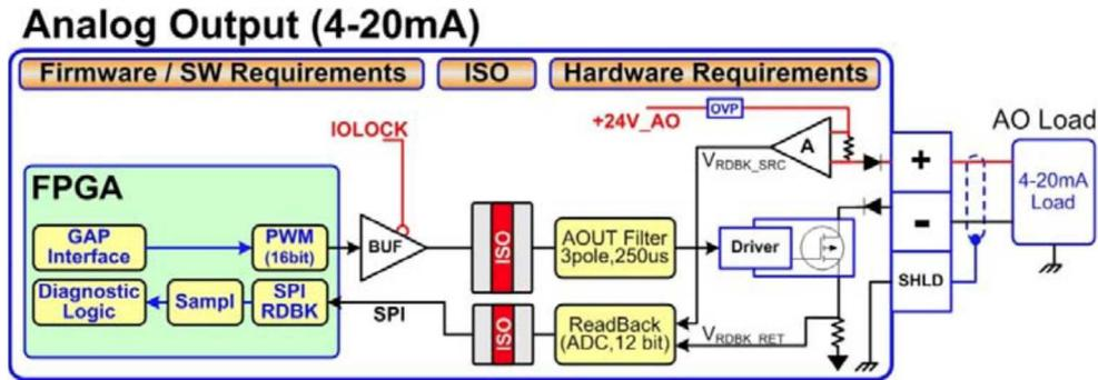
Figure 2-9. Analog Output Block Diagram
