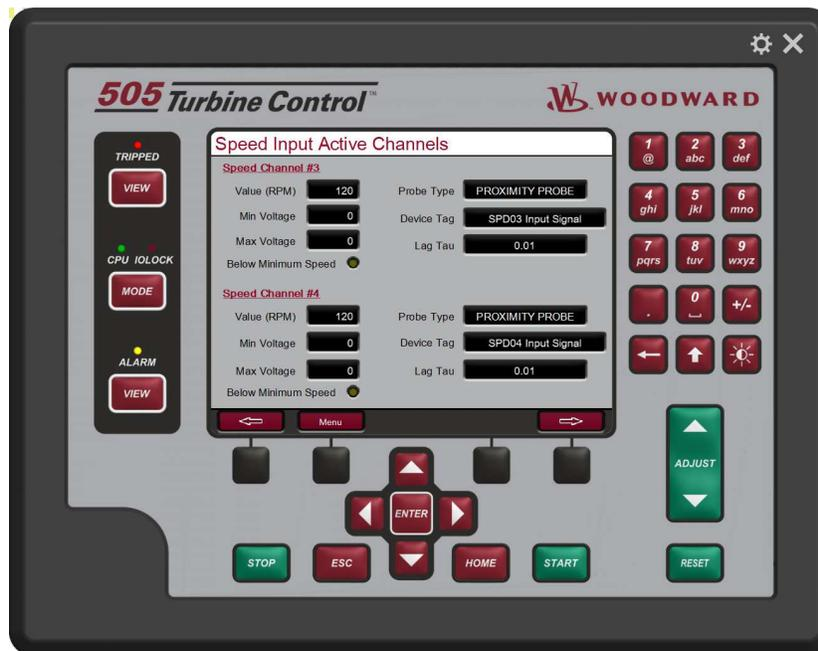
Figure 4-68. Speed Signal (Active Channels) Screen
