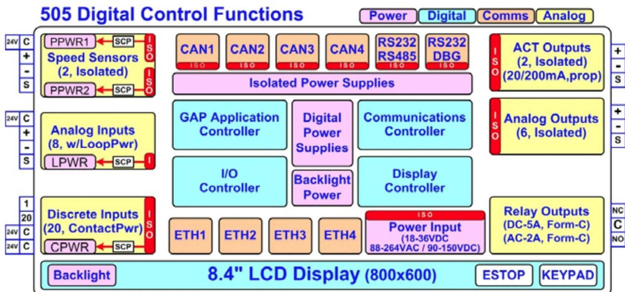
Figure 2-1. Functional Block Diagram (505 Control)
