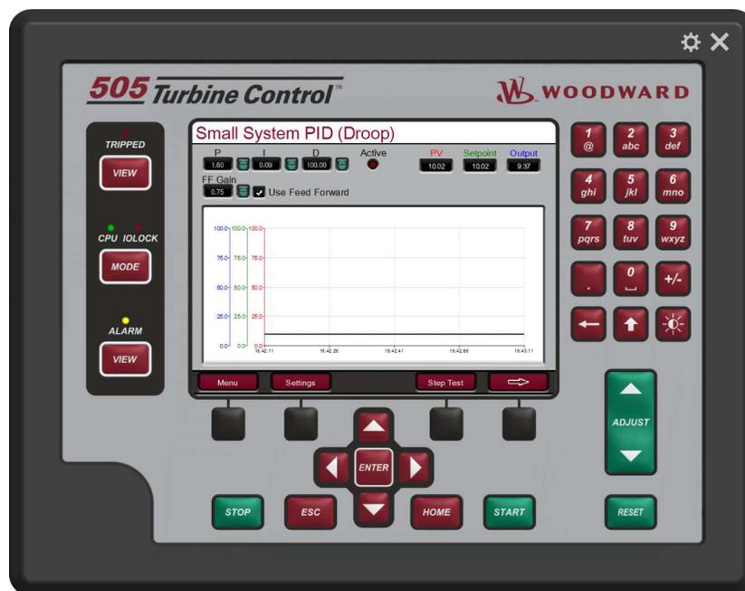
Figure 4-36. Small System PID (Droop) Screen
