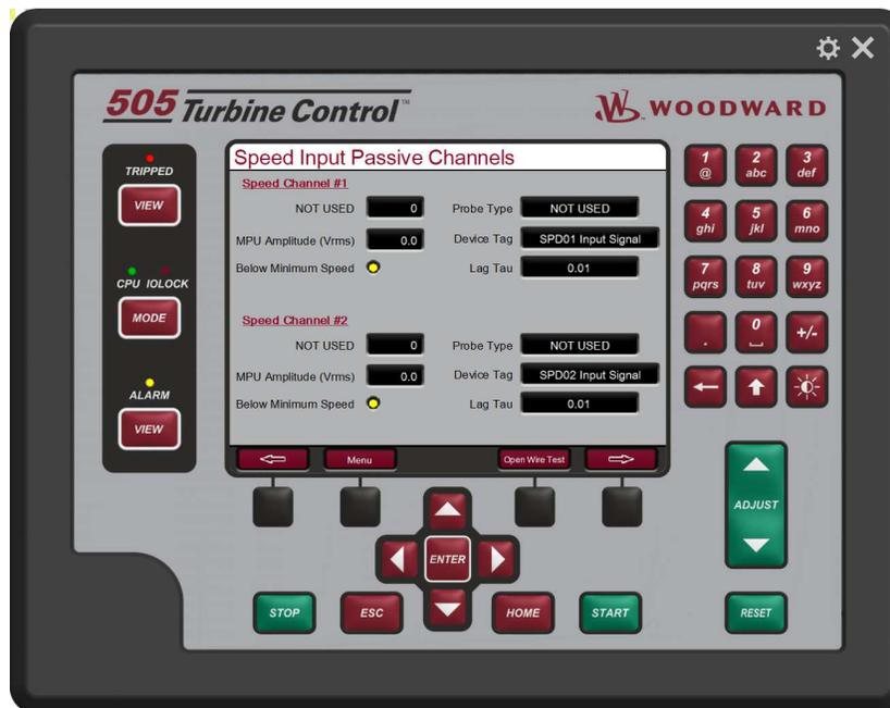
Figure 4-67. Speed Signal (Passive Channels) Screen
