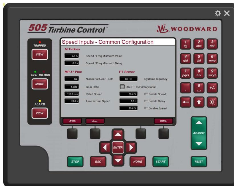
Figure 4-66. Speed Signal (Common Configuration) Screen
