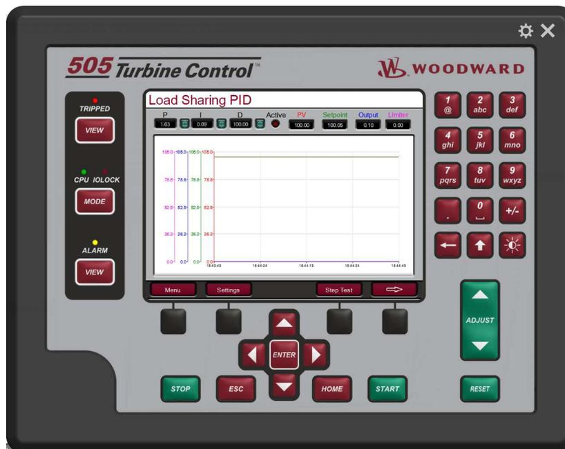
Figure 4-32. Load Sharing PID Screen
