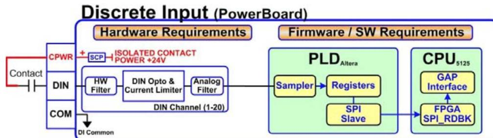
Figure 2-11. Discrete Input Block Diagram
