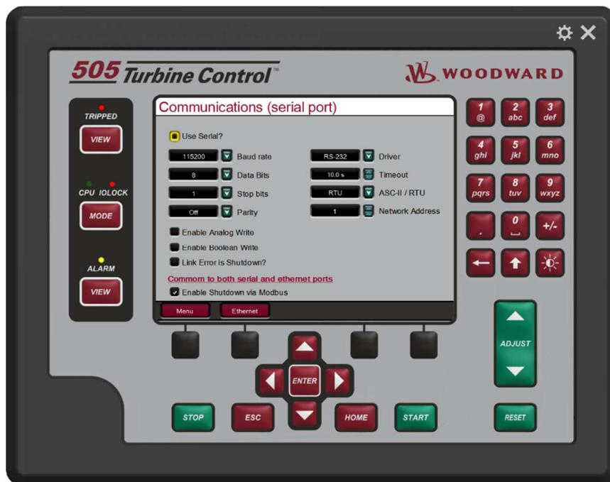
Figure 4-55. Communications (Serial Port) Screen
