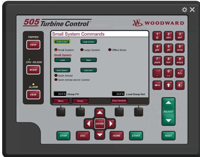
Figure 4-48. Isolated Mode Commands Screen
