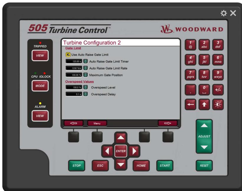
Figure 4-19. Turbine Configuration 2 Screen
