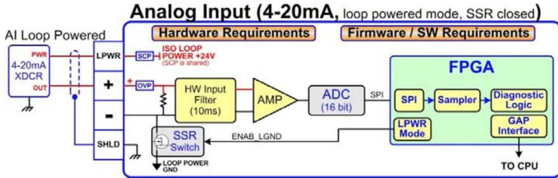
Figure 2-8. Analog Input – Loop-Powered Block Diagram
