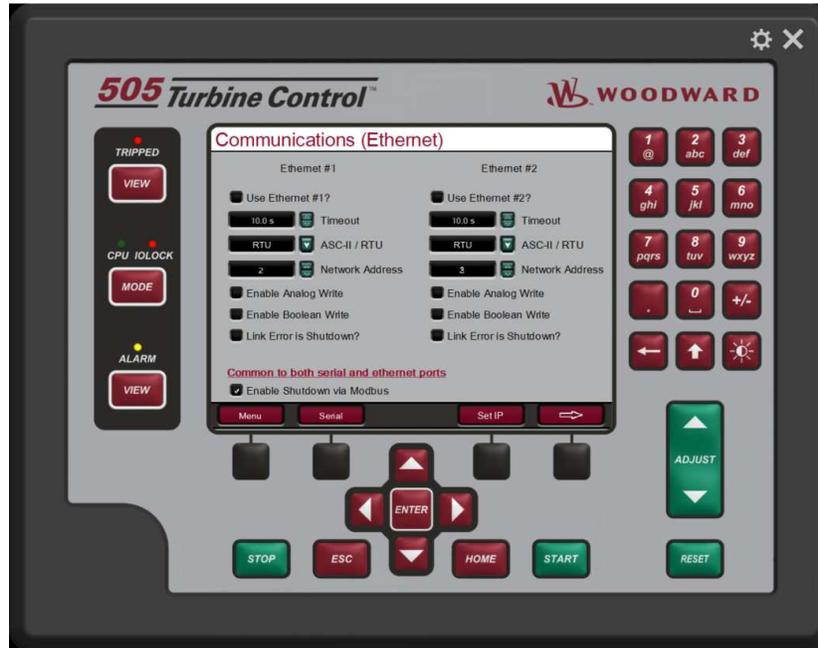
Figure 4-56. Communications (Ethernet) Screen
