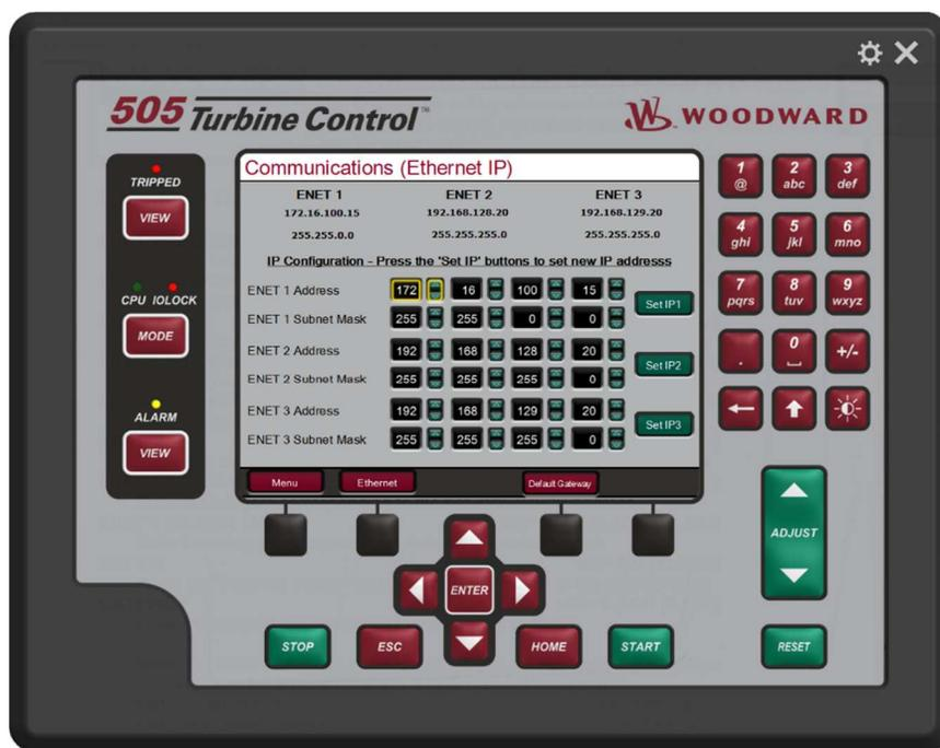
Figure 4-57. Communications (Ethernet IP) Screen
