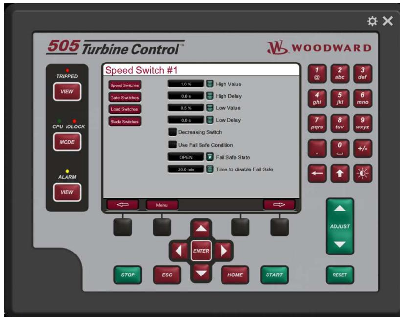
Figure 4-59 Speed Switches Screen
