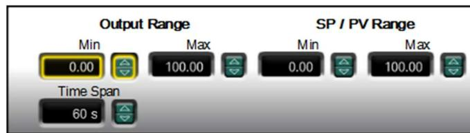
Figure 4-35. Baseload PID Settings Screen
