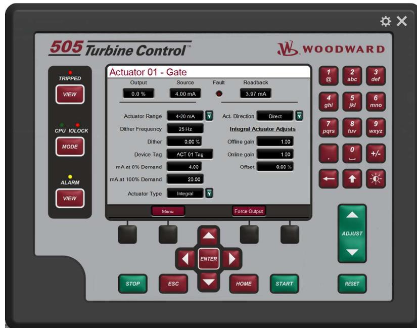
Figure 4-75. Actuator Output Screen
