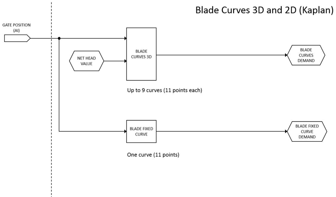
Figure F-16. Blade Curves 3D and 2D (Kaplan)
