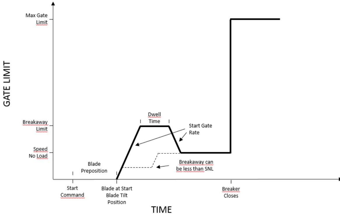
Figure 3-2. Gate Limit (Kaplan Turbine with Blade Preposition)
