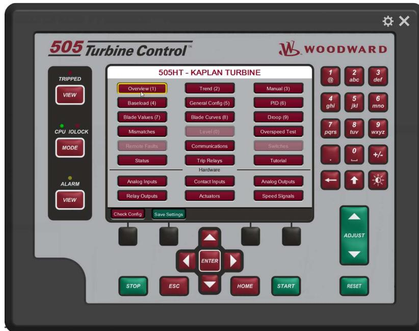
Figure 1-1. 505 Keypad and Display
