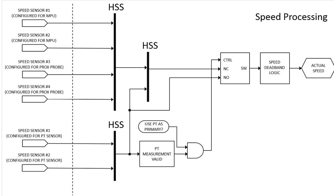
Figure F-1. Speed Processing
