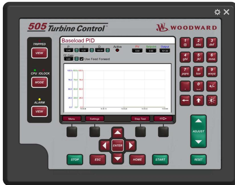
Figure 4-34. Baseload PID Screen
