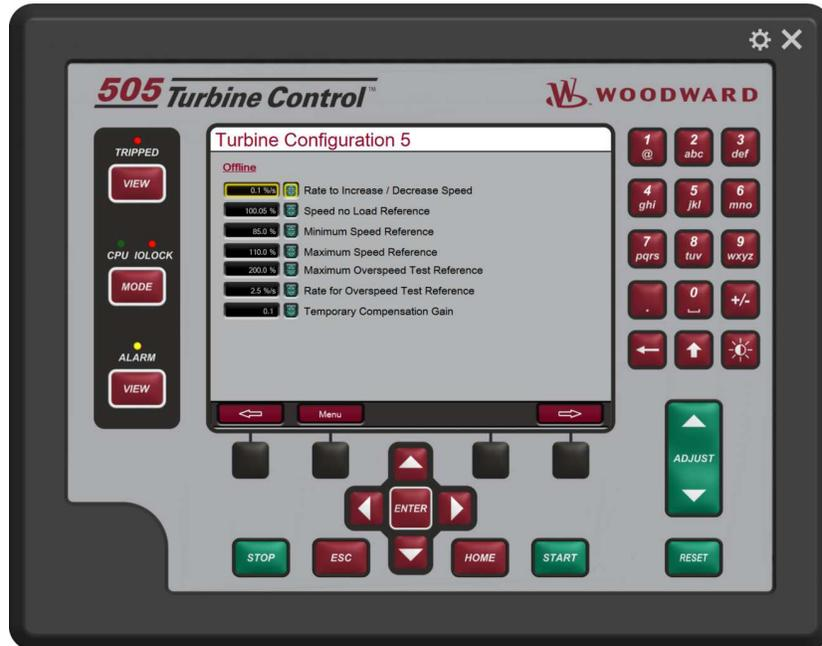
Figure 4-22. Turbine Configuration 5 Screen
