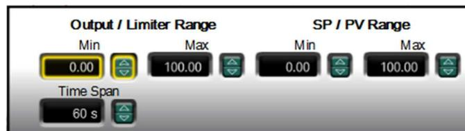
Figure 4-29 Offline PID Settings Screen
