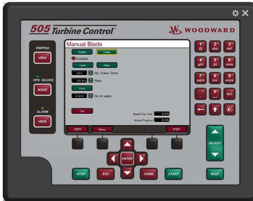
Figure 4-14. Manual Blade Screen
