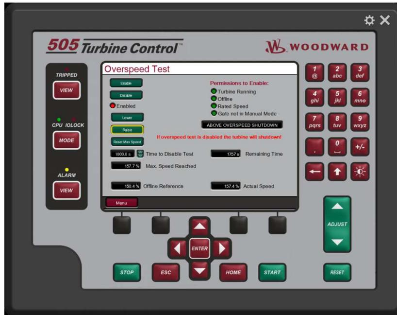
Figure 4-53. Overspeed Test Screen
