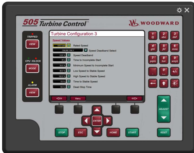
Figure 4-20. Turbine Configuration 3 Screen
