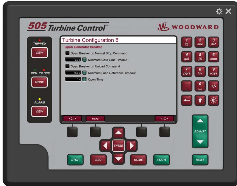
Figure 4-25. Turbine Configuration 8 Screen
