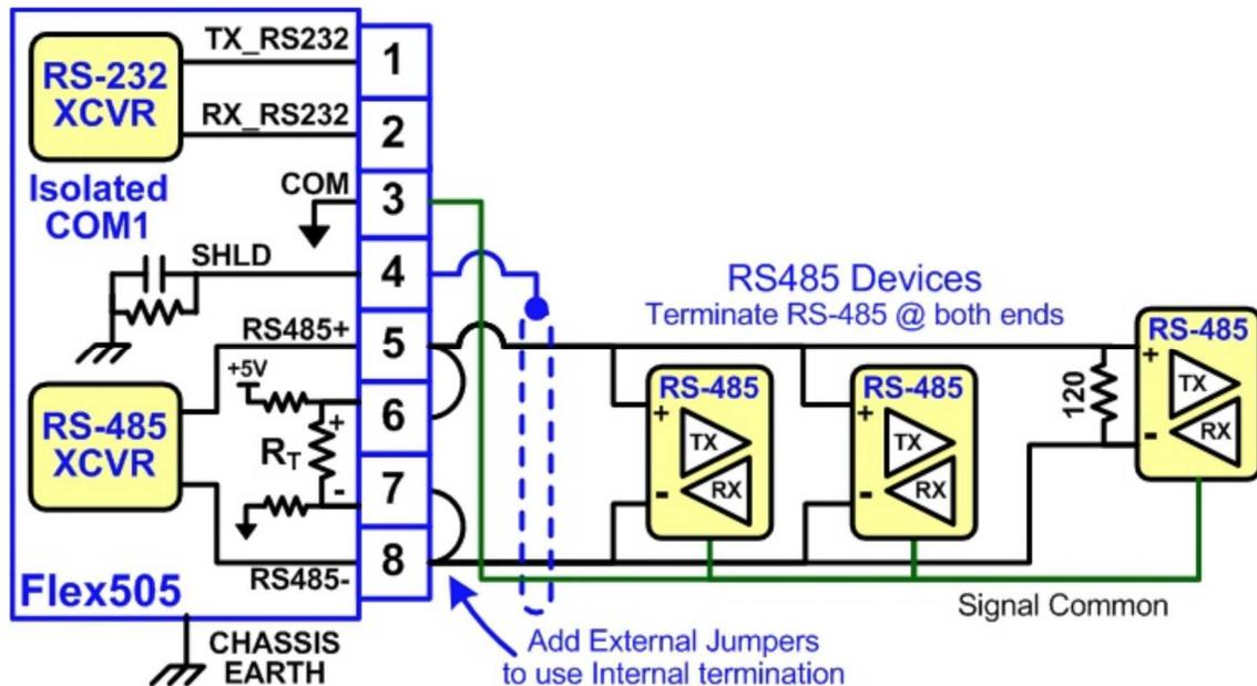
Figure 2-3. COM1 Example RS-485 wiring
