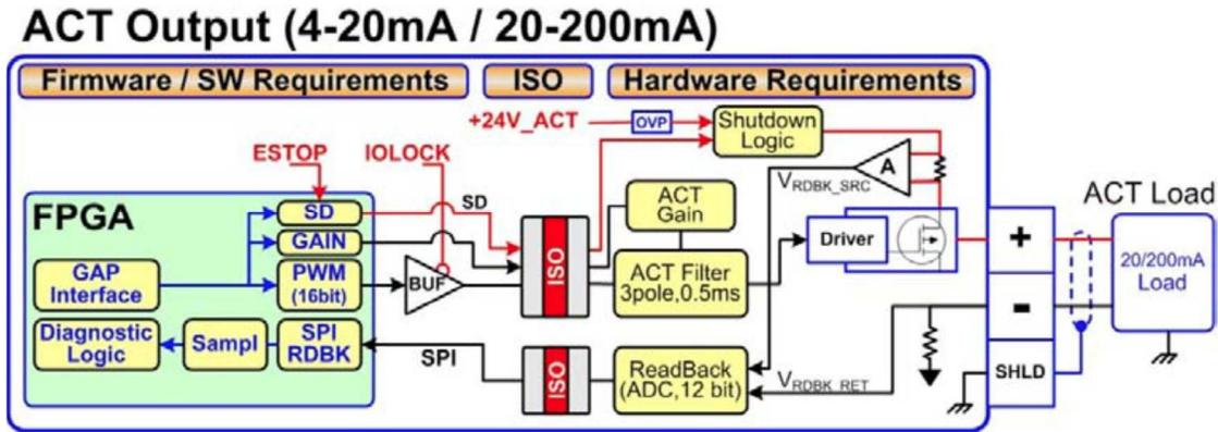
Figure 2-10. Actuator Output Block Diagram
