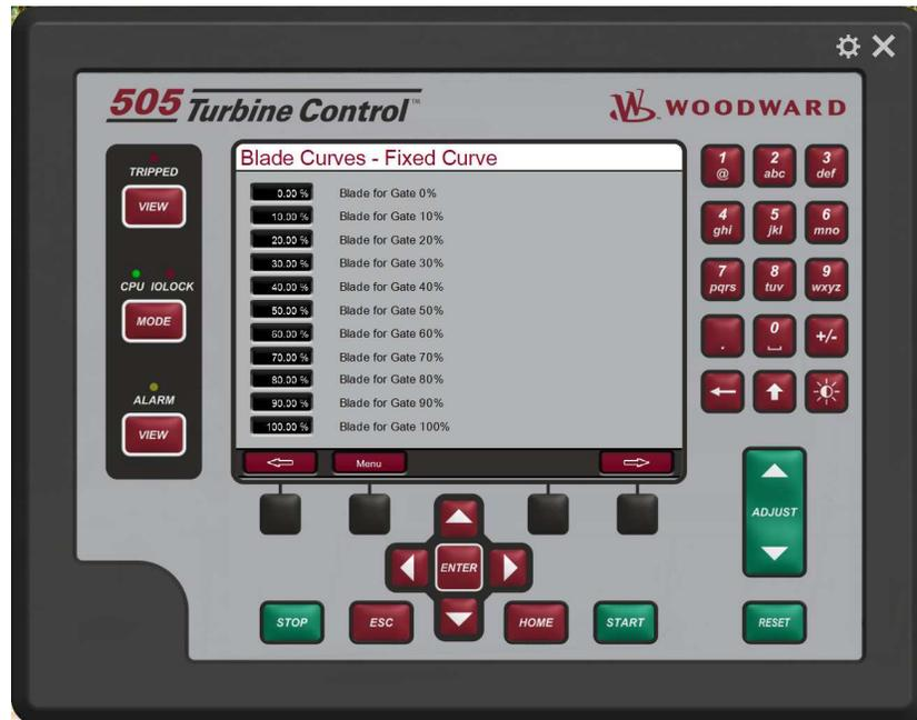
Figure 4-44. Blade Curves – Fixed Curve Screen
