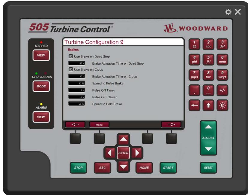
Figure 4-26. Turbine Configuration 9 Screen
