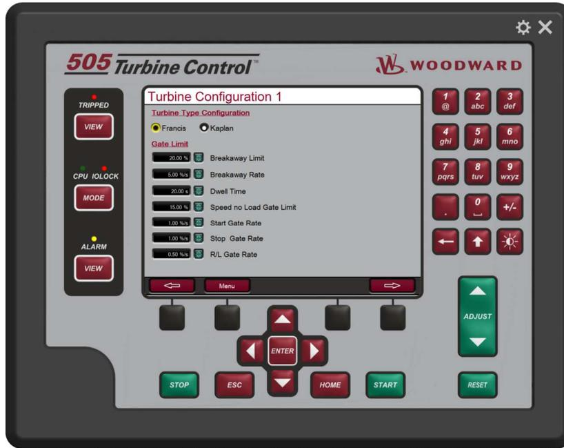
Figure 4-18. Turbine Configuration 1 Screen
