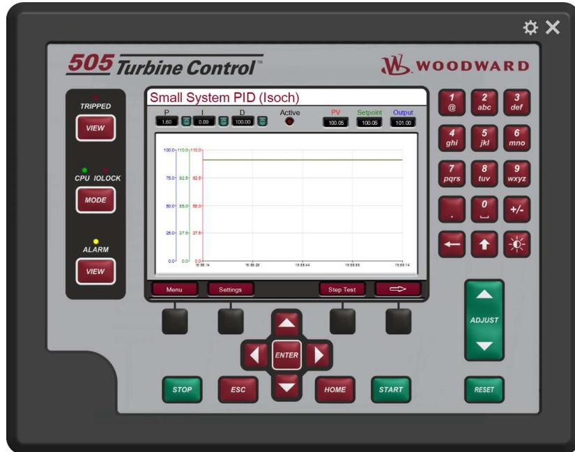
Figure 4-38. Offline PID Screen
