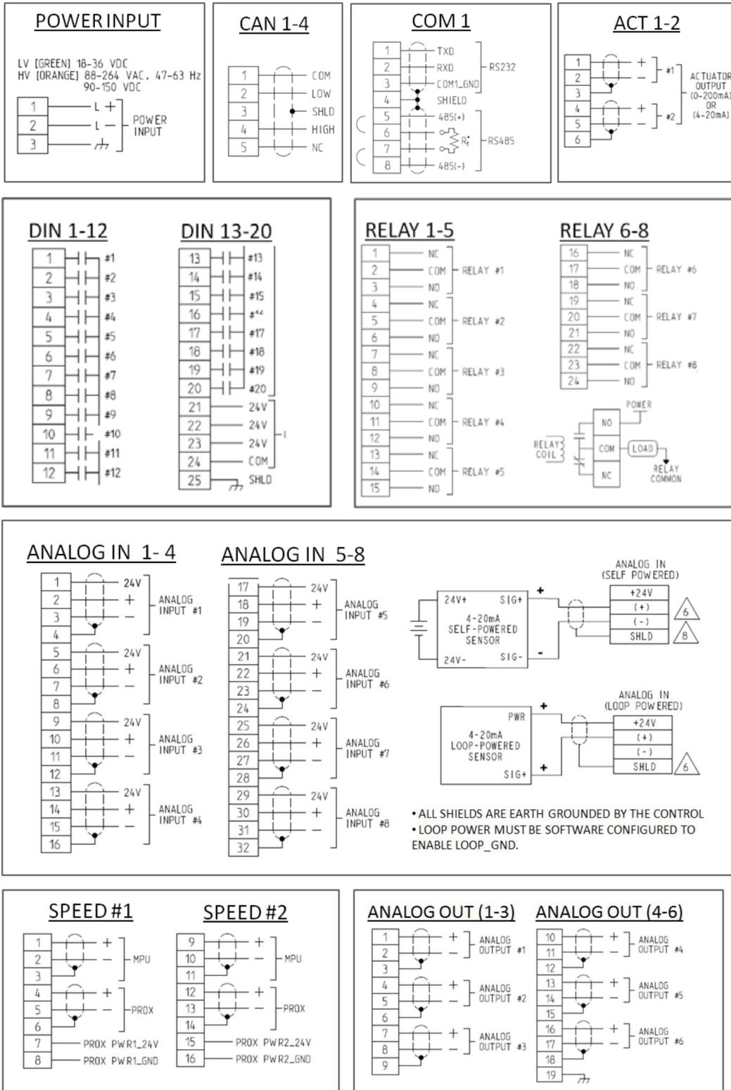
Figure 2-5. Terminal Block Connectors
