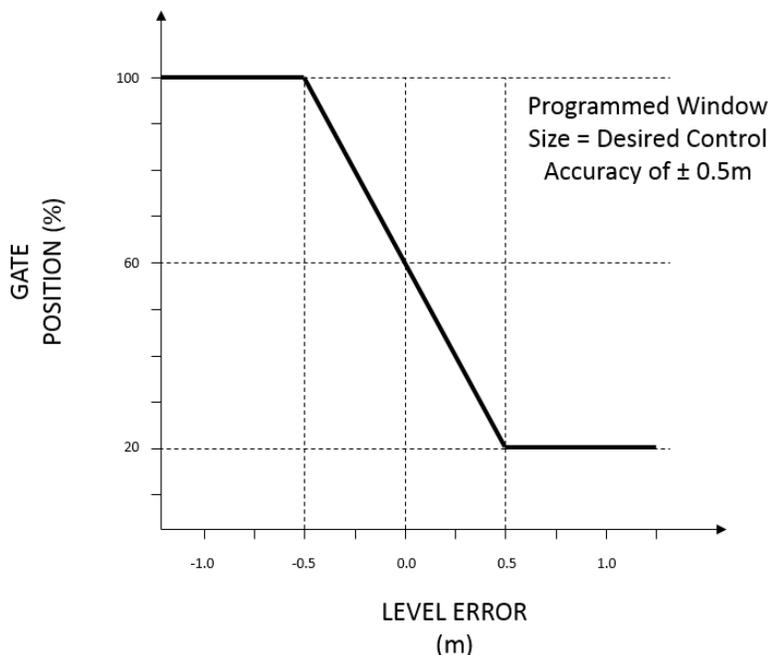
Figure 3-5. Pond Level Control Accuracy
