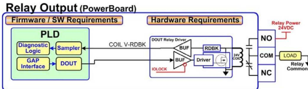
Figure 2-12. Relay Output Block Diagram
