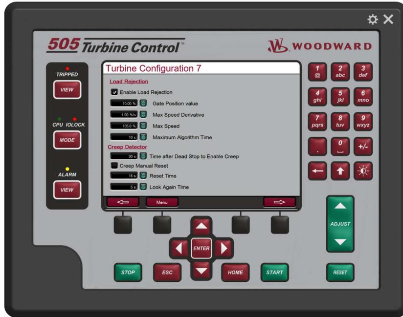
Figure 4-24. Turbine Configuration 7 Screen
