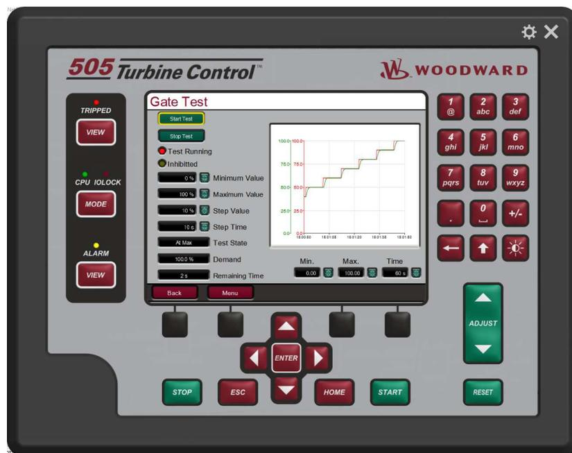
Figure 4-15. Gate / Blade Test Screen
