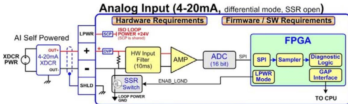
Figure 2-7. Analog Input – Self-Powered Block Diagram
