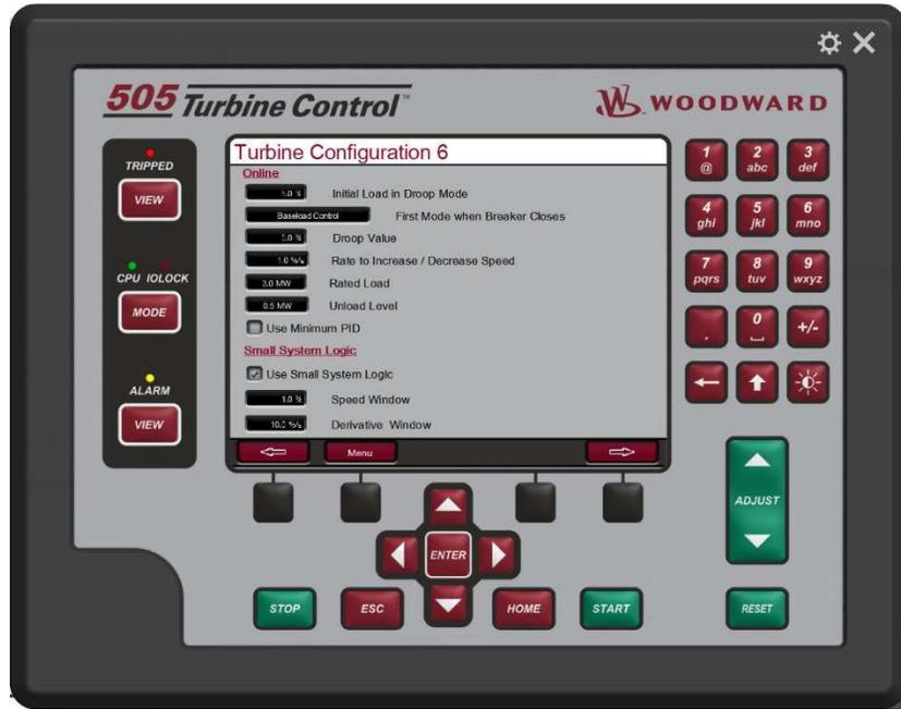
Figure 4-23. Turbine Configuration 6 Screen
