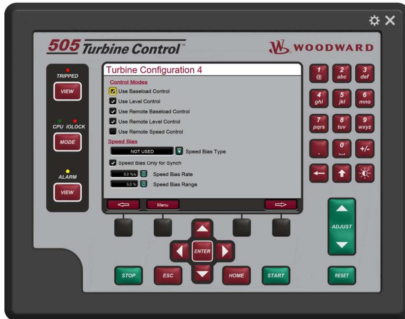
Figure 4-21. Turbine Configuration 4 Screen
