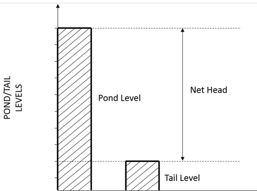
Figure 3-6. Net Head Calculation via Pond/Tail Level Inputs
