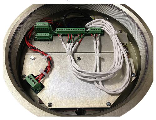
Figure 5-20. Recommended Wiring Strain Relief
