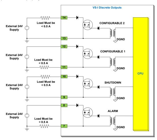
Figure 5-30. Discrete Output Connections
