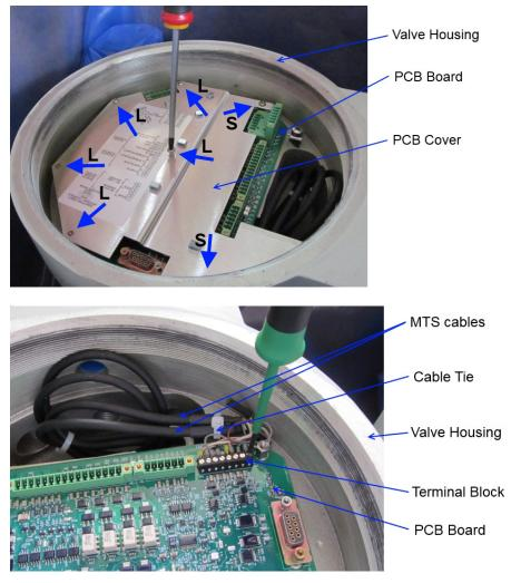
Figure 5-15. Remote Servo Only, PCBA Cover Removal
