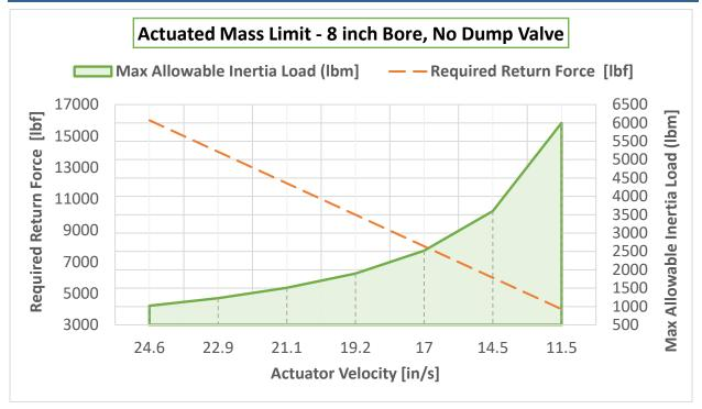
Figure 5-9. Actuated Mass Limit – 8-inch Bore, No Dump Valve
