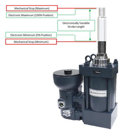
Figure 1-3. Hydraulic Power Cylinder - Stroke Adjustment Options
