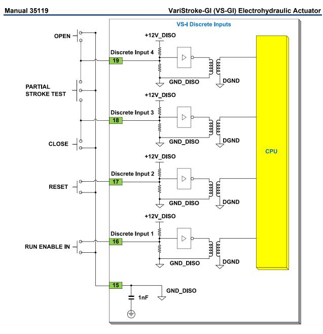
Figure 4-8. T&TV – Example Partial Stroke Test and Open/Close Signal Wiring
