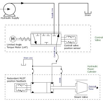
Figure 2-10. VS-GI Remote Hydraulic Schematic – Fail Extend with Externally Provided Closing Load
