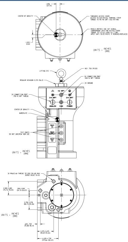
Figure 5-3b. VS-GI Remote Servo - Bolting Pattern and Installation Features – Side, Top, and Bottom View
