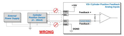
Figure 5-25. Example of Incorrect Cylinder Position Sensor Connection When Using External Power Supply
