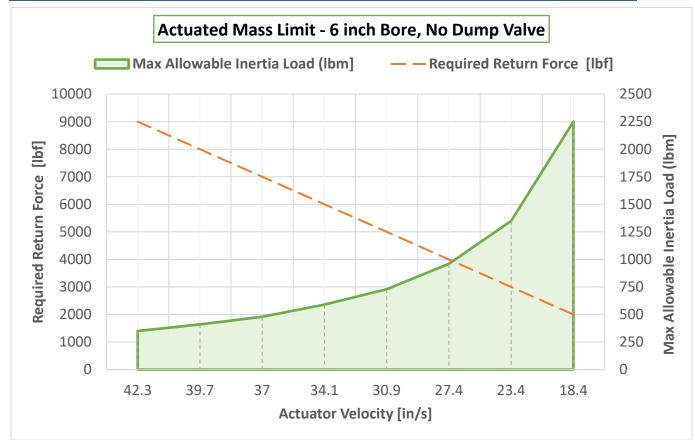
Figure 5-8. Actuated Mass Limit - 6-inch Bore, No Dump Valve
