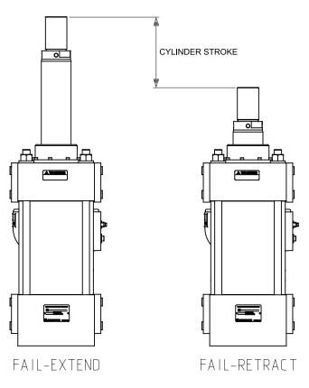
Figure 5-1. Hydraulic Rod Position for Different Cylinder Versions
