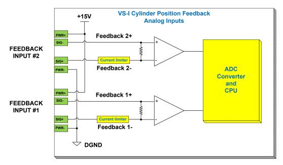
Figure 5-22. Final Cylinder Position Feedback Analog Input Connections
