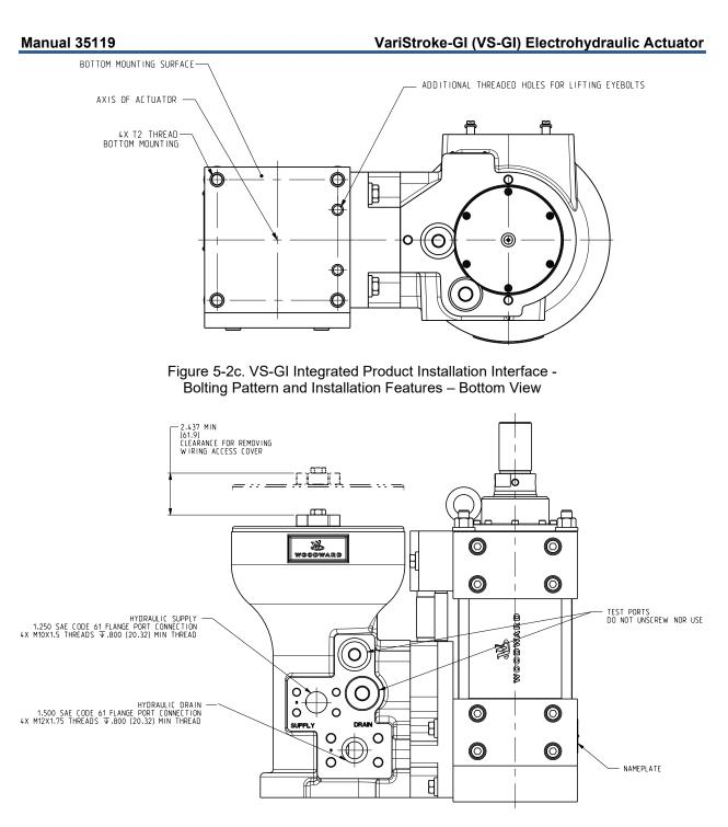
Figure 5-2d. VS-GI Integrated Product Installation Interface -Bolting Pattern and Installation Features – Side View
