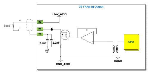
Figure 5-28. Analog Output Connection
