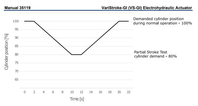
Figure 4-3. Example Partial Stroke Test
