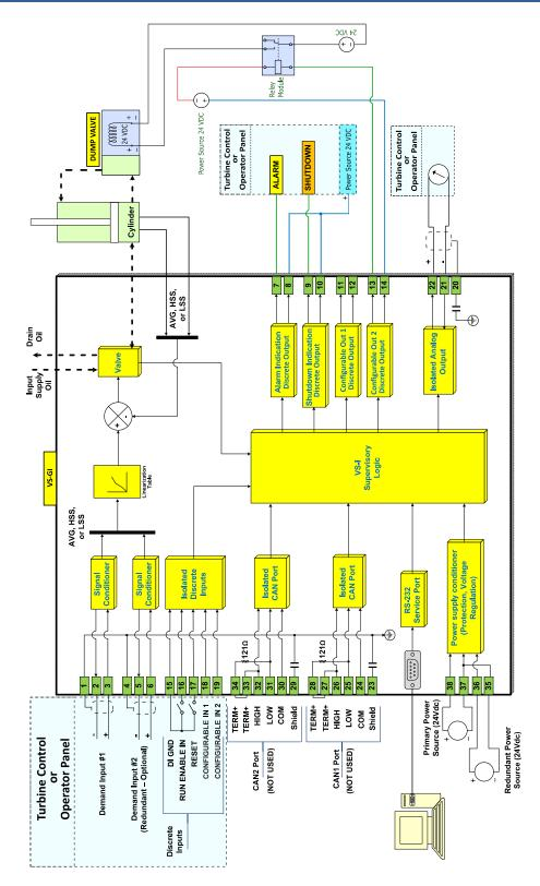
Figure 3-5. Example Wiring Diagram for Use of the VS-GI Discrete Output Signal to Control the Dump Valve
