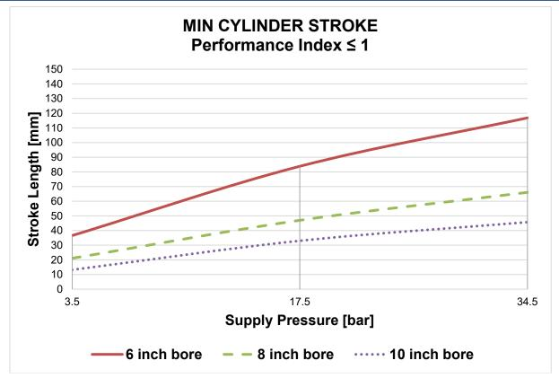
Figure 2-3. Performance Chart for 6", 8", and 10" Bore Actuators
