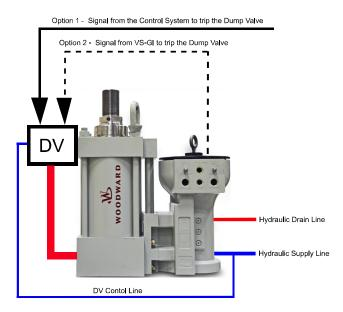
Figure 3-3. Dump Valve Schematic
