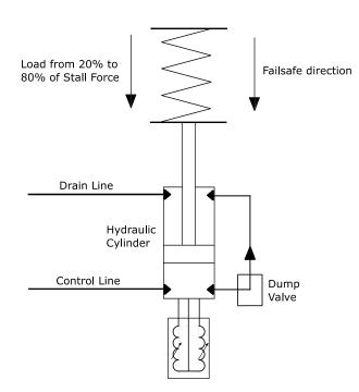
Figure 5-7. Hydraulic Cylinder with Load
