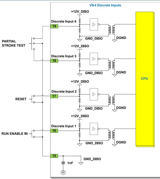
Figure 4-7. T&TV – Example Partial Stroke Test Functionality Wiring
