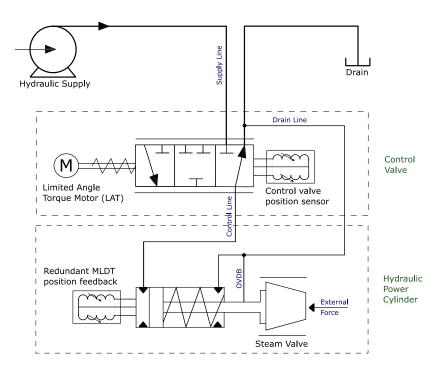
Figure 2-7. VS-GI Integrated Hydraulic Schematic – Fail Retract with Spring
