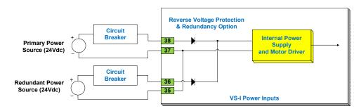
Figure 5-16. Power Supply Input Connections
