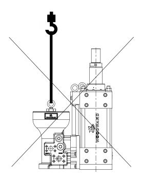
Figure 5-5. Incorrect Lifting Method
