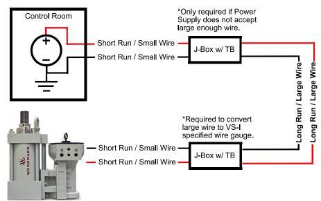
Figure 5-19. Example of wire gauge step-up, step-down to achieve longer runs
