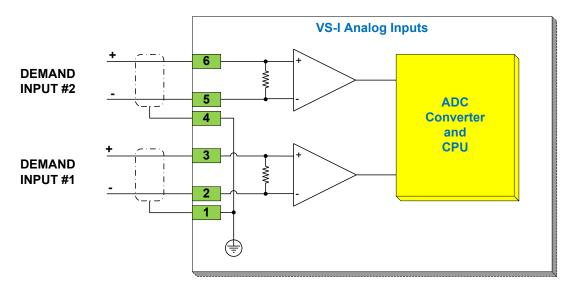
Figure 5-21. Analog Input Connections
