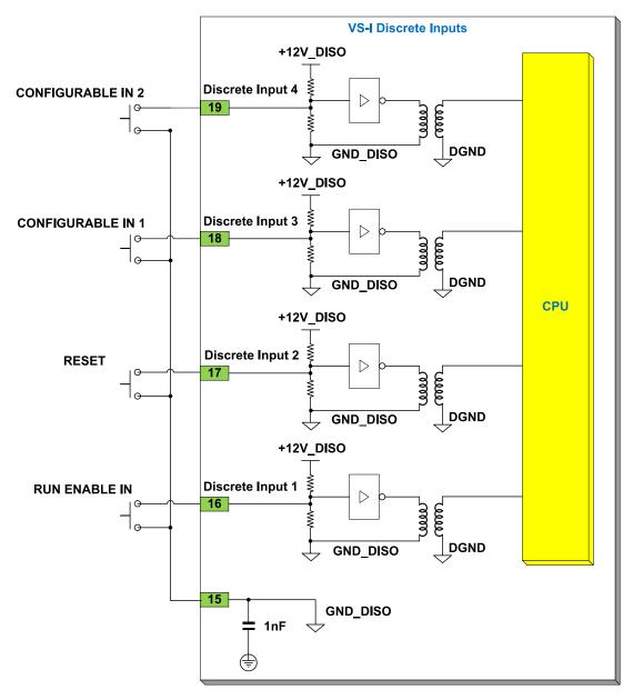
Figure 5-29. Discrete Inputs Connections
