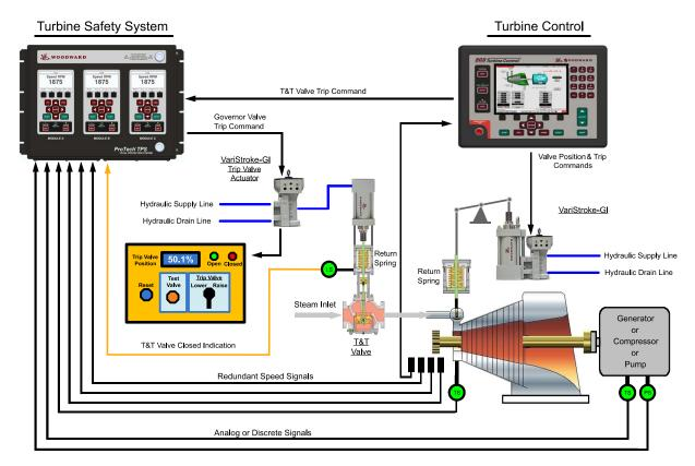
Figure 4-1. Example VS-T&TV Actuator Application
