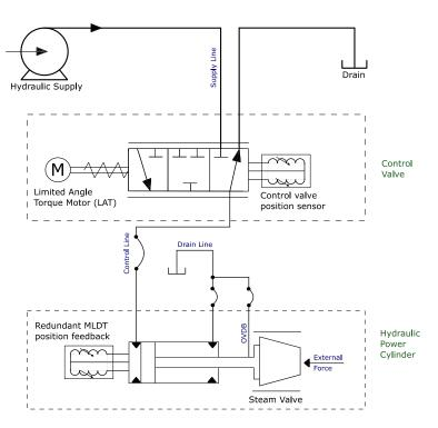
Figure 2-9. VS-GI Remote Hydraulic Schematic – Fail Retract with Externally Provided Closing Load
