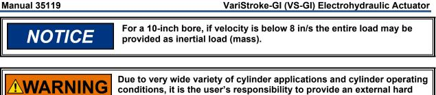
stop to prevent damage to the VariStroke actuator due to impact.
