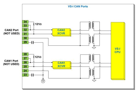
Figure 5-31. CAN Ports Connections
