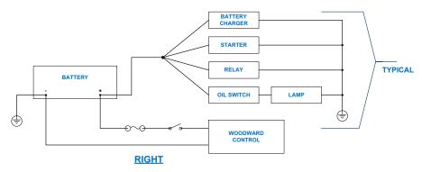
Figure 5-17. Correct Wiring to Power Supply Input
