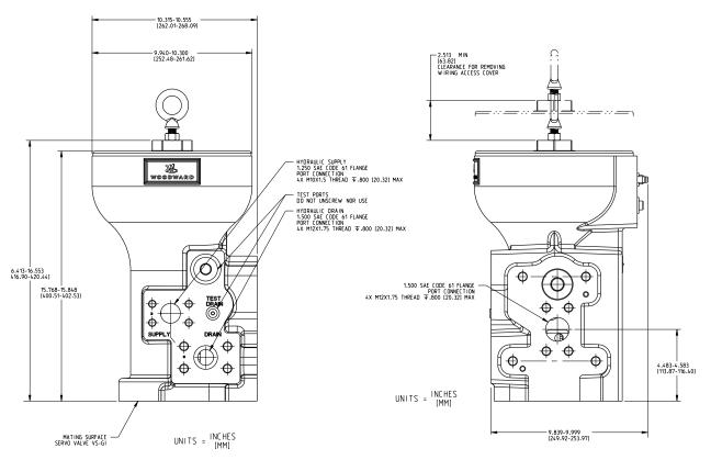
Figure 5-3a. VS-GI Remote Servo - Bolting Pattern and Installation Features - Side View
