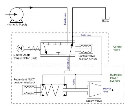
Figure 2-8. VS-GI Integrated Hydraulic Schematic - Fail Extend with Spring
