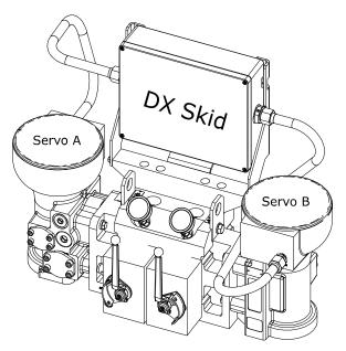
Figure 1-6. VS-DX Duplex Hydraulic Servo Skid
