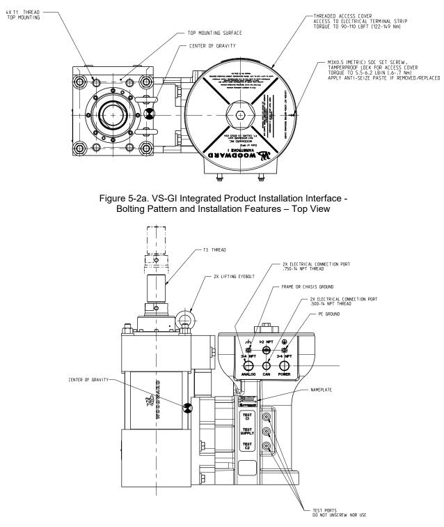
Figure 5-2b. VS-GI Integrated Product Installation Interface -Bolting Pattern and Installation Features – Side View
