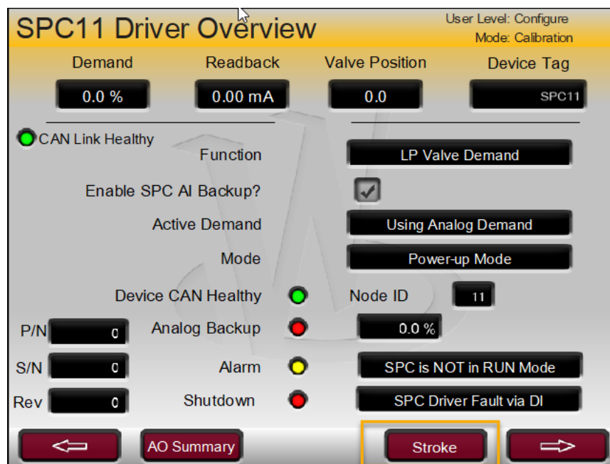
Figure 17-20. Access to Stroking of SPC Demand (Calibration Mode)
