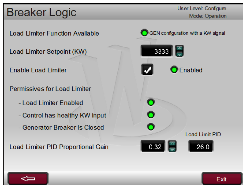
Figure 17-23. Service/Breaker Logic – Load Limiter Function Settings
