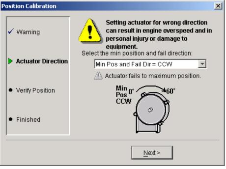
Figure 4-19. Service Tool—Manual Position Calibration
