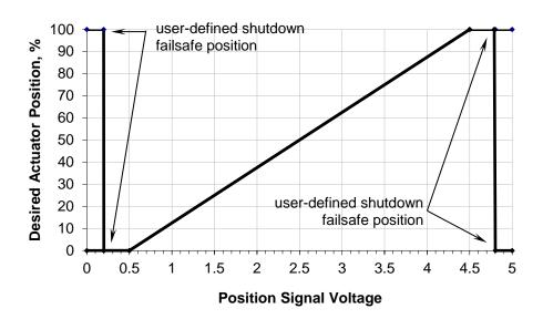
Figure 2-6. Analog 0–5 V Linear Demand to Position
