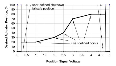
Figure 2-7. Analog 0-5 V Non-Linear Demand to Position
