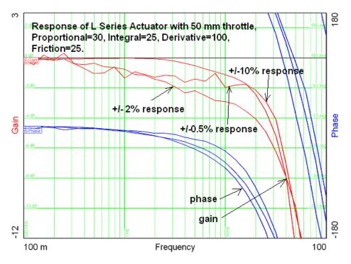
Figure 5-1. Bode Plot of L-Series Response
