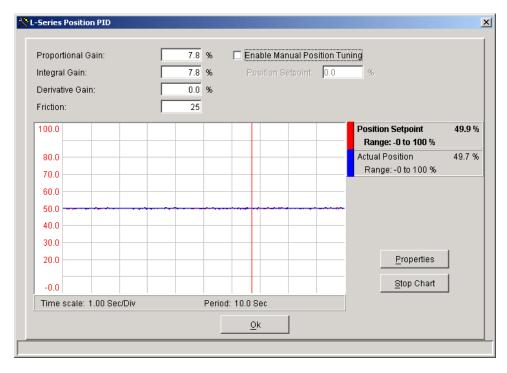
Figure 4-16. Service Tool—PID Tuning Window
