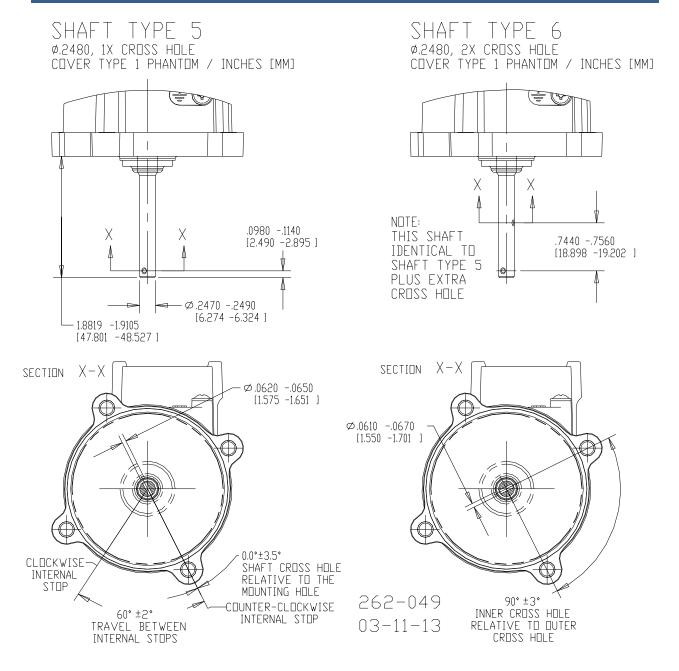
Figure 3-3c. L-Series Shaft Types
