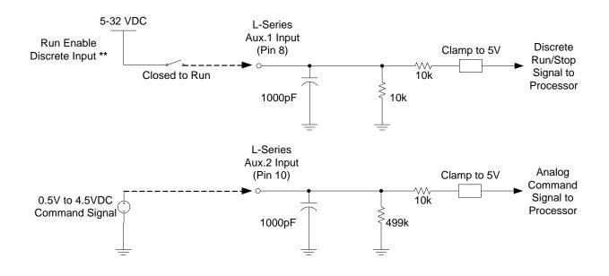
\*\* if optional external Run Enable is chosen during L-Series configuration, Aux. 1 can be used to enable or disable the actuator output shaft torque.
