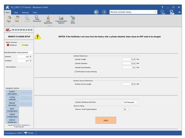
Figure 6-2. Remote Cylinder Setup Screen
