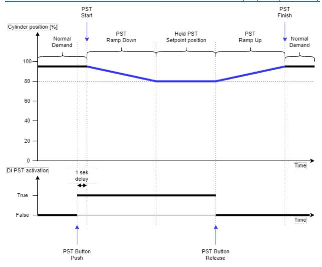
Figure 5-11. Partial Stroke Test
