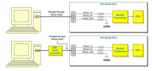
Figure 2-1. Service Port Connections
