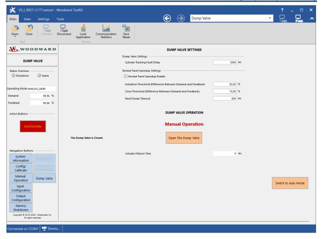
Figure 5-17. Dump Valve Manual Operation
