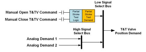
Figure 5-9e. VS T&T Valve Demand - Dual Analog High Signal Select
