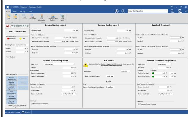
Figure 5-2. Input Configuration Screen
