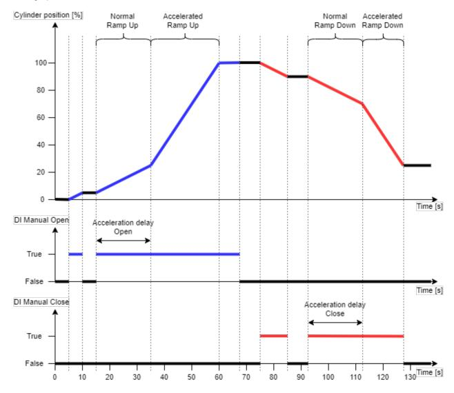
Figure 5-10. Trip and Throttle Manual Demand Operation
