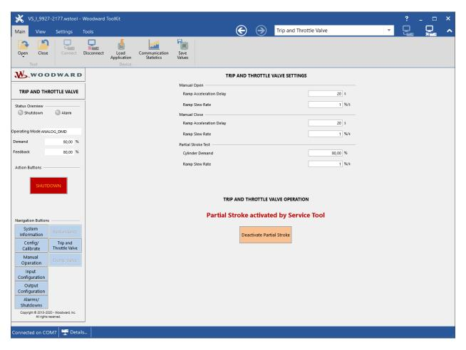
Figure 5-12. Partial Stroke Test by Service Tool Command
