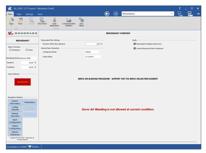
Figure 5-19. Redundancy Configuration Screen
