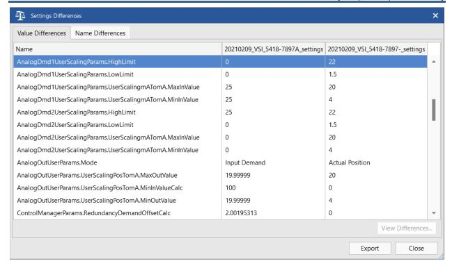
Figure 10-12. Setting Files Comparison - Value Differences
