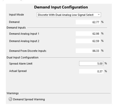
Figure 5-3. Demand Input Configuration for Trip and Throttle Valve Example
