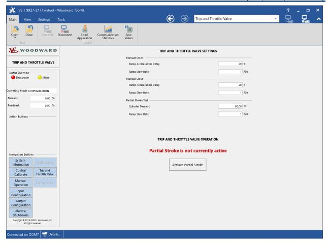
Figure 5-8. Trip and Throttle Screen
