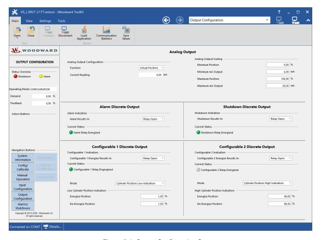
Figure 5-4. Output Configuration Screen
