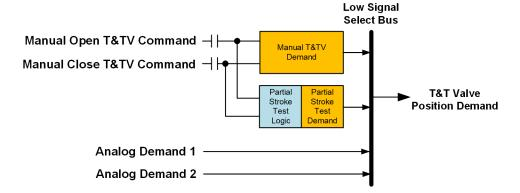
Figure 5-9h. VS T&T Valve Demand - Discrete with Dual Analog Low Signal Select
