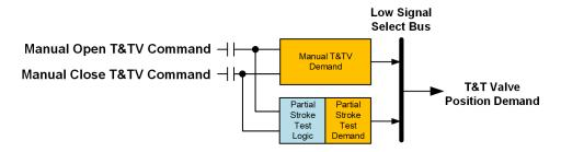
Figure 5-9f. VS T&T Valve Demand - Discrete Only
