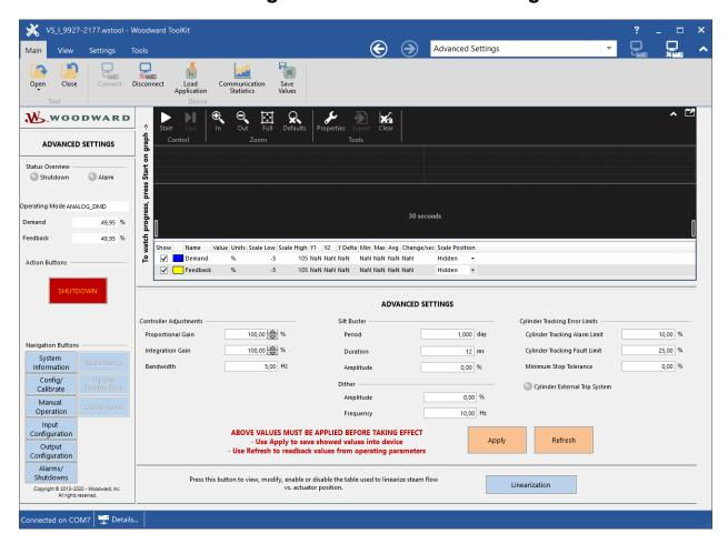
Figure 5-6. Advanced Settings Screen - On-Line Parameter Changes
