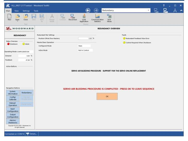
Figure 7-3. Servo Air Bleeding Completed
