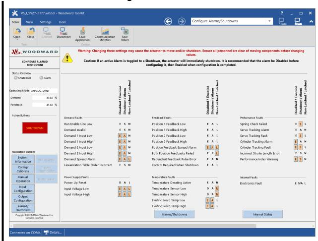
Figure 5-22. Alarms and Shutdowns Configuration Screen
