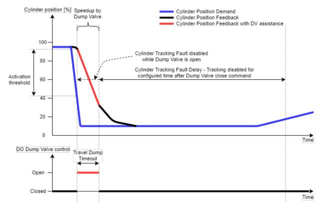
Figure 5-16. Dump Valve Speedup Operation with Timeout
