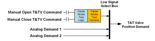
Figure 5-9d. VS T&T Valve Demand - Dual Analog Low Signal Select
