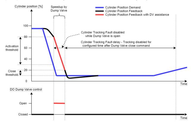
Figure 5-15. Dump Valve Speedup Operation
