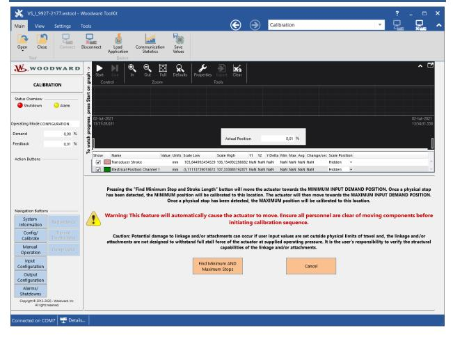
Figure 6-6. Calibration Find Minimum and Maximum Stops Screen
