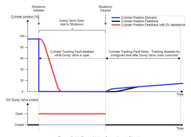
Figure 5-14. Dump Valve Operation at Shutdown
