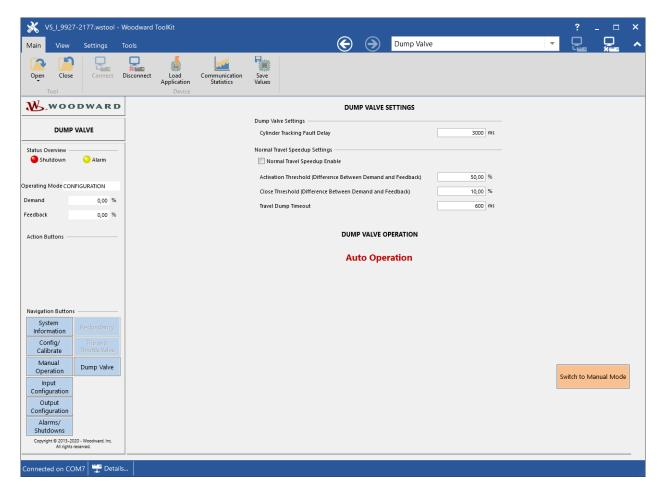
Figure 5-13. Dump Valve Settings Screen
