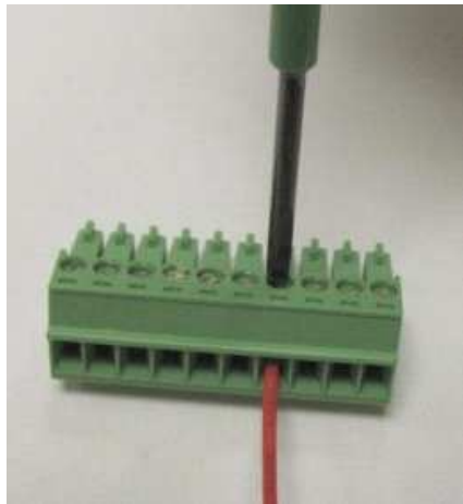
Figure 2-1. Screw Connection Terminal Block Used on A5200 SmartCore Board
