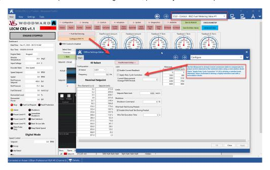
Figure 3-16. Fuel Control Valve Configuration
