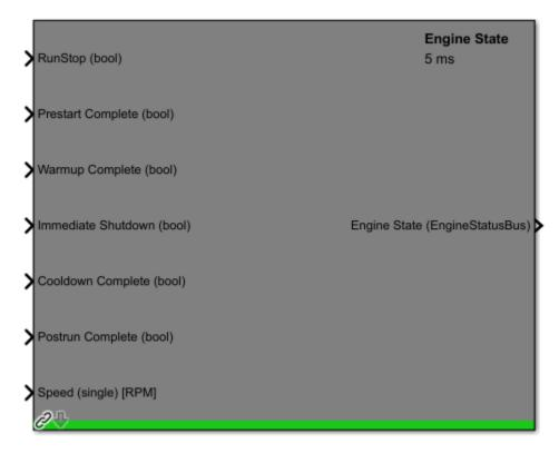
Figure 8-3. LESP Model Reference 'Functions – Engine State' Block
