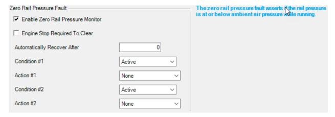
Figure 2-36. Zero Rail Pressure Monitor Configurations
