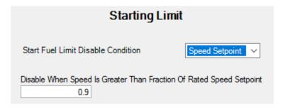
Figure 5-30. Speed Setpoint Dependent Switch Off
