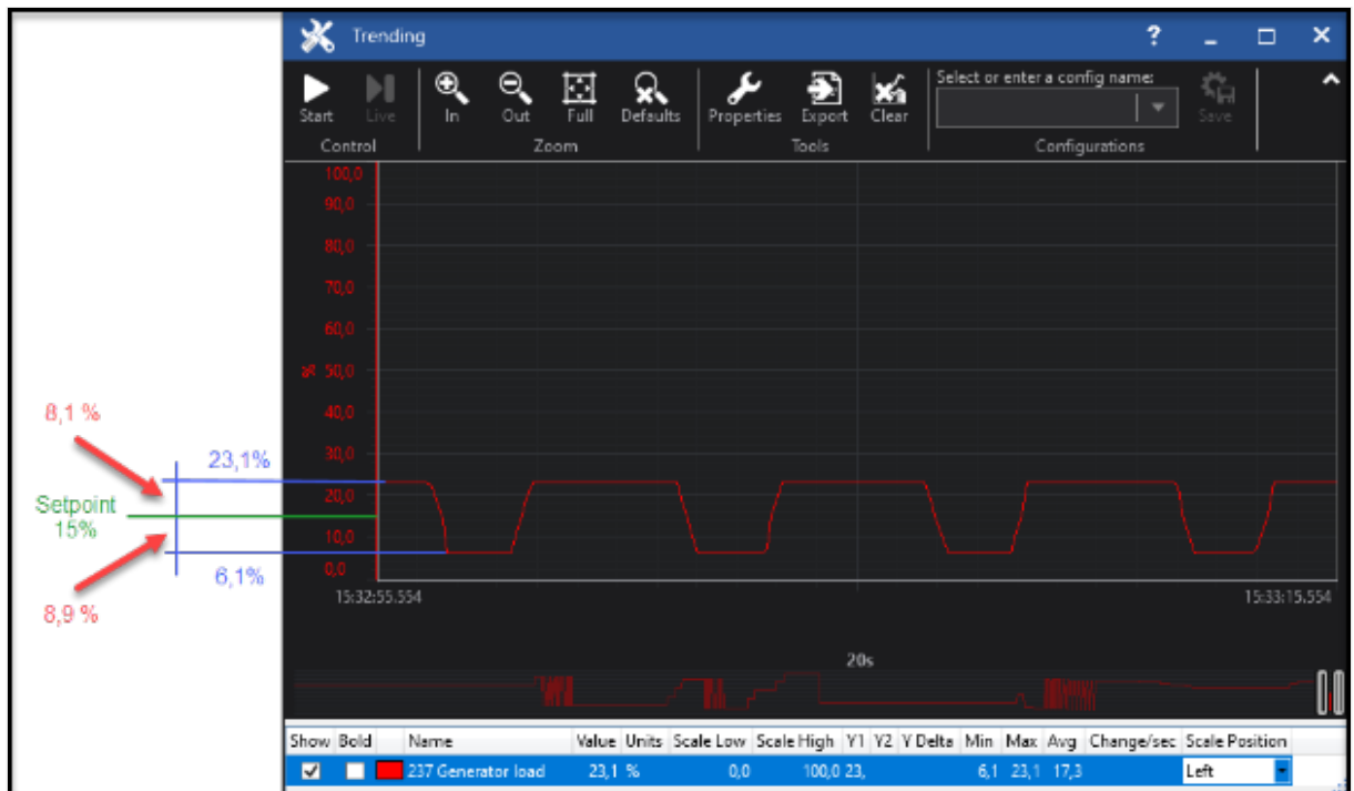
Fig. 181: The ToolKit trend shows the oscillating of a load step. The example shows that the dead band must be minimum 8.9\% + 1\% = 9.9\% that the oscillating is prevented.
