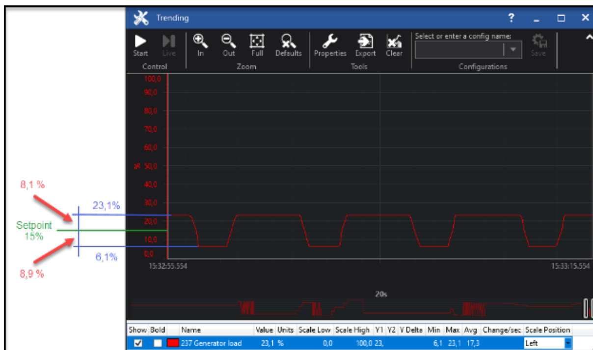
Fig. 191: The ToolKit trend shows the oscillating of a load step. The example shows that the dead band must be minimum 8.9\% + 1\% = 9.9\% that the oscillating is prevented.
