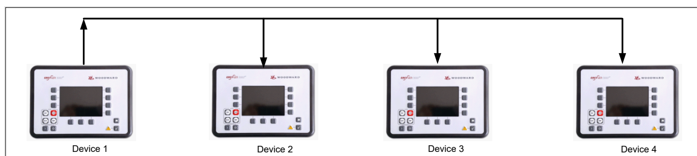
Fig. 271: Device 1 sends data to device 2, 3 and 4
