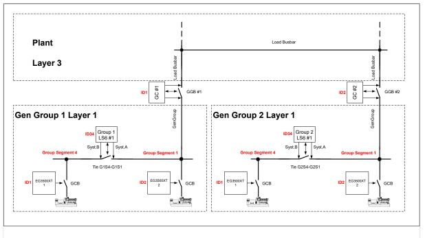
*Fig. 100: Drawing of an application with 2 Groups containing 2 Gensets connected over Tie-breaker*
