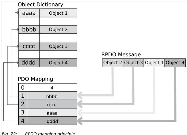
Fig. 72: RPDO mapping principle
