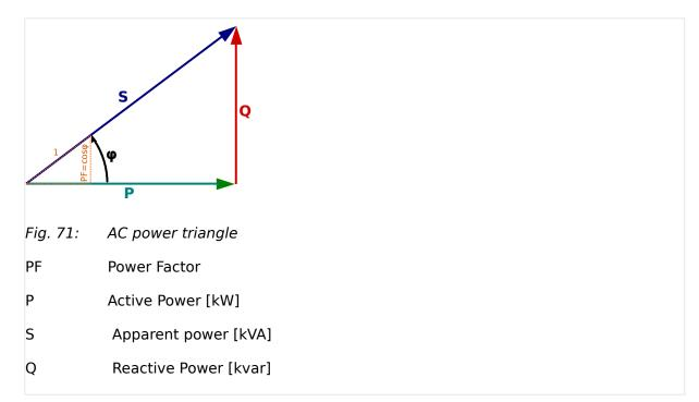
The AC power triangle illustrates the dependencies between active power, apparent power, reactive power and power factor.
