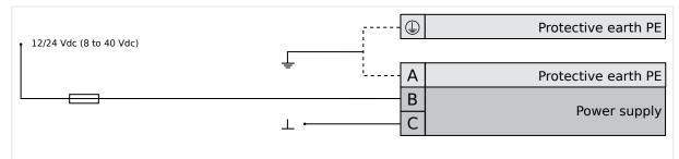
Fig. 12: Power supply - wiring
