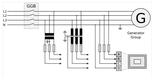
*Fig. 14: Voltage measuring - generator group - wiring*
