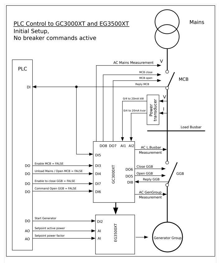
Fig. 77: Initial Setup controlling breaker via the GC-3400XT-P1 in conjunction with a PLC
