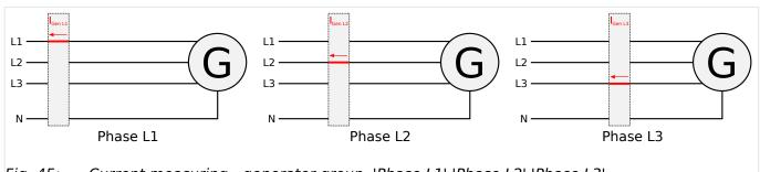
*Fig. 45: Current measuring - generator group, 'Phase L1' 'Phase L2' 'Phase L3'*
