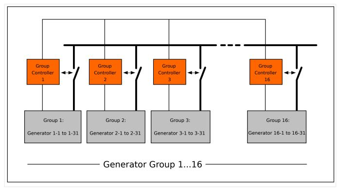
Schematic: The Group Controllers and its generators
