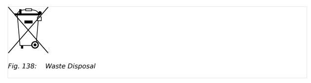
This device contains a battery, and therefore it is labeled with the symbol shown beside according to the EU Directive 2006/66/EC.
