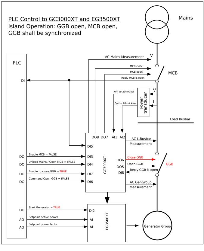
*Fig.* 79: Synchronization of the GGB initiated by PLC.
