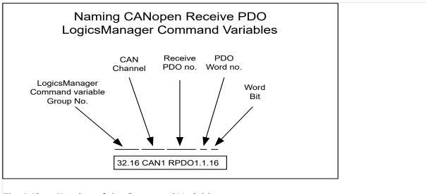
Fig. 142: Naming of the Command Variables.
