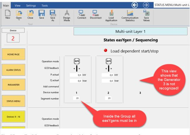
*Fig.* 87: ToolKit screen: Example with a faulty generator group 3
