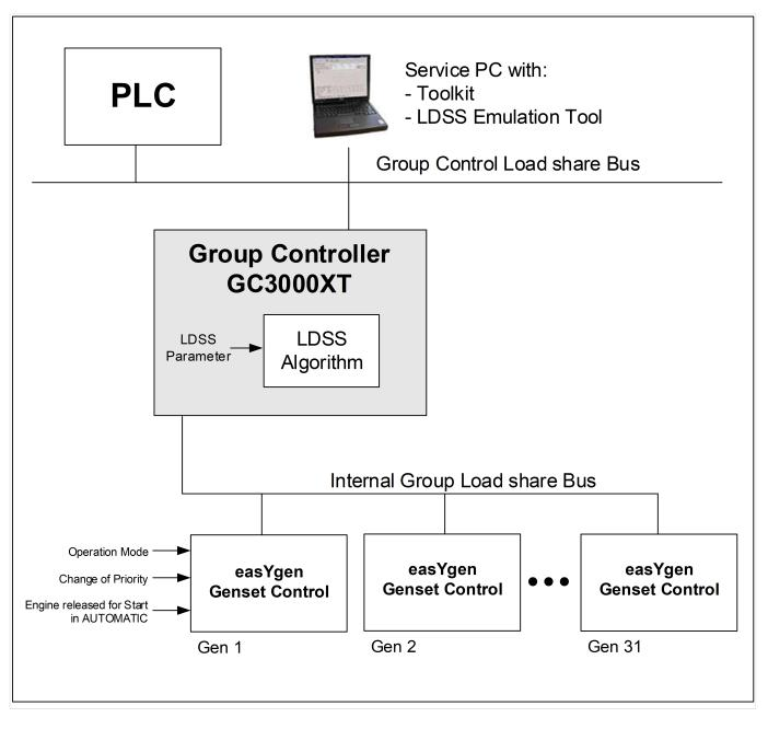
Schematic: The Group Controller with its group and its setting
