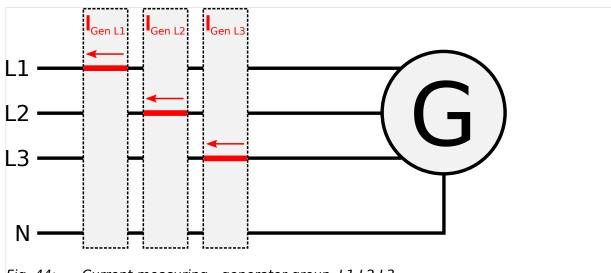
*Fig. 44: Current measuring - generator group, L1 L2 L3*
