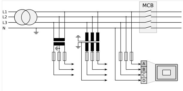
*Fig. 27: Voltage measuring - mains - wiring*
