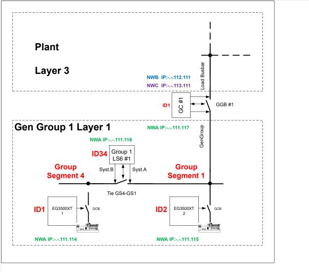
*Fig. 101:* The Group LS-6XT is connected to the group communication bus
