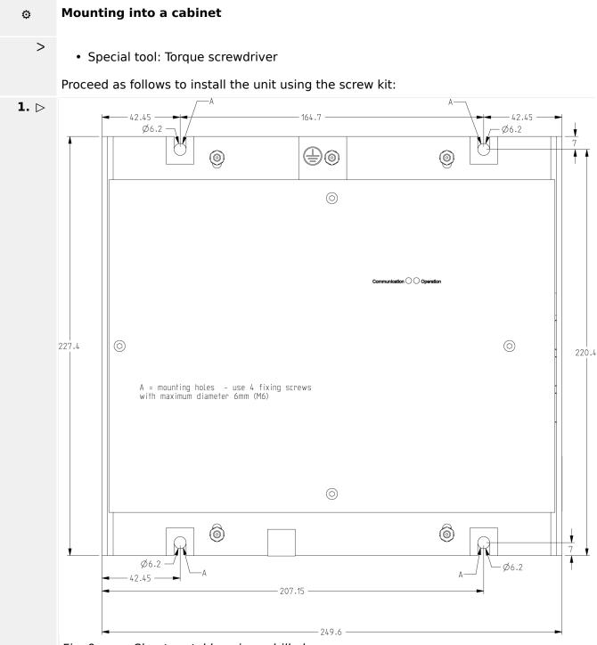
*Fig. 9: Sheet metal housing - drill plan*
