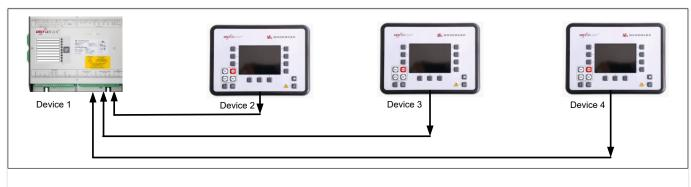
Fig. 122: Device 1 receives data from device 2, 3 and 4
