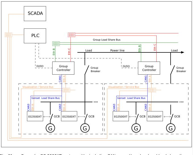
*Fig. 61: Example: GC-3000XT system with single line CAN on easYgen level and load share line redundancy on GC level*
