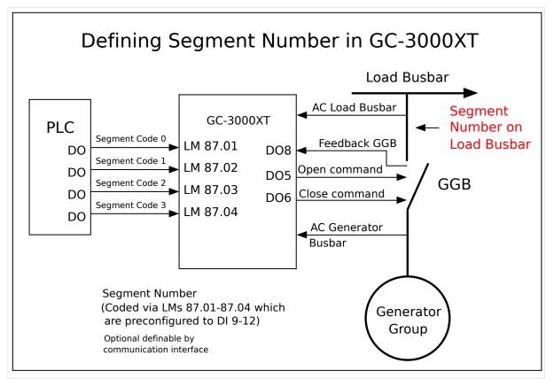
The Segment number handling defines the Load Busbar Segment.
