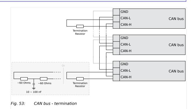
For very critical EMC conditions (many noise sources with high noise levels) and for high transmission rates we recommend to use the 'Split termination concept' as shown.
