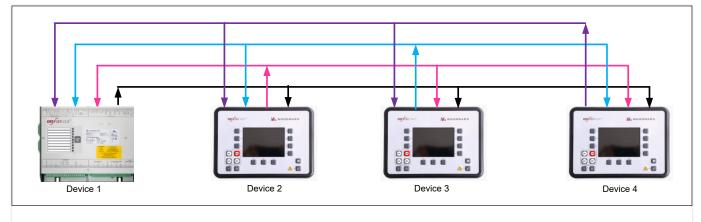
*Fig. 123: Each Device receives data from the other devices*
