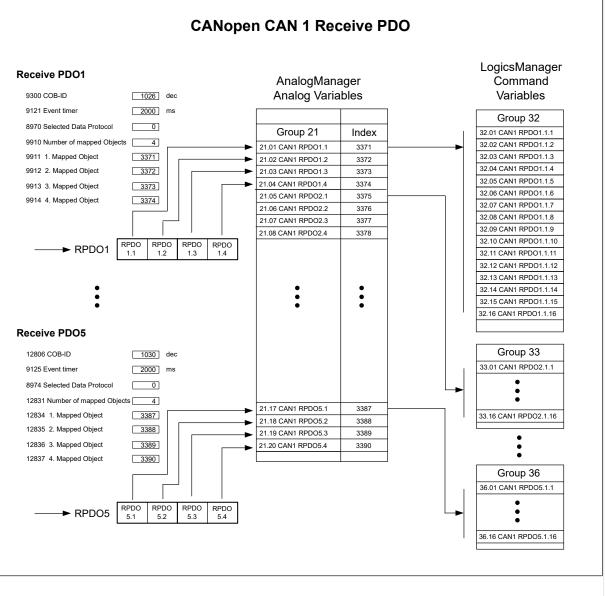
*Fig. 143:* Example of a CAN 1 RPDO configuration for interconnectivity.
