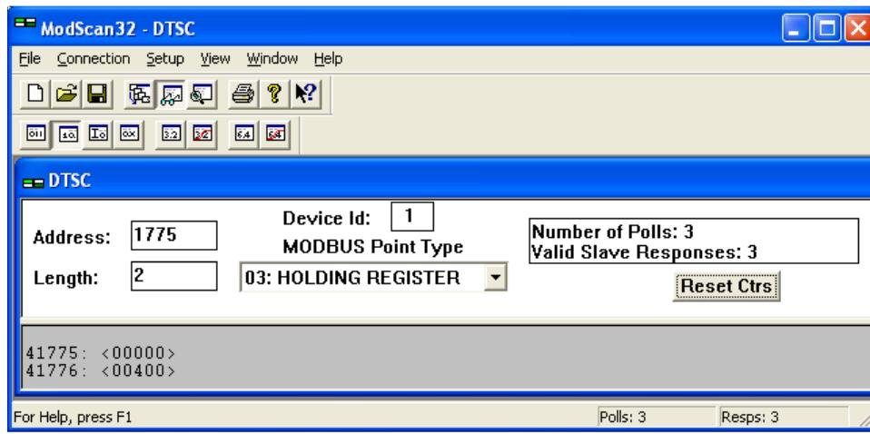
Figure 3-4: Modbus - configuration example 2
