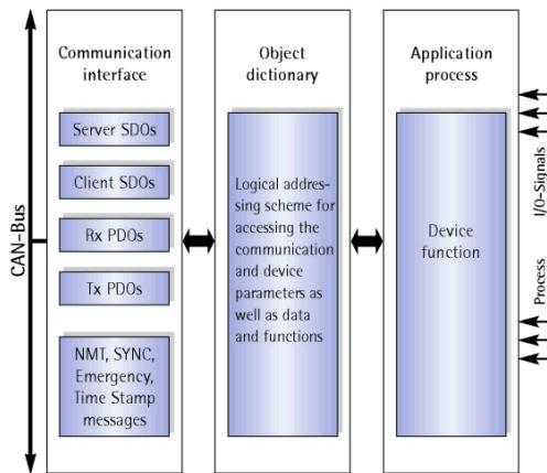
The CANopen family profile defines a standardized application for distributed industrial automation systems based on CAN as well as the communication standard CAN CAL. CANopen is a standard of CAN-in-Automation (CiA) that after its release, found a broad acceptance, especially in Europe. CANopen can be considered the leading standard for CAN based industrial and embedded system solutions.
