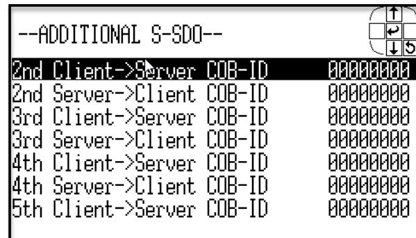
Figure 4-12: Display screen - configure Server SDOs
