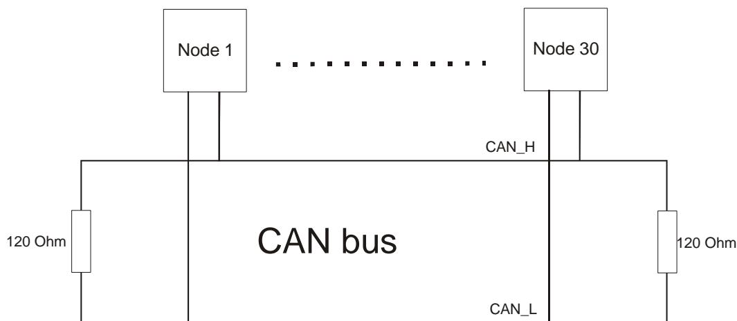
Figure 1-4: Interface - The CAN bus loop
