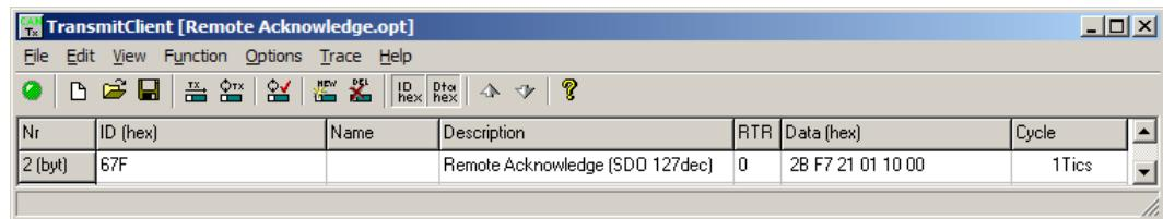
Figure 4-13: CANopen request data for additional Server SDO
