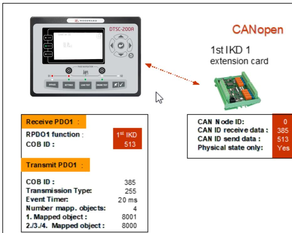
Figure 4-4: CANopen Interface – Adjustments for external devices
