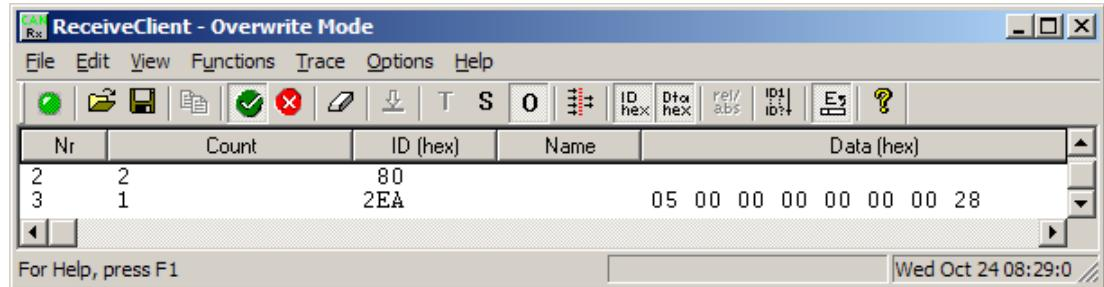
Figure 4-17: Cyclical sending of data - reply
