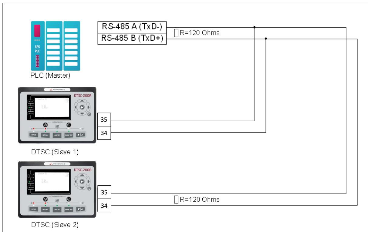
Figure 1-2: Interface overview - serial interface Modbus half-duplex
