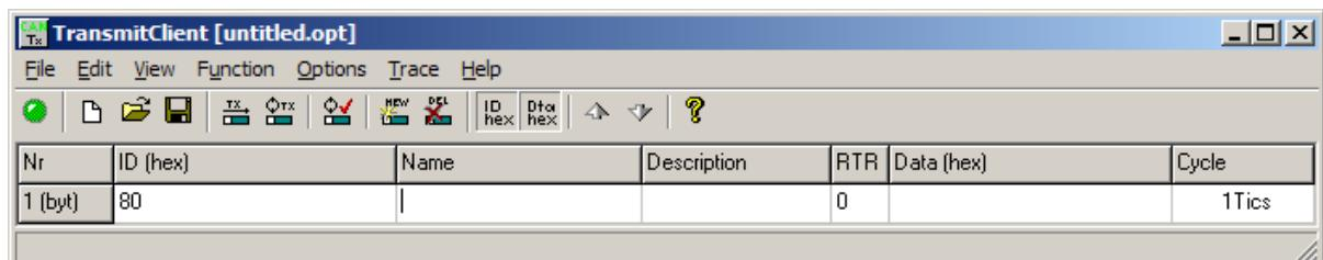
Figure 4-16: Cyclical sending of data - Sync Message request
