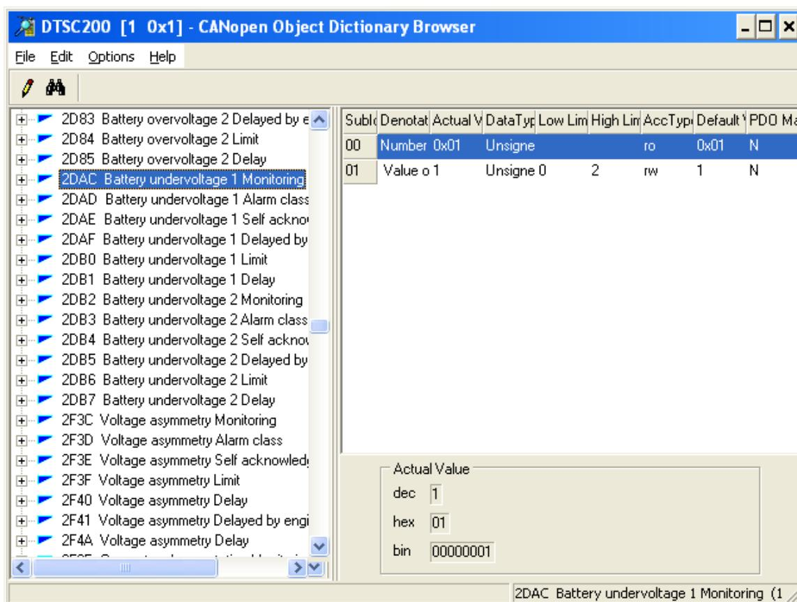
Figure 4-2: CANopen interface - CANopen configuration software
