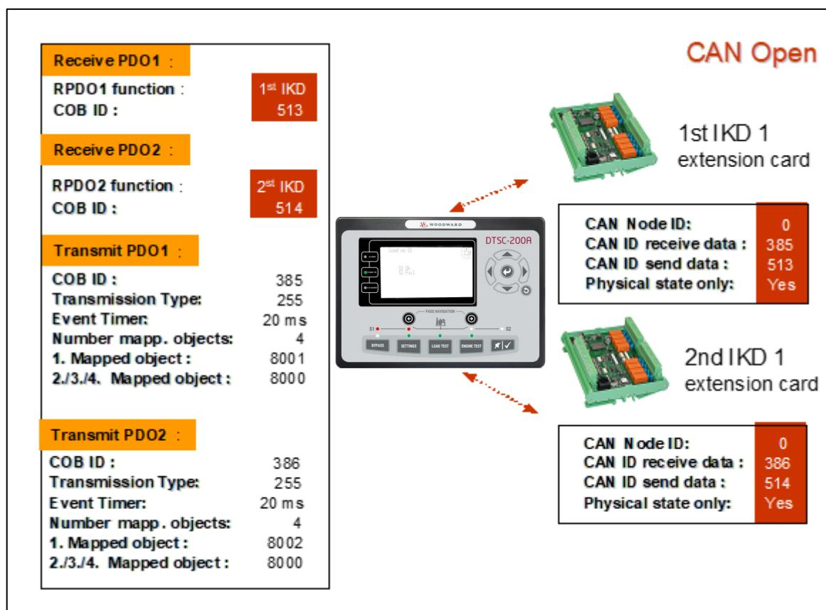
Figure 4-5: CANopen interface - expansion with two IKD 1
