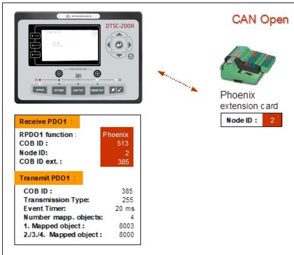
Figure 4-6: CANopen interface - expansion with Phoenix terminal
