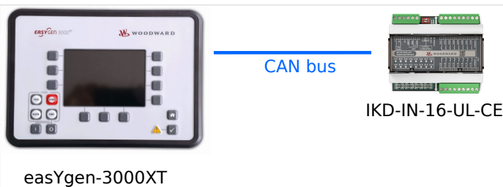
Fig. 9: easYgen-3000XT and one IKD-IN-16(UL, CE)
