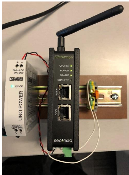
Figure 2-1. Remote Access Unit (RA_Unit)
