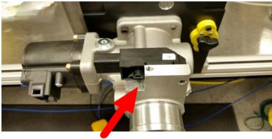
Press sensor into EFR housing
