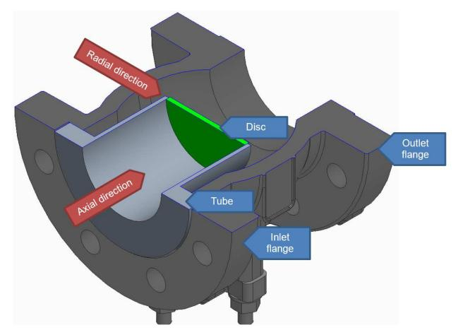
Figure 1. Partial Section of RVP-200 with housing orientation and valve trim identified
