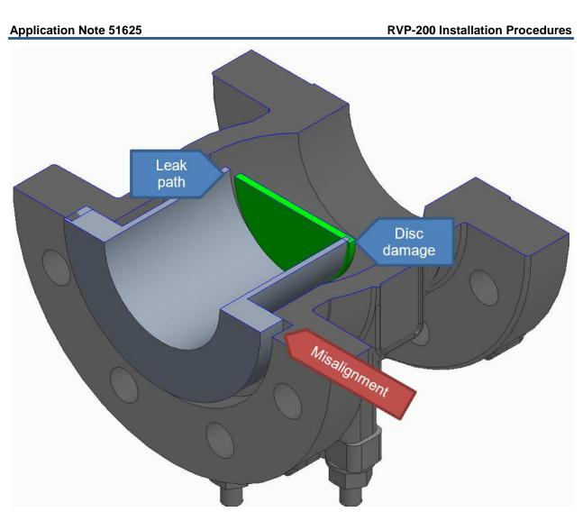
Figure 2. Partial section showing exaggerated misalignment and resulting performance degradation
