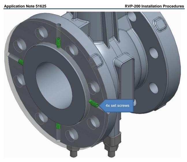
Figure 3. Partially transparent view of updated design showing set screws that provide greater alignment stability
