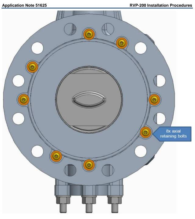
Figure 4. Six-inch valve with additional axial retaining bolts
