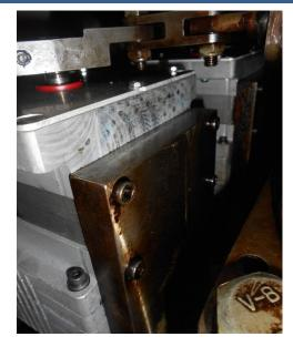
Figure 2-3. Dismantling Actuator from Mounting Plate
