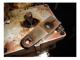
Figure 2-2. Removing Actuator Terminal Lever from Actuator Output Shaft
