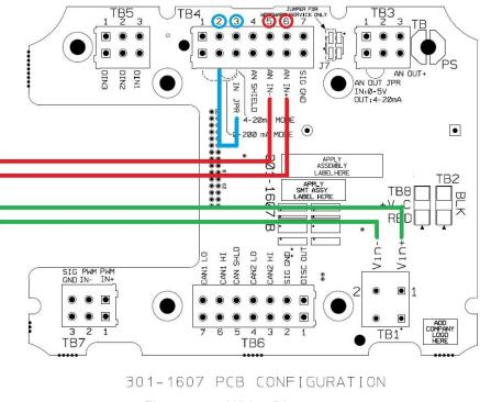
Figure 2-10. Wiring Diagram
