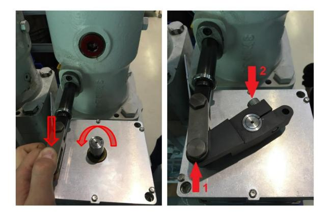
Figure 2-11. Linkage Adjustment
