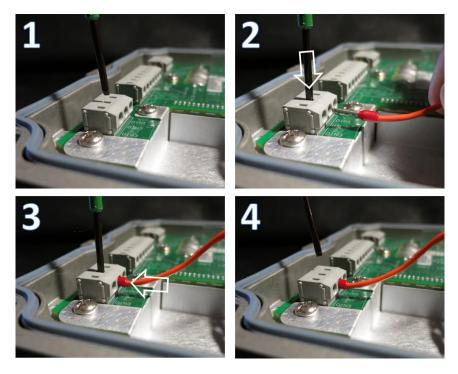
Figure 2-7. I/O Terminal Block Ferrule Installation
