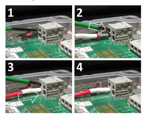
Figure 2-8. Power Terminal Block Ferrule Installation
