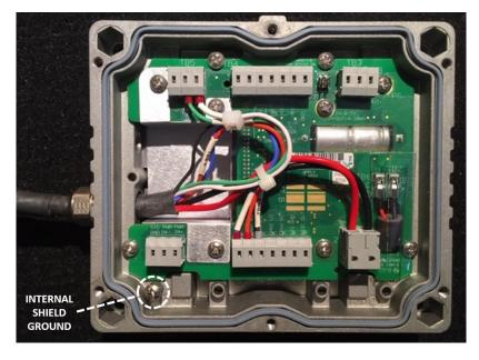
Figure 2-9. Example of Internal Wiring of ProAct Gen3 FLEX
