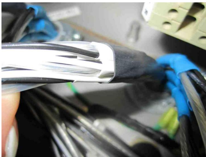
Figure 3-6. GS40 Twisted Pair and Final Wiring Prep
