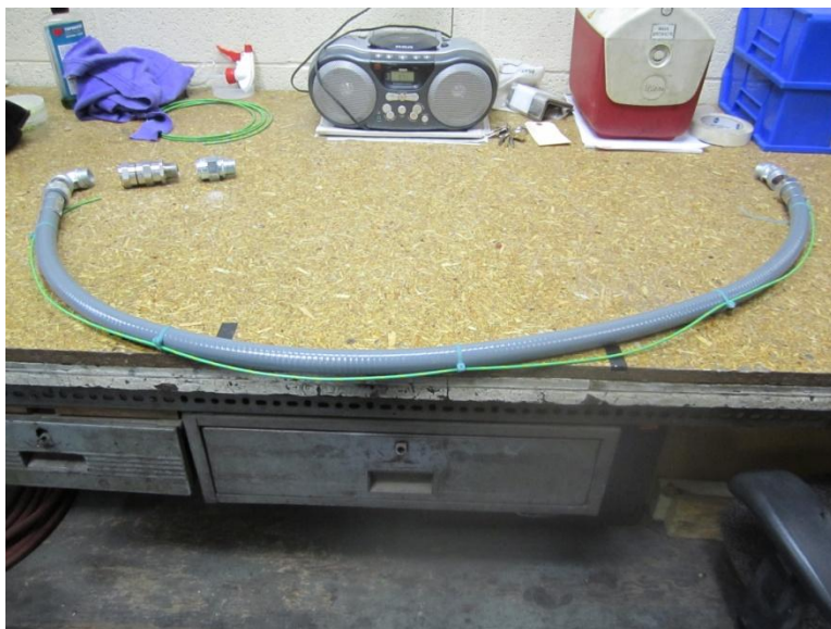
Figure 3-2. Tefzel Grounding Wiring Installation
