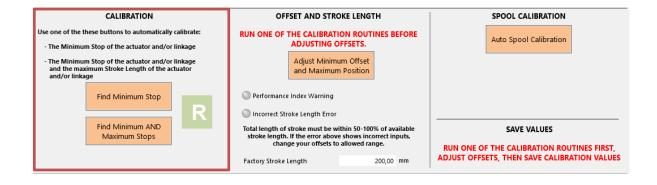
Figure 2-23. Cylinder Calibration
