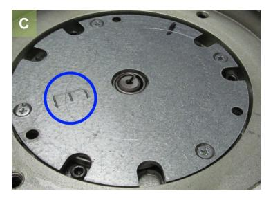
Figure 5-1. Remove Cover Screws and Note Letter on Spring Assembly Face
