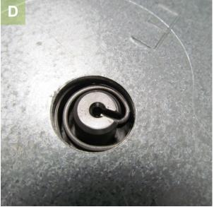
Figure 5-6. Verify Spring Orientation and Install Spring Assembly
