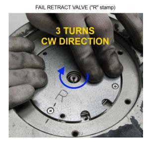
Figure 5-7. Mark Return Spring and Housing, Rotating Spring
