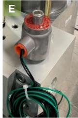
Figure 7-2. Install Solenoid with O-rings.
