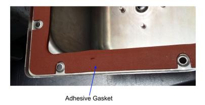
Figure 2-10. Gasket and Shaft Seal Replacement
