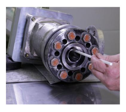
Figure 3-4. Proper Obstruction Removal
