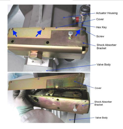
Figure 2-1. Cover and Attachment Hardware
