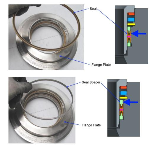
Figure 3-8. Second Seal and Spacer Installation
