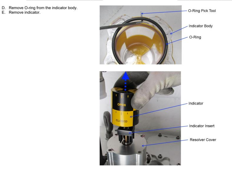
Figure 5-2. O-ring and Indicator Body Removal
