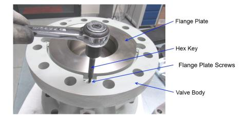
Figure 3-12. Screw Installation
