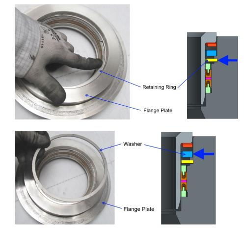
Figure 3-9. Retaining Ring and Washer Installation
