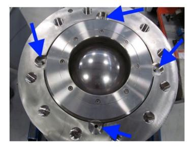
Figure 4-1. Flange Plate Assembly Removal
