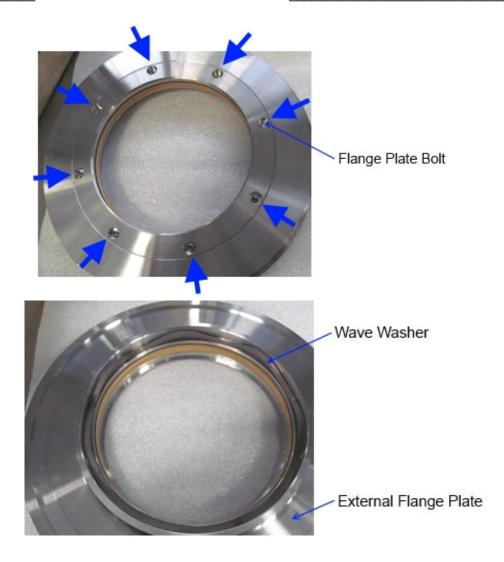
Figure 4-7. Install Flange Plate and Wave Washer
