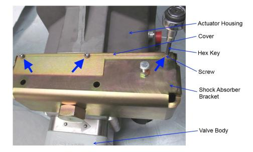
Figure 2-5. Install Cover Screws
