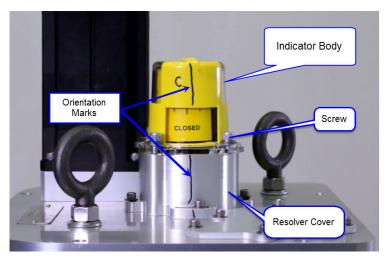
Figure 5-8. Install the Indicator Body
