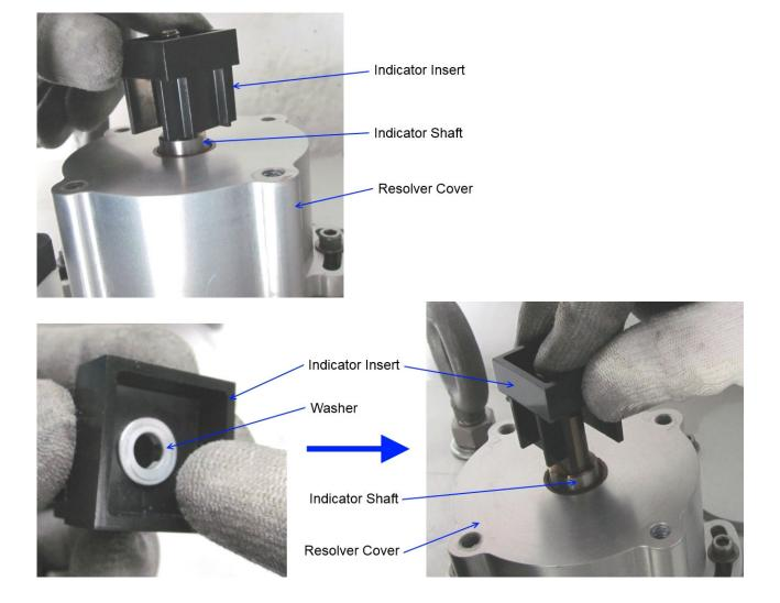
Figure 5-6. Install Indicator Insert
