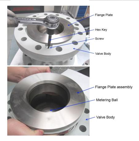
Figure 3-1. Flange Plate Assembly Removal
