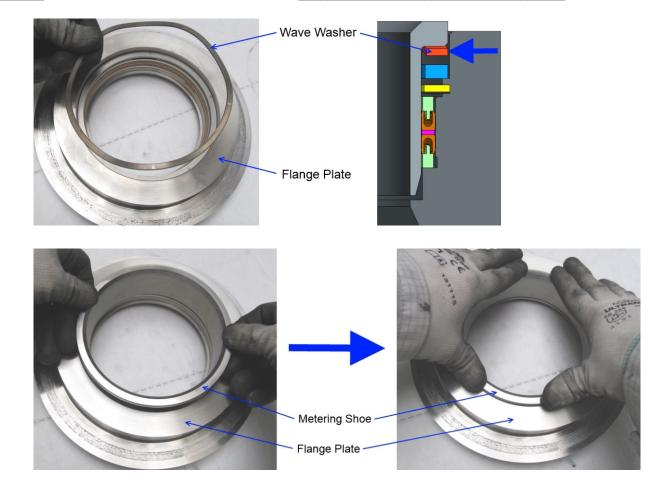
Figure 3-10. Wave Washer and Metering Shoe Installation
