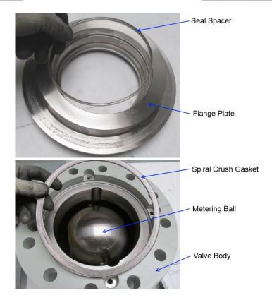
Figure 3-5. Second Spacer Removal
