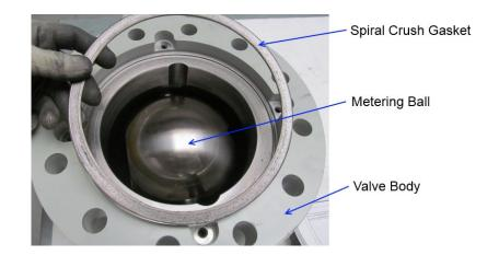
Figure 4-5. Gasket Removal
