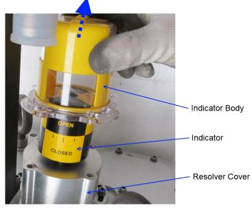
Figure 5-1. Indicator Body Removal
