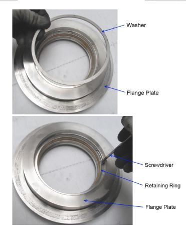
Figure 3-3. Washer and Retaining Ring Removal
