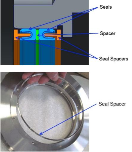
Figure 4-4. Spacer and Seal Removal
