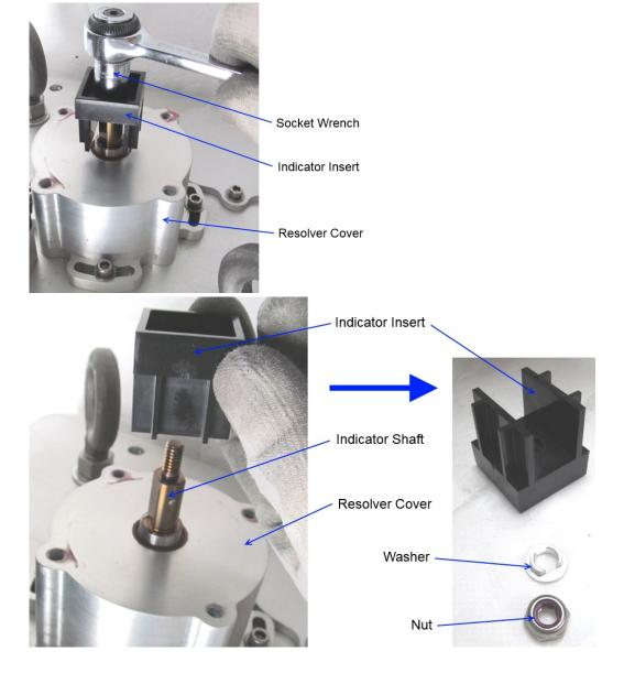
Figure 5-3. Indicator Insert Removal
