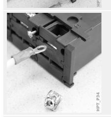
Every terminal consists of a screw with a non-losable metal contact. Screw (plus contact) can be unscrewed completely.
