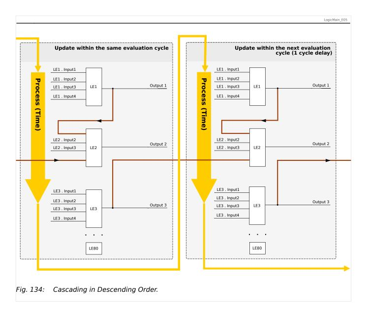
In the example shown in  $\square$  Fig. 134 above, "Logic Equation **2**" uses the output states of two other equations, "Logic Equation **1**" and "Logic Equation **3**". The result of "Logic Equation **1**" is used in ascending order and has therefore been evaluated within the same process cycle. The result of "Logic Equation **3**" is used in descending order and has therefore been evaluated in the previous process cycle.
