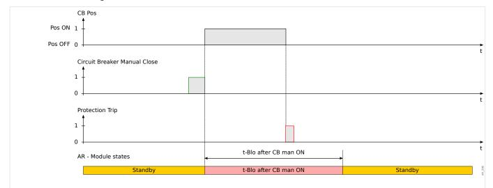
*Fig. 106: Protection Trip while Manual Close Blocking time is Timing.*
