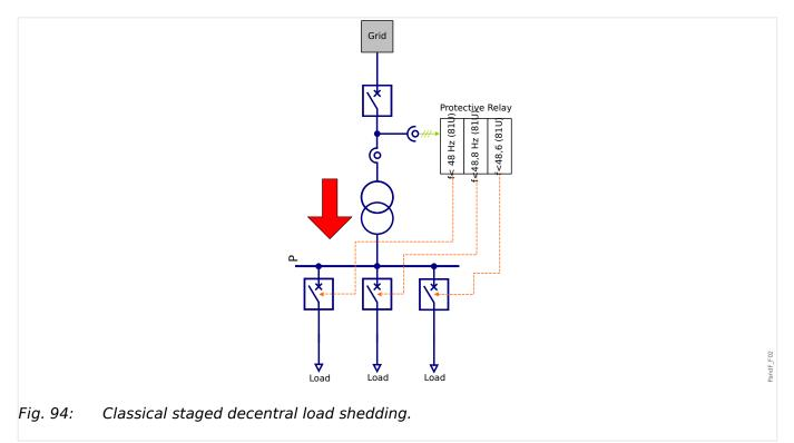
A classical decentralized load shedding can be done by deactivating the power flow direction detection.
