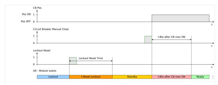
*Fig. 107: AR Lockout Reset Logic in case lockout Reset coming before manual breaker closed.*
