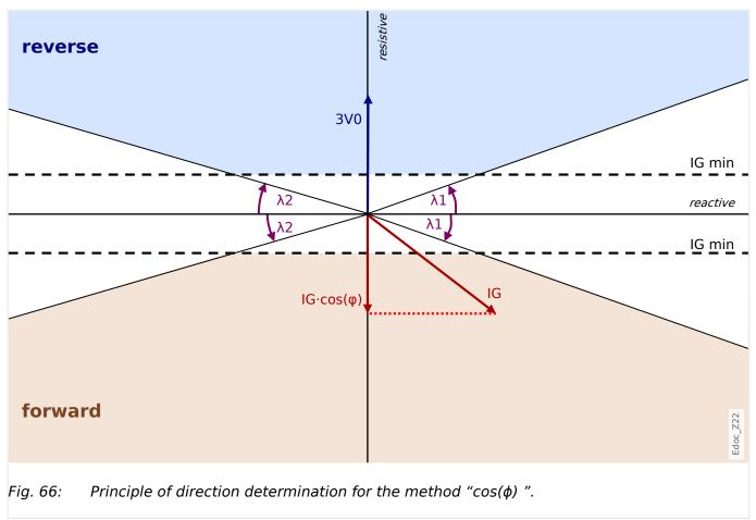
4.1.2.2.3 Wattmetric / Sensitive Ground (Earth) Fault Direction
