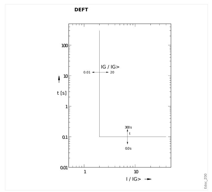
Trip delay for IG > IG>, settable via [Protection Para / Set 1...4 / I-Prot / IG[x]] »t«. The reset delay for IG  $\leq$  IG> always equals 0 ("instantaneous").
