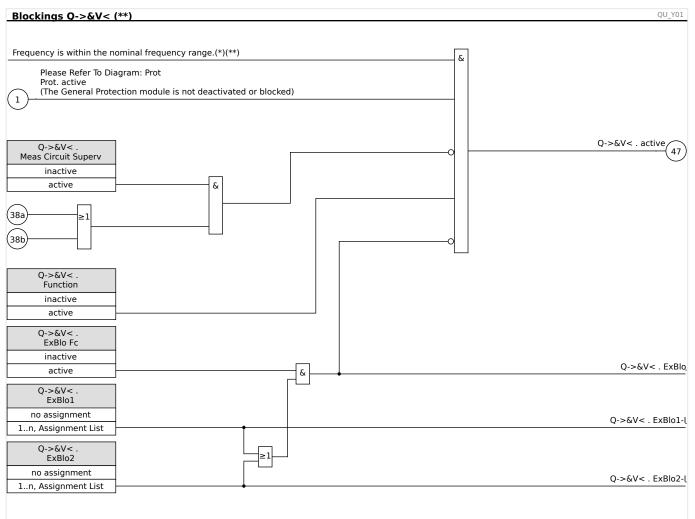
(\*) All protective elements will be blocked that are using fundamental or harmonics measured values, if the frequency leaves the nominal frequency range. Protective elements that are using RMS values will remain active. See chapter "Wide frequency range".
