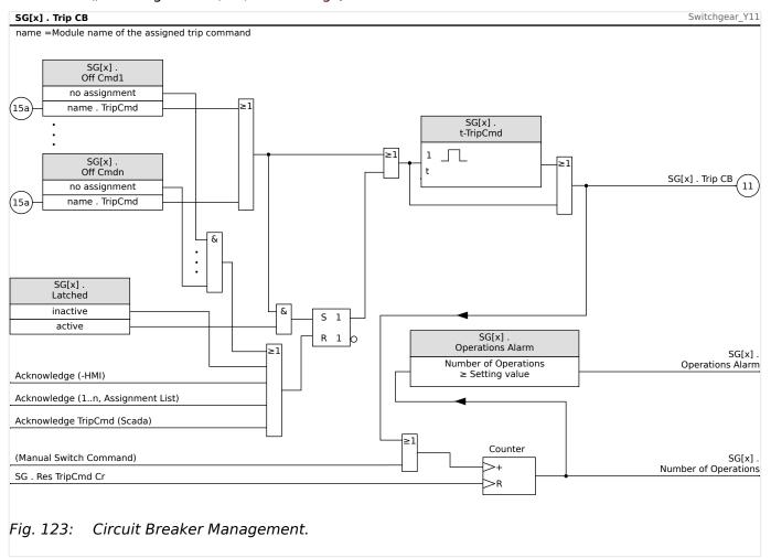
Note that in the diagram above, "SG[x]" represents "switchgear number x"; however, the exact designation is defined in the single-line file, see also  $\square$  "Single-Line Diagram".
