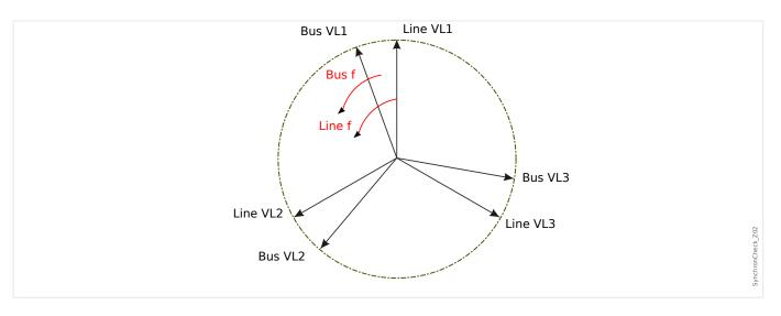
If the generator frequency fBus is not equal to the mains frequency fLine, it results in a slip frequency  $\Delta F = |fBus - fLine|$  between the two system frequencies.
