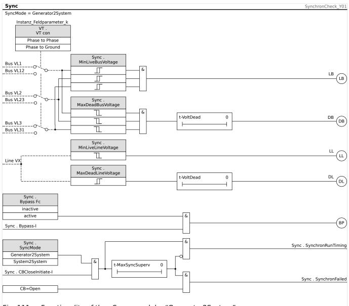
Fig. 111: Functionality of the »Sync« module, "Generator2System".
