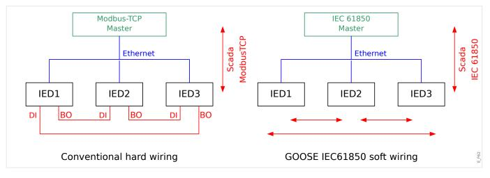
Commissioning steps for a conventional substation with modbus TCP environment:
