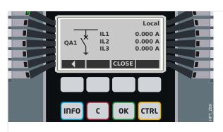
*Fig. 121: Control Page Example, with the "Circuit Breaker" in open position.*
