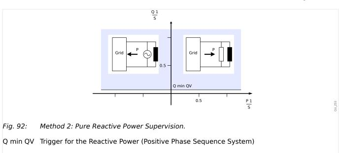
A minimum current supervision (I1) in the positive phase sequence system prevents a hyperfunction of the reactive-power supervision at lower power levels.
