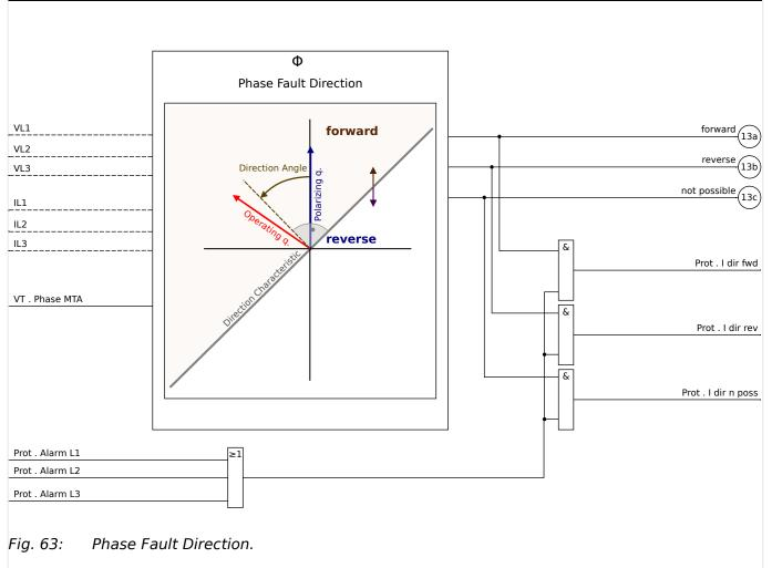
The MCA4 evaluates the angle between the current of the phase with the highest current (*Operating quantity*) and the phase-to-phase voltage of the other phases (Polarizing quantity). For three-phase-faults where the phase-to-phase-voltage is too low a voltage memory is used.
