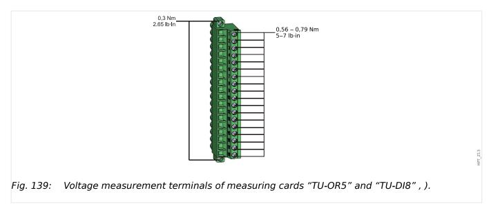
Voltage and Residual Voltage Measurement ("TU-OR5")
