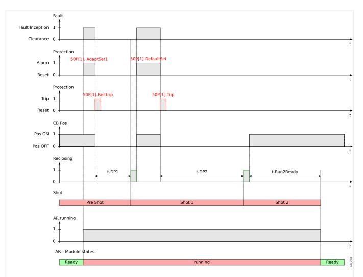
*Fig. 104:* Auto Reclosing timing diagram for **successful** 2-shot auto reclosing scheme with acceleration at pre-shot.
