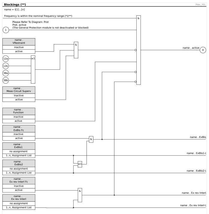
(\*) All protective elements will be blocked that are using fundamental or harmonics measured values, if the frequency leaves the nominal frequency range. Protective elements that are using RMS values will remain active. See chapter "Wide frequency range".
