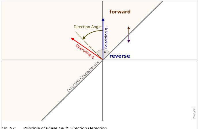
Principle of Phase Fault Direction Detection. Fig. 62:
