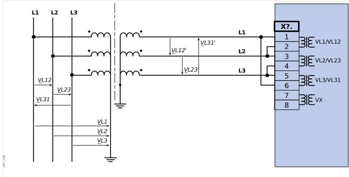
*Fig. 32:* Three-phase voltage measurement - wiring of the measurement inputs: "deltaconnection"
