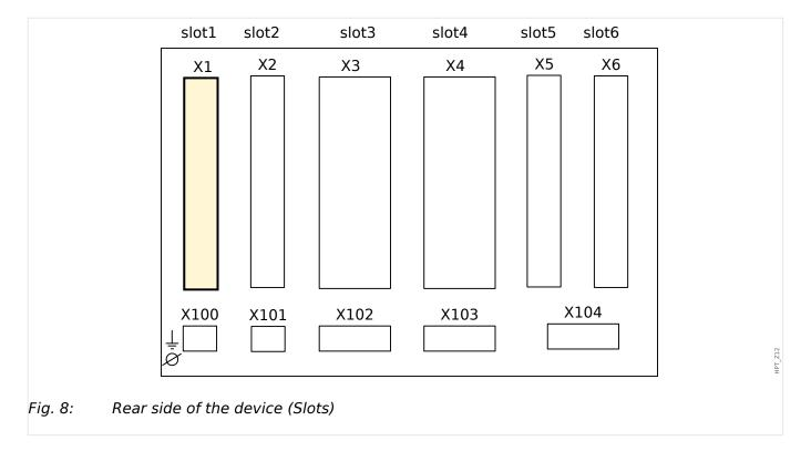
Power Supply Card with Digital Inputs
