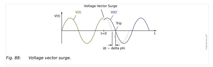
As shown in the voltage/time diagram the instantaneous value of the voltage jumps to another value and the phase position changes. This is called phase or vector surge.
