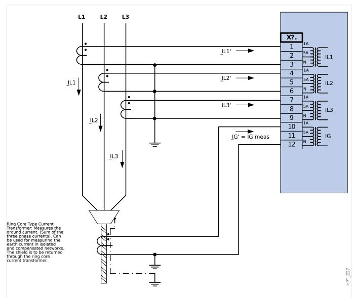
*Fig. 20:* Three phase current measurement; In secondary = 1 A. Earth-current measuring via cable-type current transformer ; IGnom secondary = 1 A.
