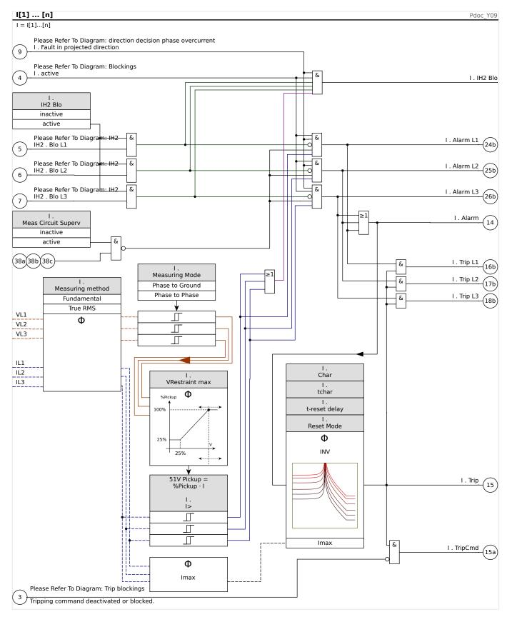
Remark: For the sake of simplicity, the diagram above does not show the fact that in case of [Field Para / VT] »VT con« = "Phase to Phase", the parameter »I[x]« . Measuring Mode is internally re-set to "Phase to Phase", independent of its configured value (see the Notice in  $\square$  Chapter 4.4.3).
