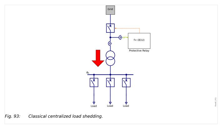
Classical load shedding of a sub-grid from a central connection point. The load shedding will be initiated by under frequency.
