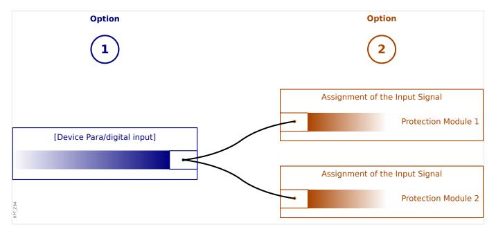
**Option 1:** Assigning a Digital Input onto one or mutliple modules.
