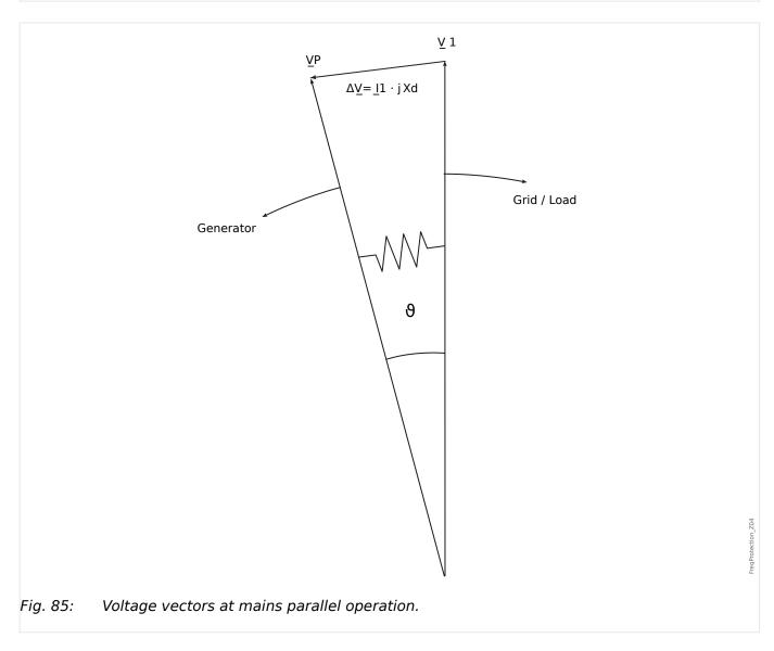
The rotor displacement angle between stator and rotor is dependent on the mechanical moving torque of the generator. The mechanical shaft power is balanced with the electrical fed mains power and, therefore the synchronous speed keeps constant.
