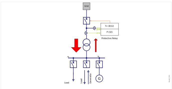
*Fig. 95: Centralized Under Frequency Load Shedding within grids with temporary power supply.*
