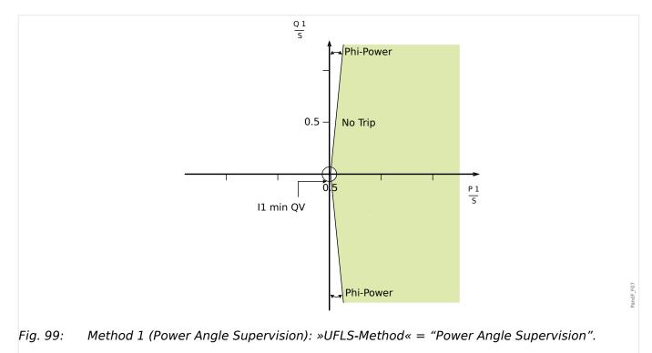
A load shedding during under frequency will be blocked, if the active power is within the area limited by the power angle.
