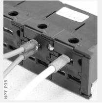
Remark: As long as the cable cross-sections are within the limits given in the Technical Data chapter ( > "12 Technical Data", > Tab. ) it is also possible to insert two rings into one terminal, as shown here. This is useful for setting up the neutral point connection.
