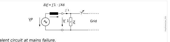
Equivalent circuit at mains failure. Fig. 86:
