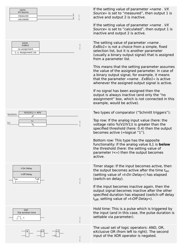
1 MCA4 – Directional Feeder Protection 1.1.2.2 Symbols in Function Diagrams
