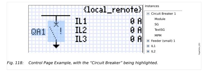
Although a switchgear always appears using a fixed representation in the *Page Editor*, with an exclamation mark "!" being placed aside, this symbol features several representations: one for the closed switchgear, one for the open switchgear, one for the intermediate and faulty positions.
