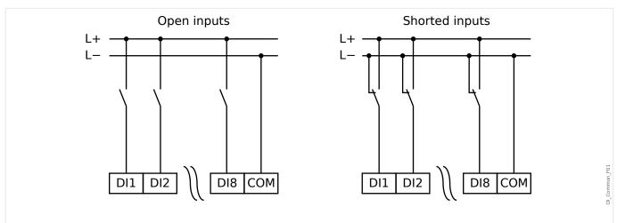
*Fig. 140:* Safe State of the Digital Inputs
