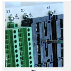
For either connection type, the first step is to remove the terminals from the device by opening the screws.
