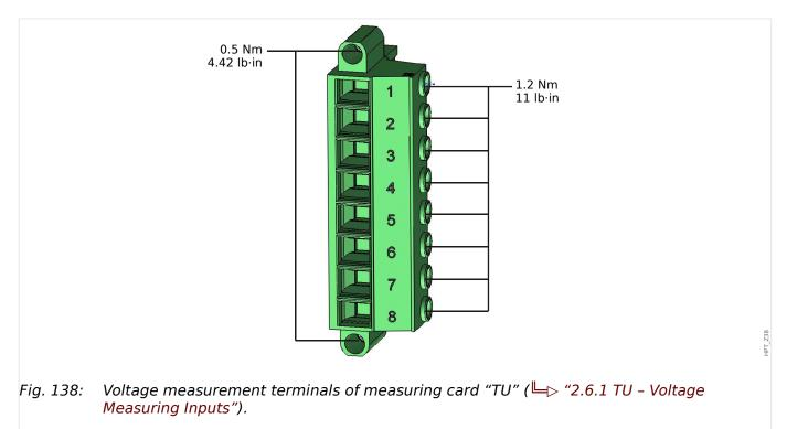
Voltage and Residual Voltage Measurement ("TU")
