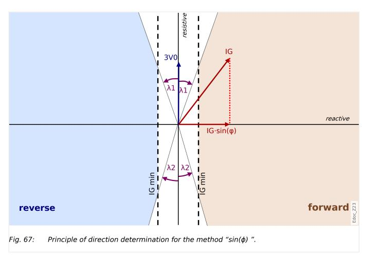
There are additional settings for the wattmetric direction detection methods:
