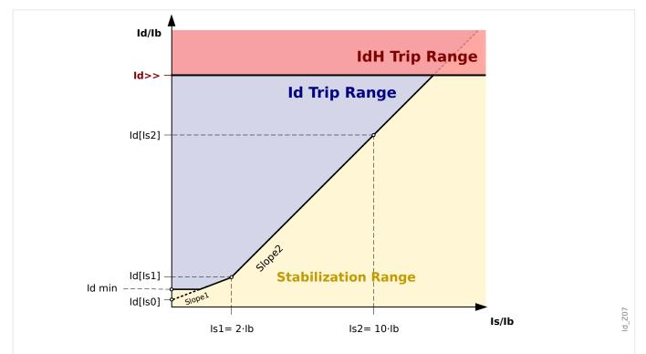
Fig. 48: Tripping curves of the »Id« (blue area) and of the »IdH« (red area) protection functions.
