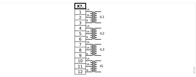
Fig. 15: TI - Terminal Marking
