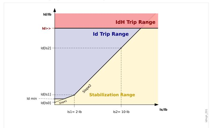
Fig. 51: Unrestrained High-set Differential Protection Step IdH.
