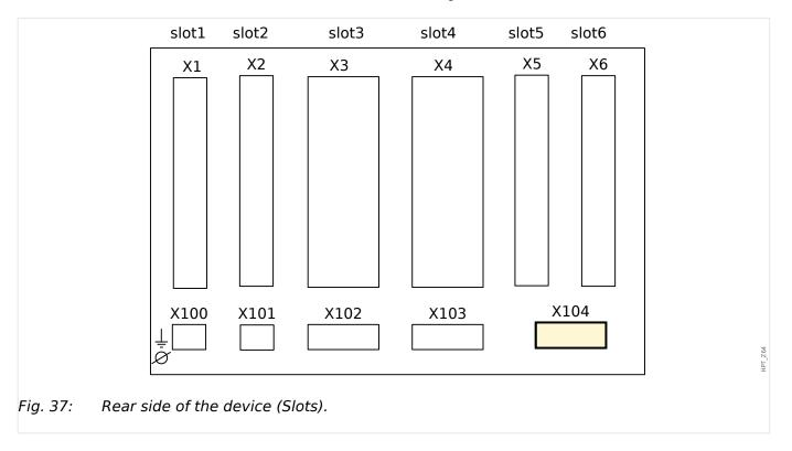
This slot comprises the IRIG-B00X and the Selfsupervision Contact.
