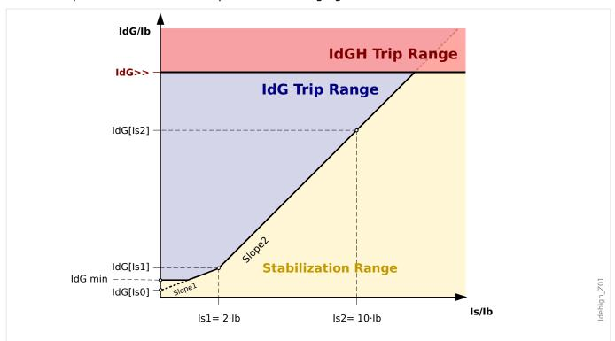
Fig. 53: Pickup value »IdG>>« of the earth differential current based on the rated current »Ib« of the related protection object.
