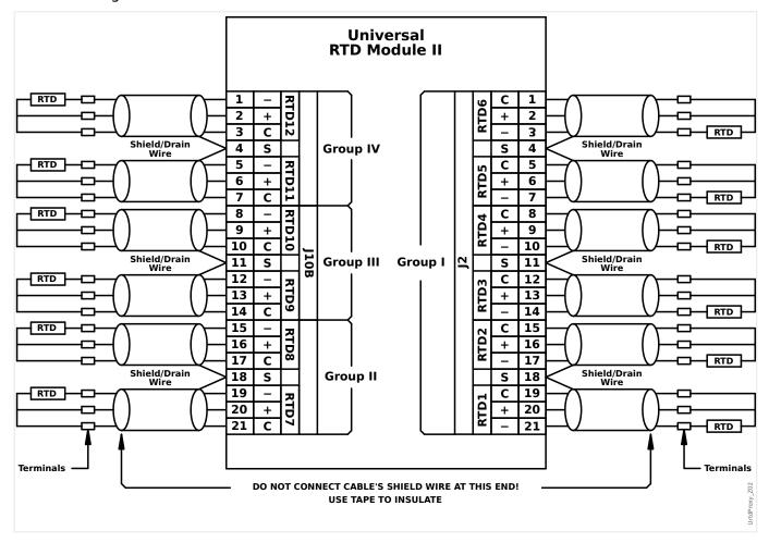
See the figure above for wiring of RTDs to the URTD inputs. Use three-conductor shielded cable. Note the connection rules in the figure. When making connections to a two-lead
