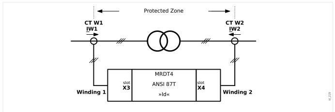
Fig. 47: ANSI 87T: Transformer Phase Differential Protection.
