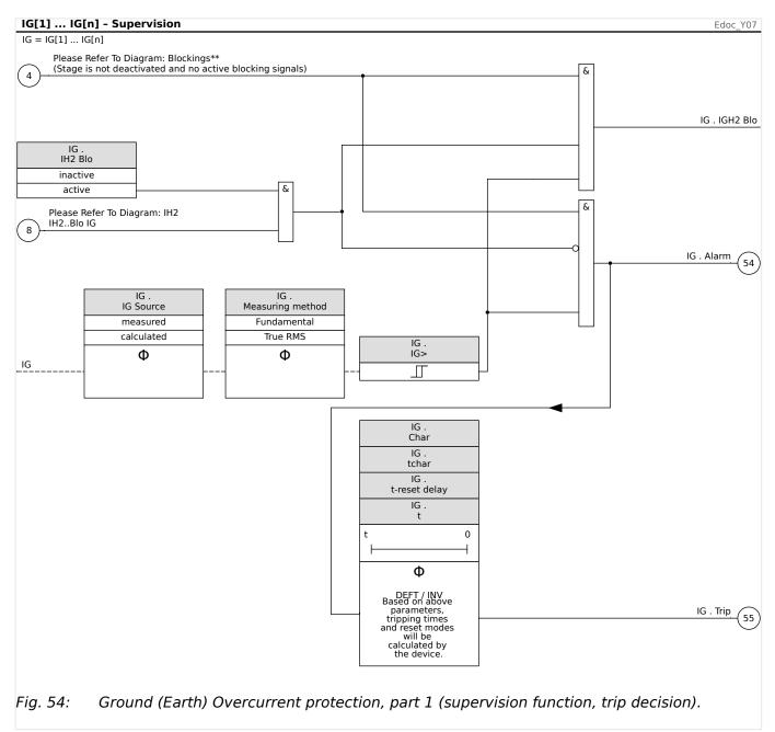
4.8.3 Commissioning: Ground Fault Protection - non-directional [50N/G, 51N/G]
