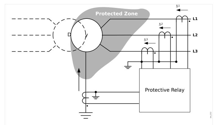
Fig. 52: Protection principle of Ground Current Differential Protection connected on wye-side winding of a transformer.
