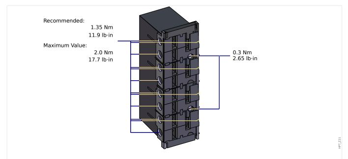
Fig. 81: Plug-in Connector with Integrated Short-Circuiter (Conventional Current Inputs)
