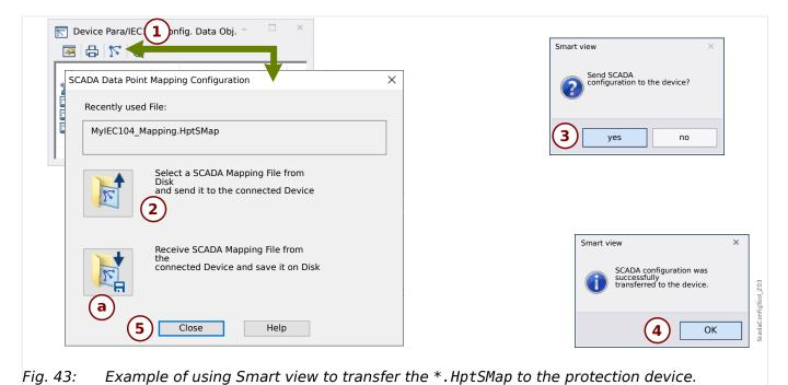
Button (2), »Select a SCADA Mapping File from Disk and send it to the connected Device. «, starts the upload of an edited mapping file. After clicking this button a file-select dialog opens.
