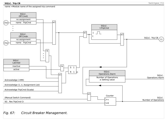
Note that in the diagram above, "SG[x]" represents "switchgear number x"; however, the exact designation is defined in the single-line file, see also  $\Longrightarrow$  "Single-Line Diagram".
