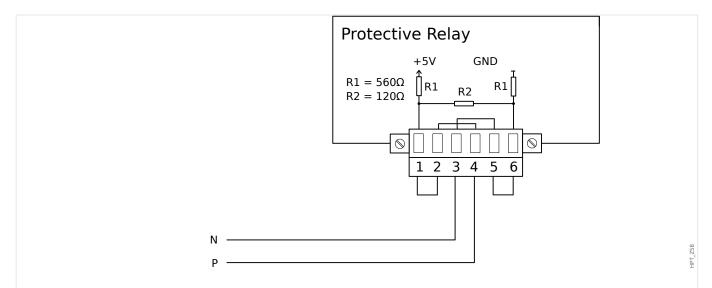
Wiring example, Device at the end of the bus. (Setting wire jumpers to activate the integrated Terminal Resistor.) Fig. 32:
