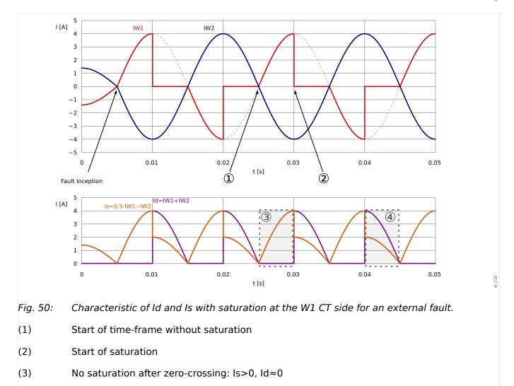
The stabilizing function evaluates for each zero-crossing event if an external fault is detected and the temporary restraining has to be triggered, or continued if already active. The restraining is removed if an internal fault is detected. This is the case when both Id and Is rise after two zero-crossing events in a row.
