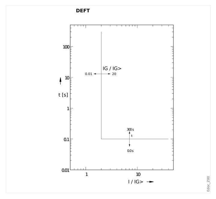
Trip delay for IG > IG > IG >, settable via [Protection Para / Set 1...4 / I-Prot / IG[x]] »t«.
