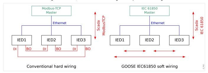
Commissioning steps for a conventional substation with modbus TCP environment:
