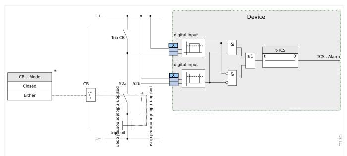
Fig. 60: Connection example: Trip circuit supervision with two CB auxiliary contacts »Aux ON« (52a) and »Aux OFF« (52b).
