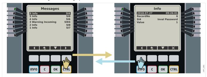
Fig. 80: Example display of the Self-Supervision messages.
