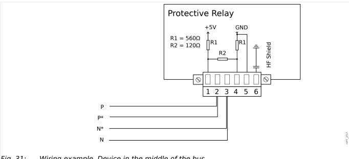
Fig. 31: Wiring example, Device in the middle of the bus
