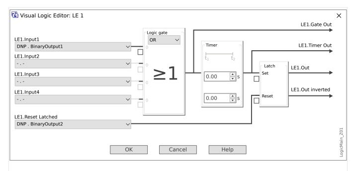
Fig. 42: Setting example from Smart view, to make a steady state signal from a DNP output signal.
