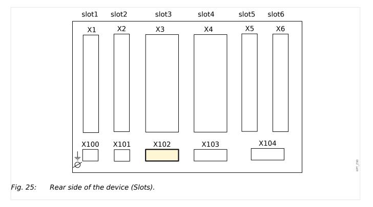
The Protection Communication interface is available in slot **X102**.
