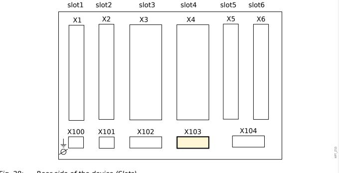
Fig. 28: Rear side of the device (Slots)
