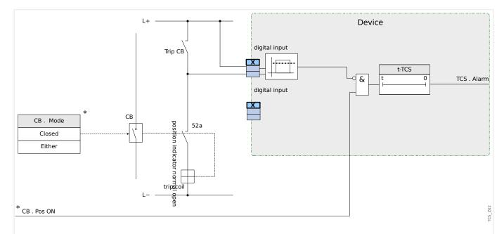
Connection example: Trip circuit supervision with only one CB auxiliary contact »Aux Fig. 61: ON« (52a).
