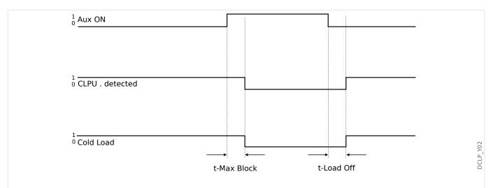
Fig. 57: Example Mode: Breaker Position.
