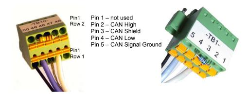
Figure 4-8. CAN Communication Ports
