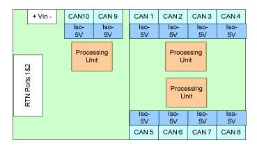
Figure 2-4. GW CAN Port Internal Configuration
