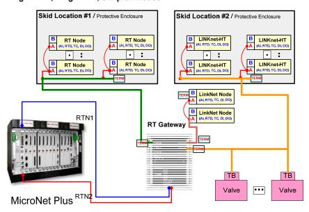
Figure 2-1. RTN Distributed I/O Single CPU, Single GW Simplex Nodes
