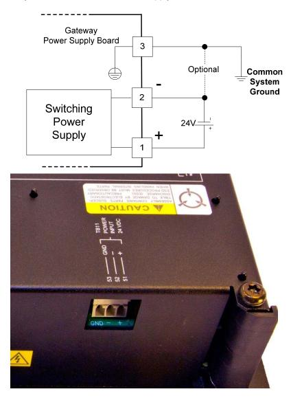
Figure 4-2. Input Power Wiring Diagram and Example
