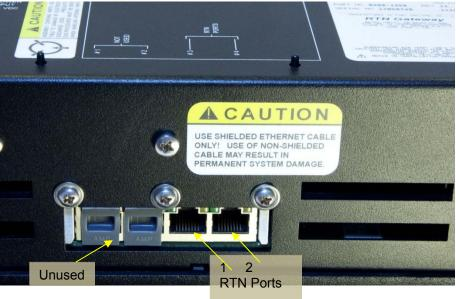
Figure 4-6. 10/100 BaseT Ethernet Ports (RJ45)
