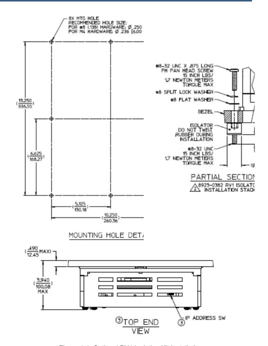
Figure 4-1. Optional RV1 Isolation Kit Installation
