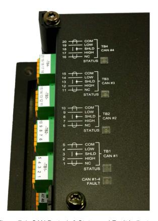
Figure 7-1. CAN Ports 1–8 Status and Fault Indicators
