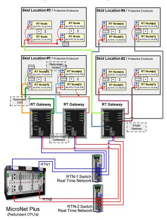
Figure 2-3. RTN Distributed I/O Dual CPU's, Multiple GW's Simplex Nodes
