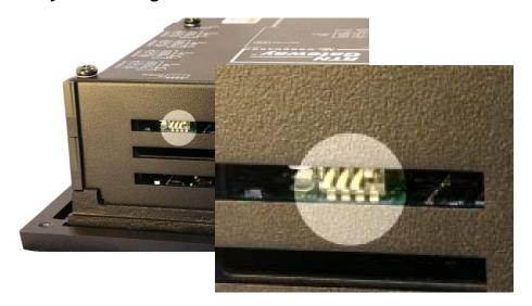
Figure 4-4. Module Configuration Switch
