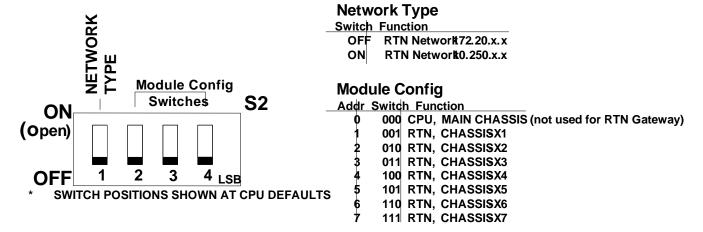
Figure 4-5. Module Configuration Switch Setting
