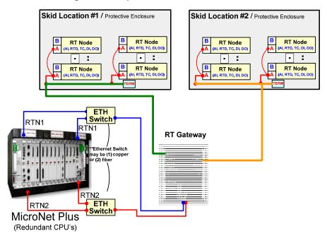
Figure 2-2. RTN Distributed I/O Dual CPUs, Single GW Simplex Nodes
