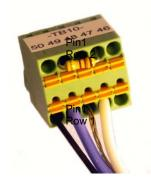
Termination Resistor (120 $\Omega$ ) Pin2->Pin4
