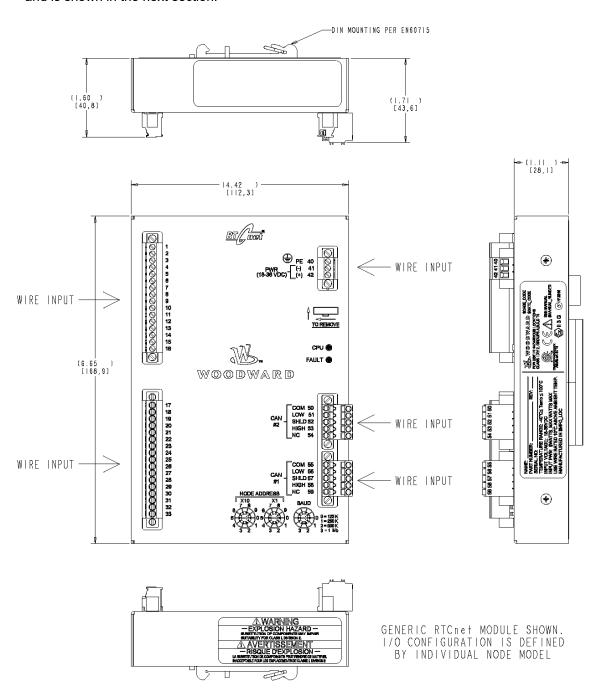
Figure 3-1. RTCnet and LINKnet HT Node Outline Drawing
