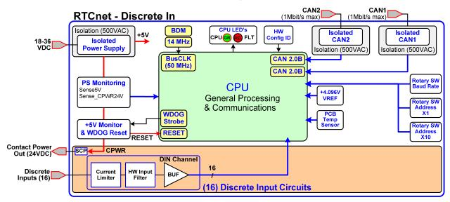
Figure 7-2. RTCnet DI Block Diagram
