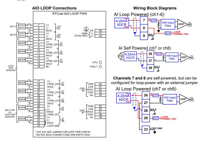
Figure 6-3. RTCnet AIO Loop Connections and Wiring Block Diagrams
