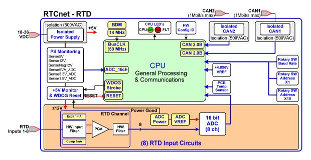
Figure 4-2. RTCnet RTD Block Diagram
