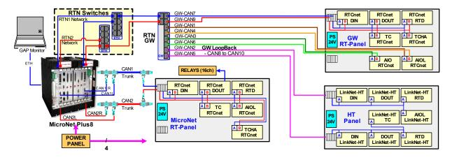
Figure 2-2. Redundant CPU's and Multiple Node Locations
