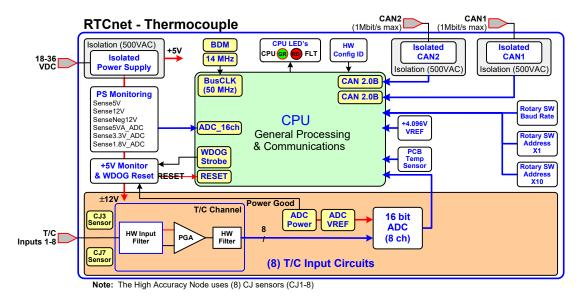
Figure 5-2. RTCnet Thermocouple Block Diagram
