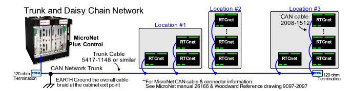
Figure 2-1. Network Wiring— Daisy Chain or Trunk and Daisy Chain
