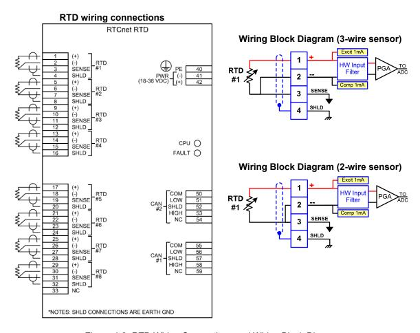
Figure 4-3. RTD Wiring Connections and Wiring Block Diagram
