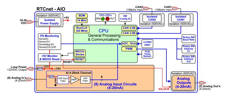
Figure 6-2. RTCnet AIO Block Diagram
