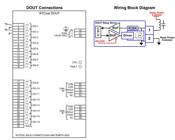
Figure 8-3. DOUT Connections and Wiring Block Diagram
