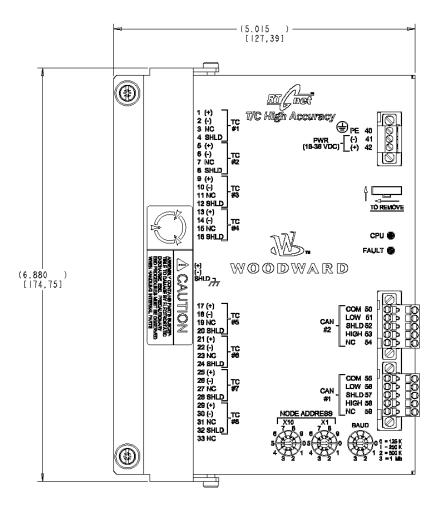
Figure 3-2. T/C High Accuracy Node Outline Drawing
