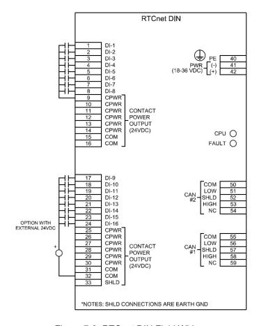
Figure 7-3. RTCnet DIN Field Wiring
