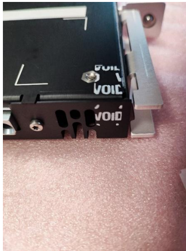
Figure A-4. Tampered Seal on Chassis
