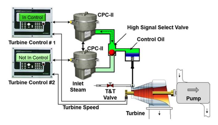
Figure 1. Basic Redundant CPC-II Skid Application
