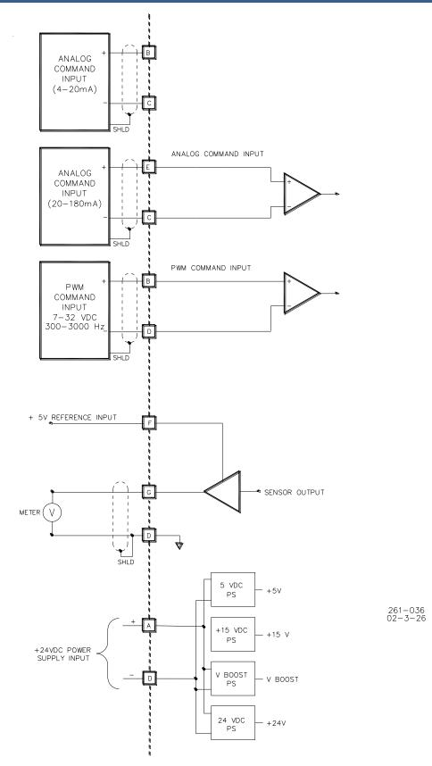
Figure 3-2. Representative I/O Schematic
