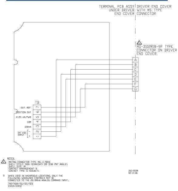
Figure 3-1. Control Wiring Diagram
