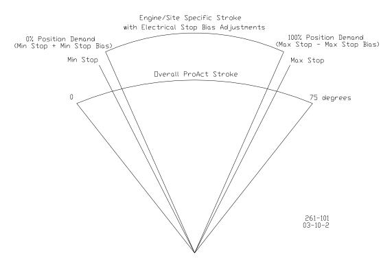
Figure 7-1. Electrical Stop Adjustments Relative to the Mechanical Min and Max Stops
