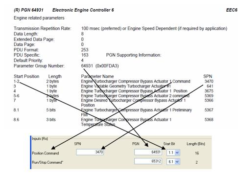
Figure B-1. Position Command Mapping
