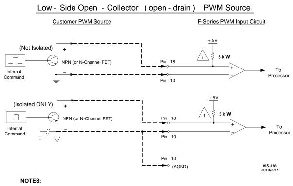
This resistor is present in all FSeries versions. It must be taken into consideration when selecting an external pullup or pull-down resistor to ensure that the PWM signal passes through the detection threshold
