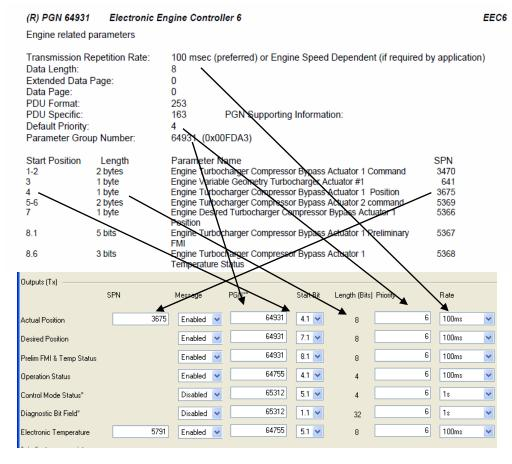
Figure B-2. Actual Position Mapping
