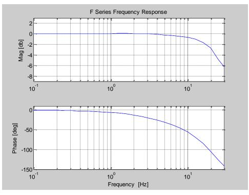
Figure B-3. Typical Bode Plot of F-Series Actuator Response
