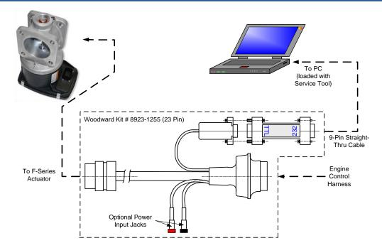
Figure 5-2. Communication- Harness Connections
