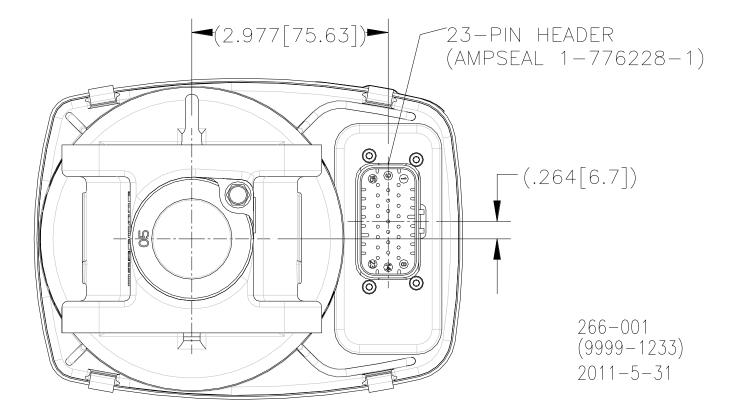
Figure 1-4. 23-Pin Electrical Connector
