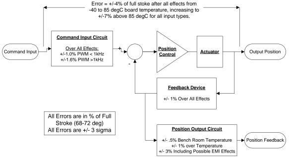
Figure 4-1. Position Tolerances
