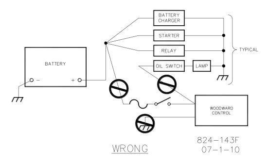
Figure 3-2b. Incorrect Power Supply Wiring
