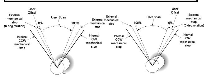
Figure 5-19a. Stops Setup for CW Operation
