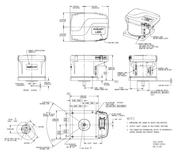
Figure 1-2. F-Series Modular Actuator Outline Drawing
