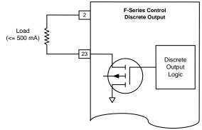
Figure 3-11. Status Discrete Output
