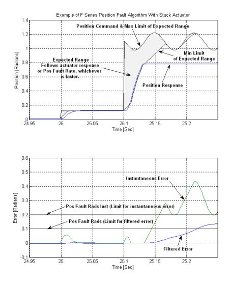
Figure 4-5. Position and Error Example with Stuck Actuator
