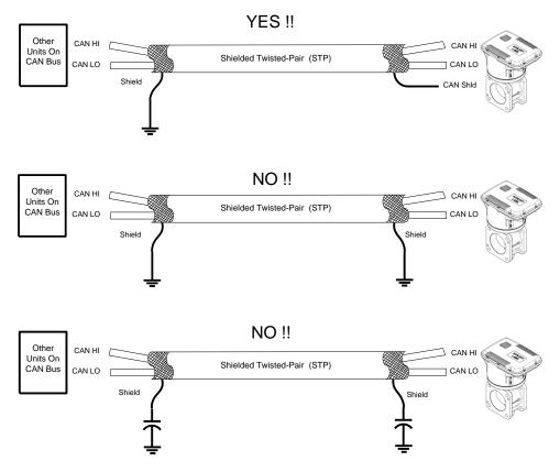
Figure 3-10. CAN Shielded Wiring
