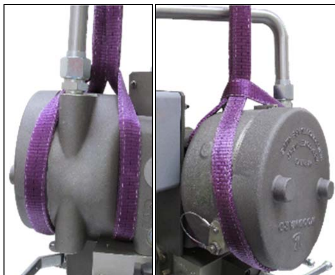
Figure 3-7. Lifting strap properly installed (CPC-II unit on the CPC-DX hydraulic manifold).
