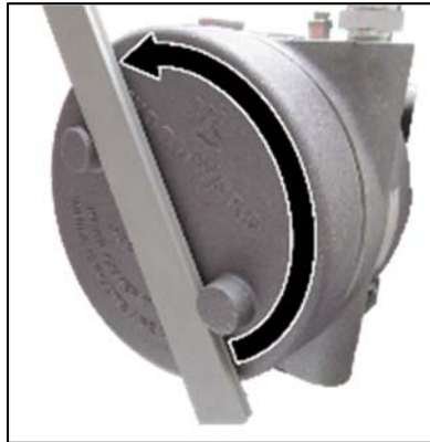
Figure 4-2. Loosening CPC-II cover with bar.
