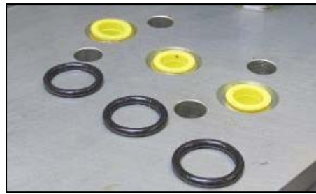
Figure 3-13. CPC-DX manifold with secured hydraulic passages after CPC-II unit removal (shown yellow plastic plugs not provided with the CPC-II unit)
