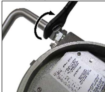
Figure 4-10. CPC-II conduit nut unscrewing.
