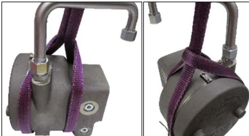
Figure 3-6. Lifting strap properly installed.
