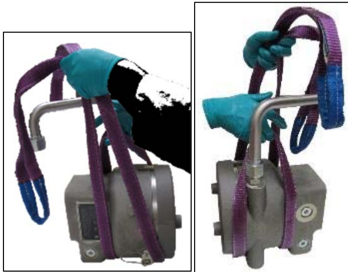
Figure 3-5. Lifting strap installation.
