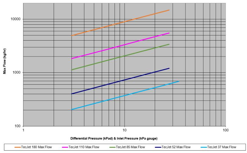
Figure 4-1. Maximum Specialty Gas Flow Capacity of TecJet 180, 110, 85, 52 and 37 (Specialty Gas, SG=1, Sea Level)
