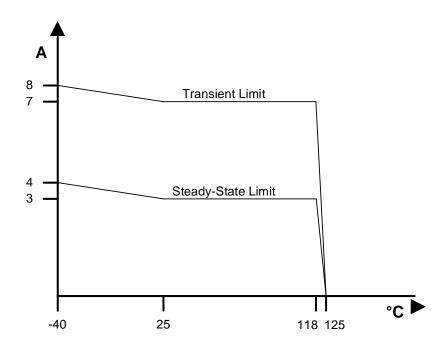
Figure 3-1. Current Limiting Based on Temperature
