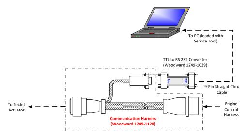
Figure 5-1. Communication- Harness Connections
