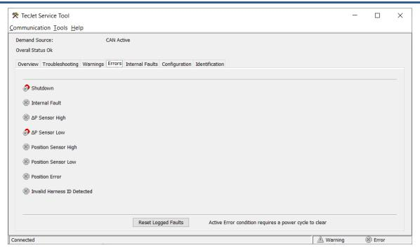
Figure 5-5b. Errors Screen after Power Cycle
