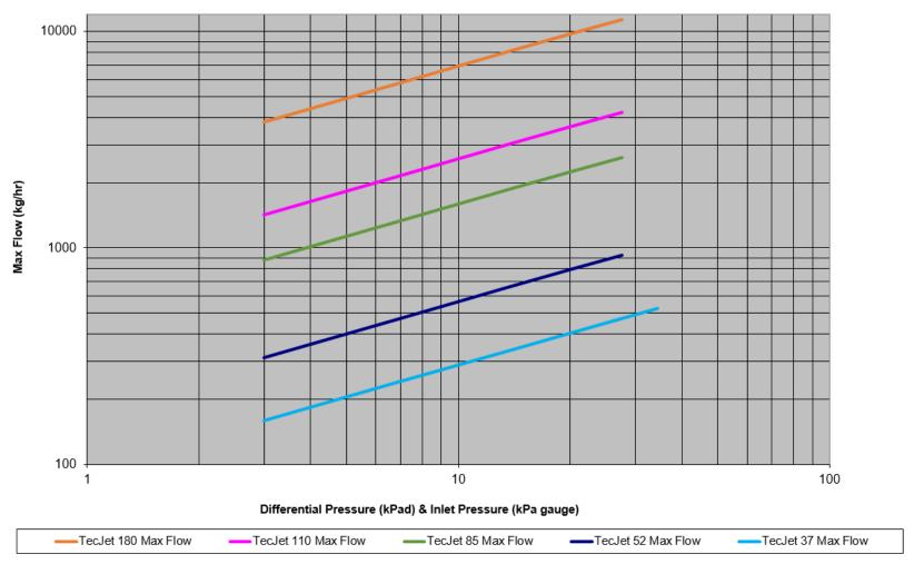
Figure 4-3. Maximum Natural Gas Flow Capacity of TecJet 180, 110, 85, 52 and 37 (Natural Gas, SG=0.6, Sea Level)
