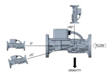
Figure 2-1c. Allowable Bore Orientations
