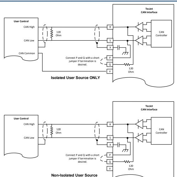
Figure 2-7. TecJet 52 CAN Wiring for Isolated/Non-Isolated Systems
