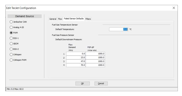
Figure 5-10. Edit TecJet Configuration - Failed Sensor Defaults
