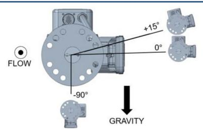
Figure 2-1b. Allowable Actuator Orientations
