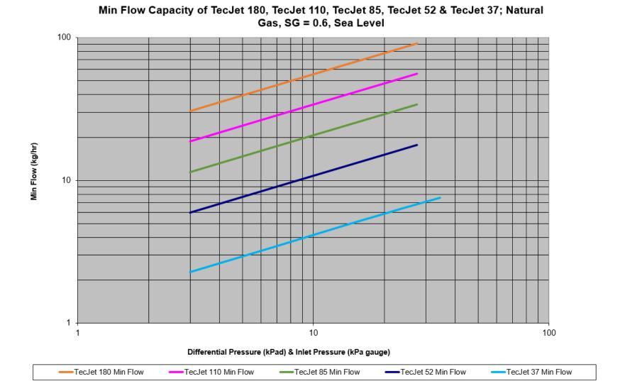
Figure 4-4. Minimum Natural Gas Flow Capacity of TecJet 180, 110, 85, 52 and 37 (Natural Gas, SG=0.6, Sea Level)
