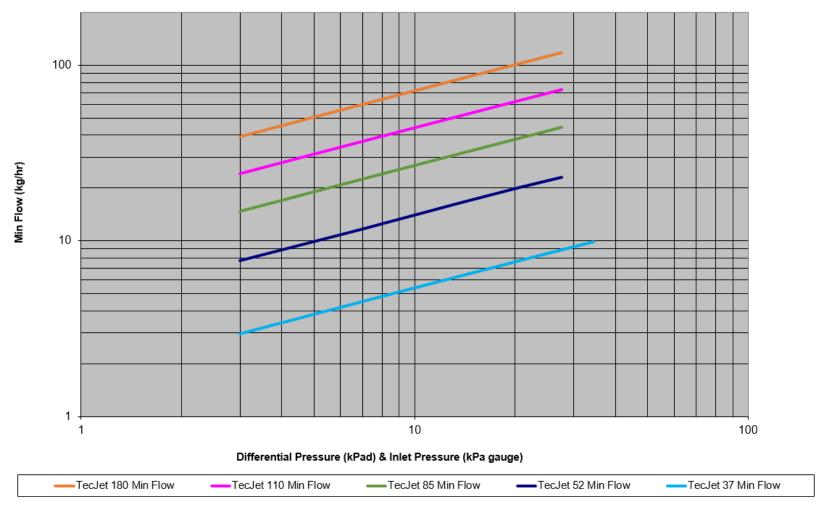
Figure 4-2. Minimum Specialty Gas Flow Capacity of TecJet 180, 110, 85, 52 and 37 (Specialty Gas, SG=1, Sea Level)
