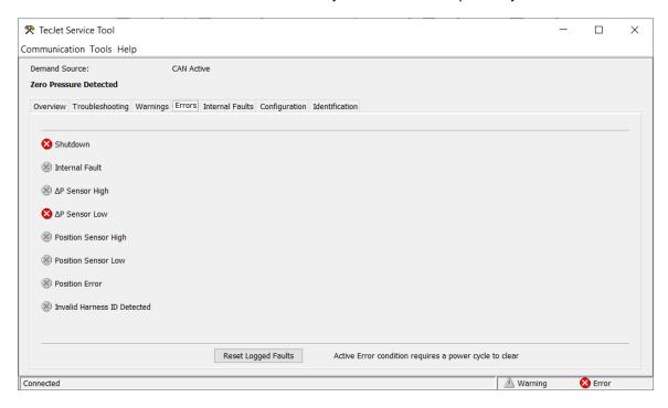
Figure 5-5a. Errors Screen before Power Cycle
