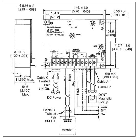
Dimensions are in mm. Dimensions in brackets [] are in inches.
