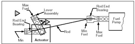
Figure 5. Rotary Actuator to Linear Fuel Pump Linkage
