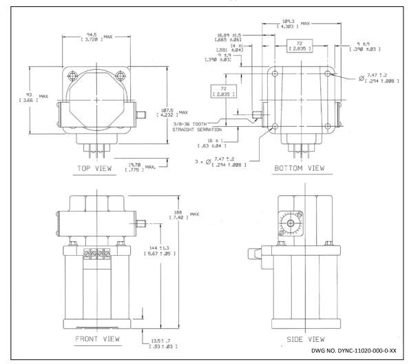
Dimensions are in millimeters. Dimensions in brackets [] are inches.
