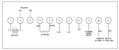
Figure 7. Wiring Diagram for CE Controllers
