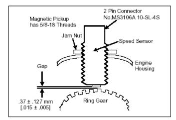
Figure 3. Installation of Magnetic Pickup
