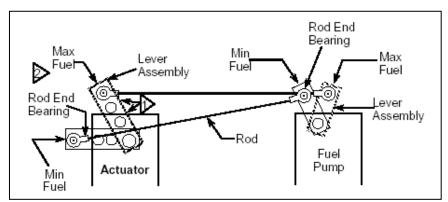
Figure 4. Rotary Actuator to Rotary Fuel Pump Linkage
