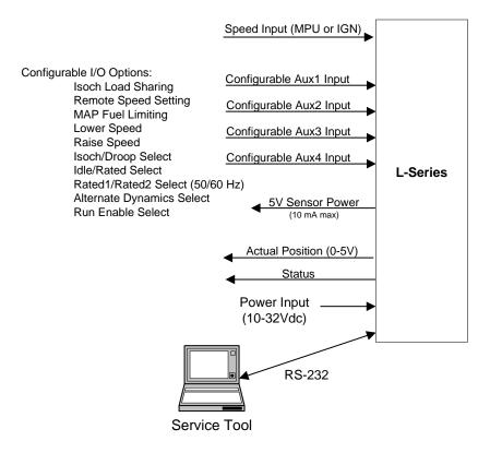
Figure 4-1 Overview of L-Series Inputs/Outputs
