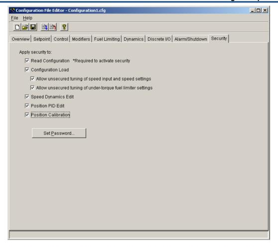
Figure 6-10. Configuration Editor—Security Tab
