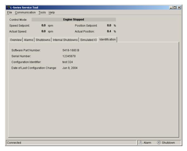
Figure 5-8. Service Tool—Identification Tab
