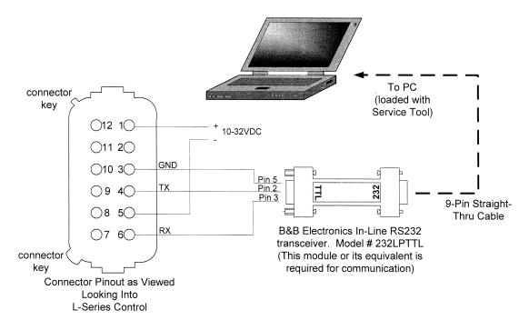
Figure 5-2b. Programming Harness Wiring
