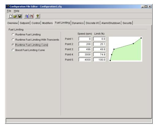
Figure 6-6a. Configuration Editor—Fuel Limiting Tab (5418-1680 software version)
