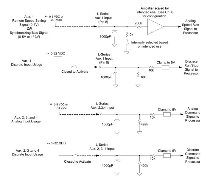
\*\* Reference all analog or discrete inputs to L-Series signal ground (Pin 3)
