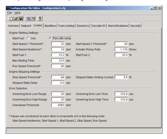
Figure 6-4. Configuration Editor—CONTROL TAB
