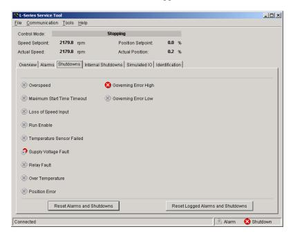
Figure 5-5. Service Tool—Shutdowns Tab
