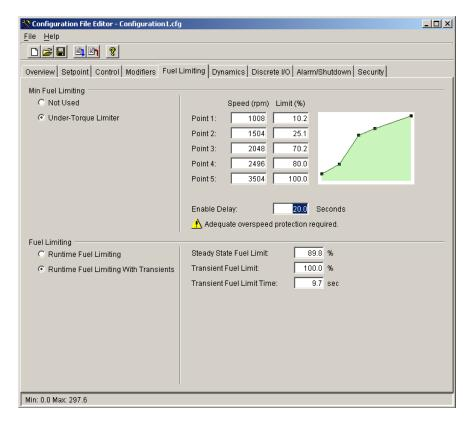
Figure 6-6c. Configuration Editor—Fuel Limiting Tab (5418-2193 software only)
