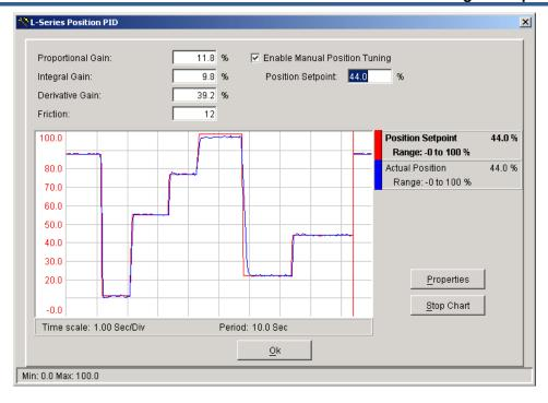
Figure 7-3. Service Tool—PID Tuning Window
