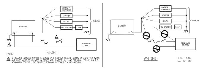
Figure 3-2. Correct and Incorrect Wiring to Power Supply
