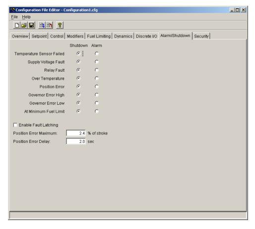
Figure 6-9. Configuration Editor—Alarm/Shutdown Tab
