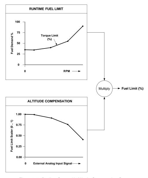
Figure 4-10. Runtime Curve with Altitude Compensation Curve
