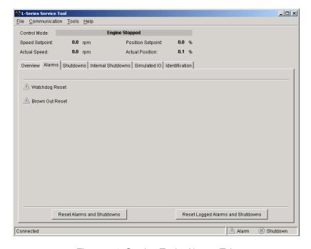
Figure 5-4. Service Tool—Alarms Tab
