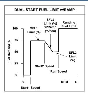
Figure 4-7. Dual Start Fuel Limiters
