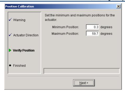
Figure 7-8. Service Tool—Manual Position Calibration Settings
