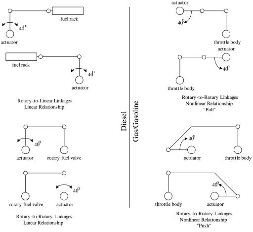
Figure 2-1. Linkage Design Examples
