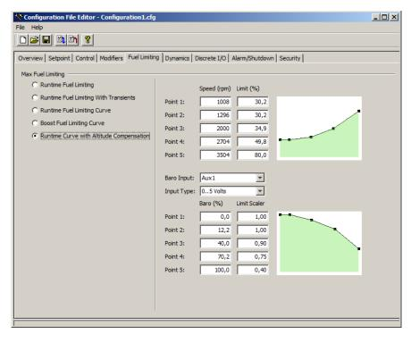
Figure 6-6b. Configuration Editor—Fuel Limiting Tab (5418-6634 software only)
