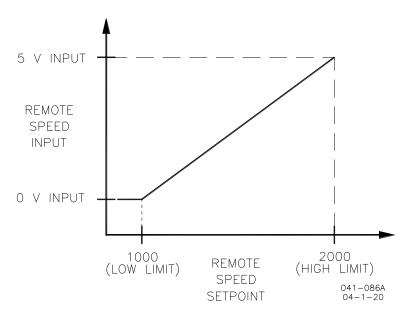
Figure 4-4 Remote Speed Setpoint
