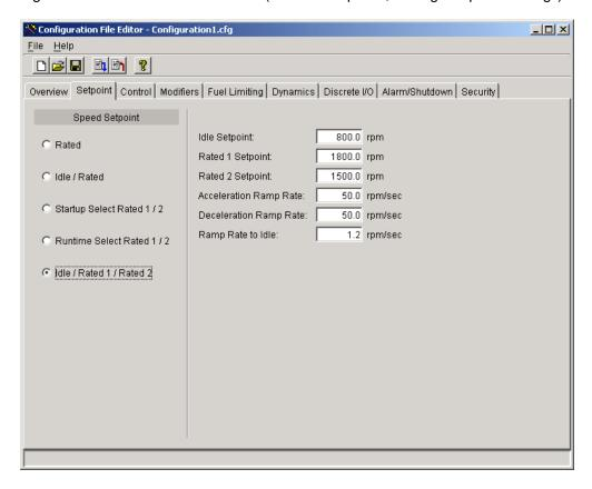
Figure 6-3. Configuration Editor—SETPOINT TAB
