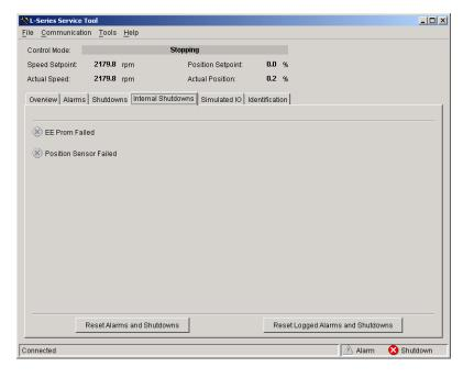
Figure 5-6. Service Tool-Internal Shutdowns Tab
