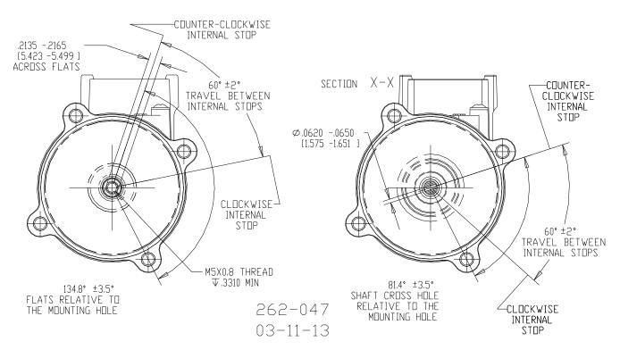
Figure 2-4a. L-Series Shaft Types
