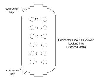
Figure 3-1b. L-Series Speed Control Connector Pin Arrangement
