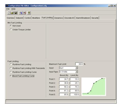
Figure 6-6d. Configuration Editor—Fuel Limiting Tab (5418-2193 software only)
