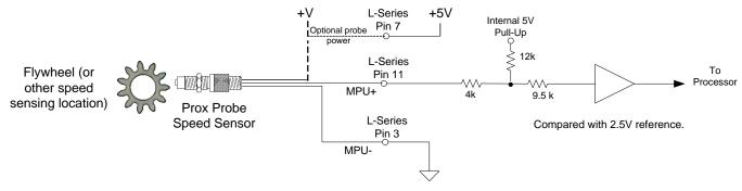
Figure 3-4. Proximity Probe Speed Sensing Input (5418-1680 rev D or newer only)
