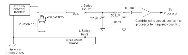
Figure 3-5. Ignition Speed Sensing Input
