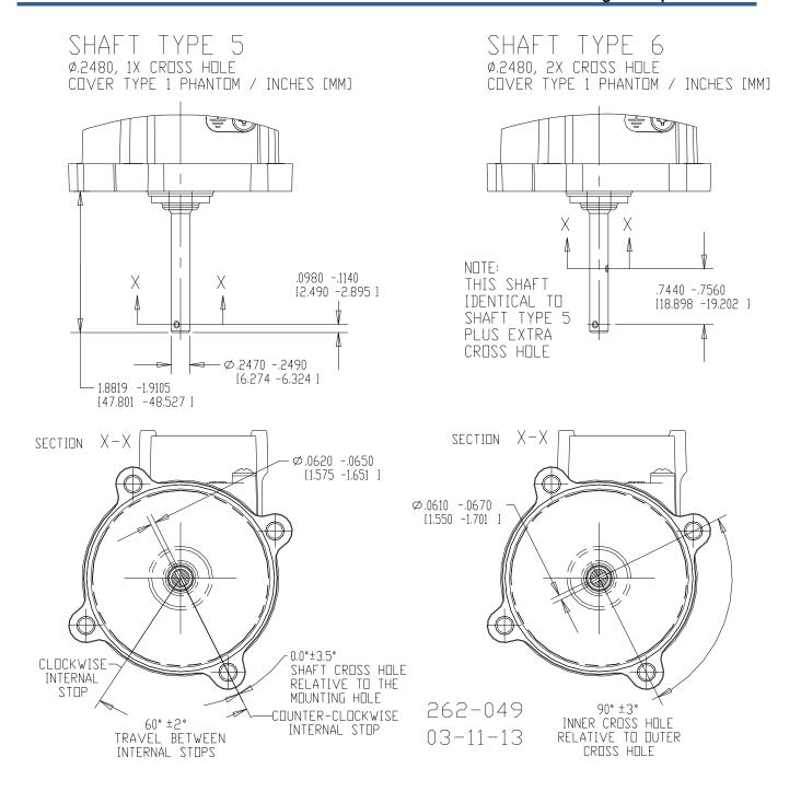
Figure 2-4c. L-Series Shaft Types
