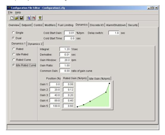
Figure 6-7. Configuration Editor—Dynamics Tab
