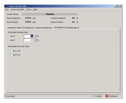
Figure 5-7. Service Tool—Simulated I/O Tab
