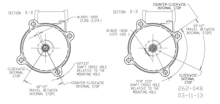
Figure 2-4b. L-Series Shaft Types
