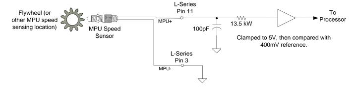
Figure 3-3. MPU Speed Sensing Input
