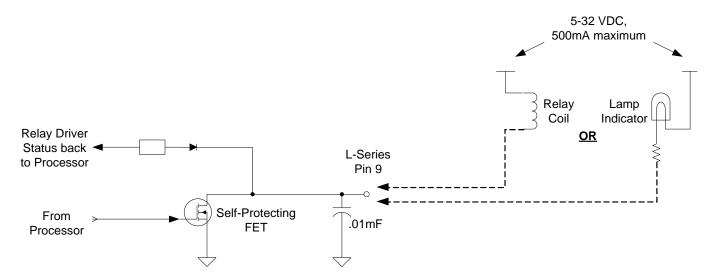
Figure 3-7. Relay Driver Output
