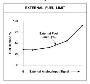
Figure 4-8. Boost (External) Fuel Limit Curve
