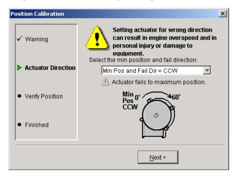
Figure 7-7. Service Tool—Manual Position Calibration
