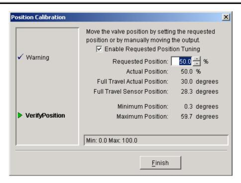
Figure 7-6. Service Tool—Verify Position Calibration
