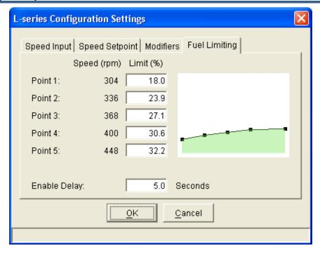
Figure 7-2c. Configuration Settings Window (5418-2193 software only)
