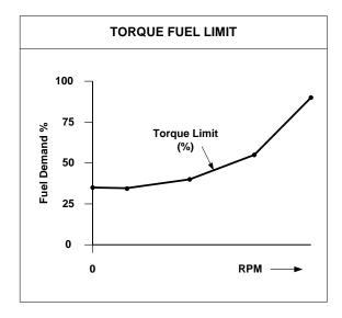
Figure 4-9. Runtime Fuel Limit Curve
