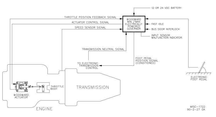
Figure 1-1. Bus Control Block Diagram
