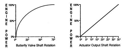
Figure 3-2. Effect of Butterfly Linkage
