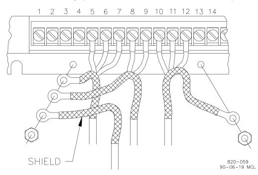
Figure 3-4. Proper Preparation of Shielded Wires
