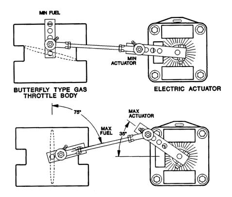
Figure 3-3. Linkage for Non-linear Installations
