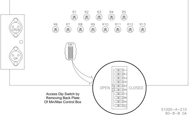
Figure 3-1. DIP Switch Location on Other Side of Printed Circuit Board
