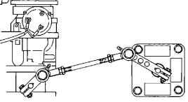
Figure 2-3. Carburetor Compensating Linkage at Minimum Fuel
