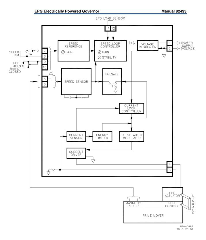
Figure 4-1. EPG Block Schematic Diagram
