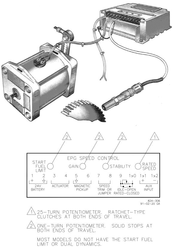
Figure 1-1. Basic Electrically Powered Governor System
