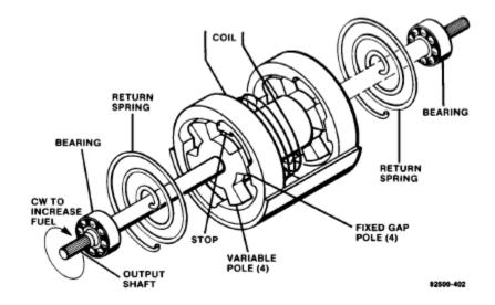
Figure 4-2. Actuator Schematic
