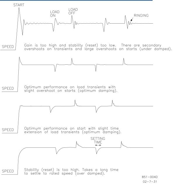
Figure 2-9. Starting and Transient Response Curves
