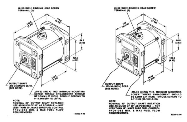
Figure 1-3. Outline Drawing for EPG 1712/1724 and 512/524 Actuators (Do not use for construction.)
