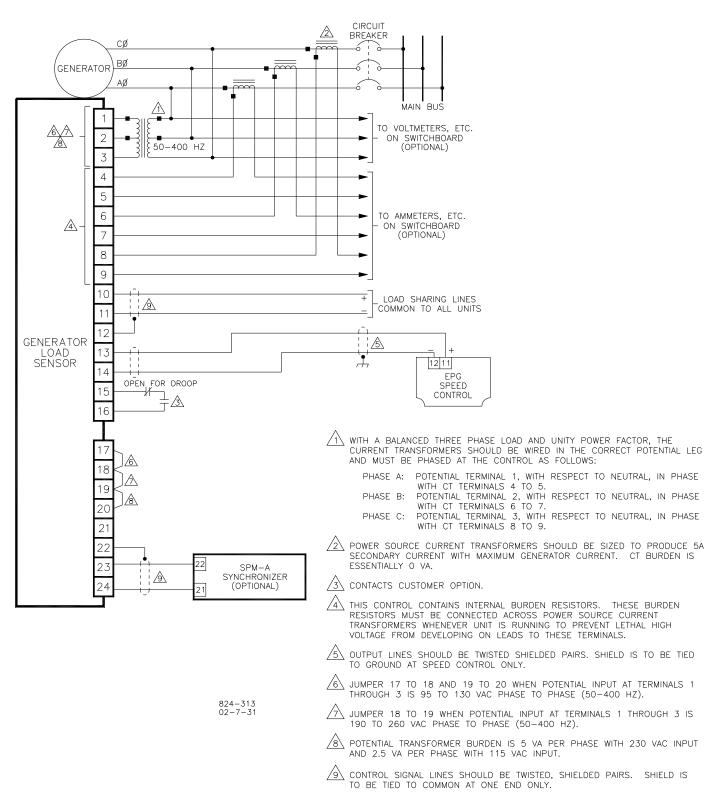
Figure 2-8. Additional Wiring to Install the EPG Load Sensor (for paralleled generator applications)
