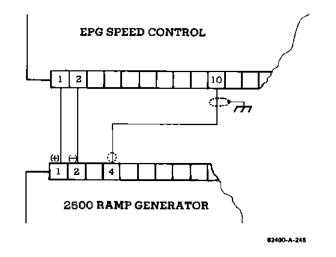
Figure 2-7. Typical Wiring to 2500 Ramp Generator
